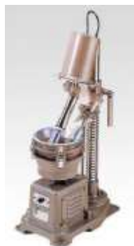
Fig. S1 An automatic agate mortar utilized for producing powder composite through mechanical mixing.
