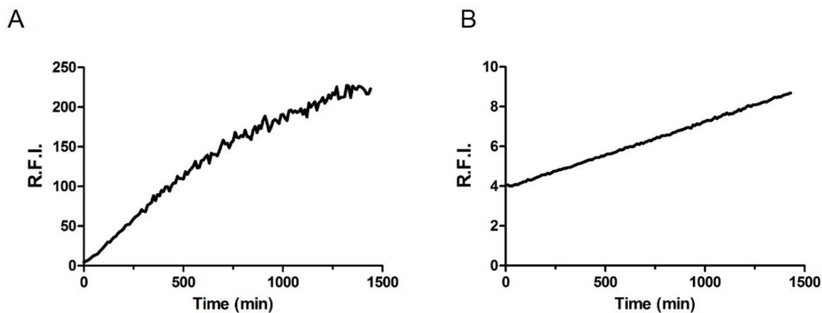
**Fig. S1.** Catalyzed fluorescence “switch-on” of the caged fluorophore **5** (50  $\mu\text{M}$ ) with the Pd-peptide **1** (5  $\mu\text{M}$ ) in (A) PBS and (B) PC-3 cell lysate for 24 h at 37  $^{\circ}\text{C}$ . Relative increase in fluorescence (RFI) was measured at  $\lambda_{\text{Ex/Em}}$  495/520 nm and normalised to a control solution of **5** in the absence of the Pd-peptide catalyst.
