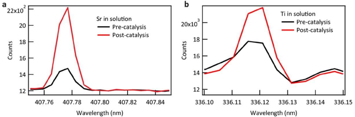
**Fig. S 2:** ICP spectra of a) Sr metal in solution and b) Ti metal in solution pre- and post-catalysis
