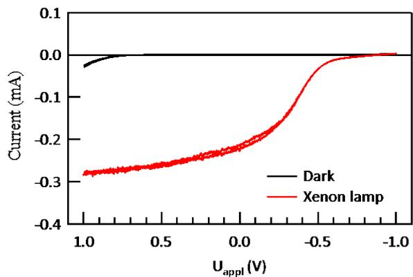
**Fig. S 1:** Cyclic voltammogram of n-SrTiO<sub>3</sub> in the dark and under irradiation by a 150 W Xenon lamp. Similar to the current-voltage curve under laser irradiation (Figure 1a of the main text), a diode-like behavior was observed under Xenon lamp irradiation.
