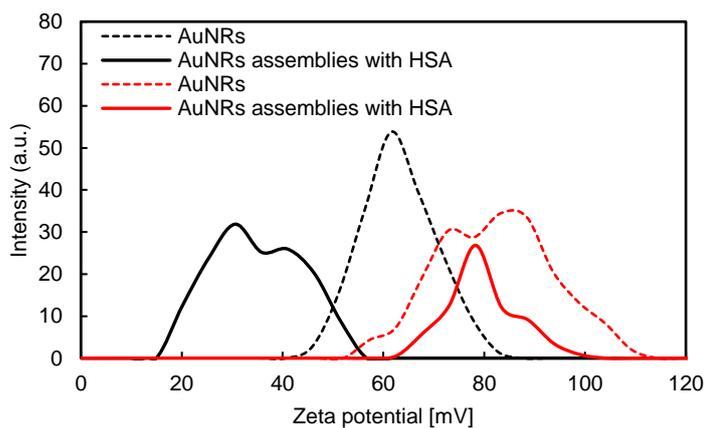
**Fig. S8** Zeta potentials of AuNRs and AuNRs assemblies with HSA in 20 % (black) and 0 % (red) MeCNaq. The concentration of HSA and AuNRs is set to 10  $\mu\text{M}$  and 0.60 nM, respectively.
