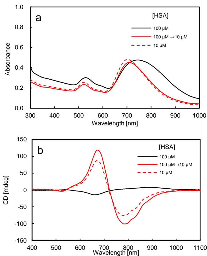
**Fig. S6** (a) UV-vis-NIR spectra and (b) CD spectra of AuNRs assemblies with 10  $\mu\text{M}$  and 100  $\mu\text{M}$  HSA and reconstructed AuNRs assemblies by adjusting the HSA concentration from 100  $\mu\text{M}$  to 10  $\mu\text{M}$ . Cell length: 1mm. The concentration of AuNRs is set to 0.60 nM.
