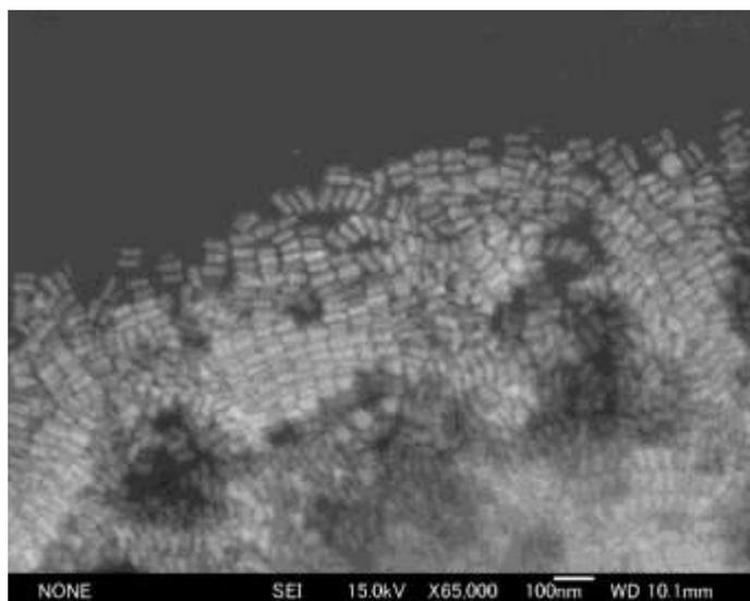
**Fig. S1** FE-SEM image of as-prepared AuNRs.
