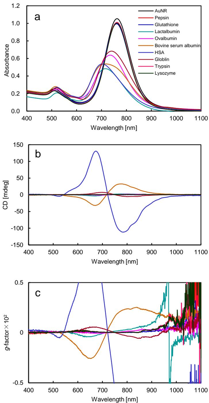
**Fig. S11** (a) UV-vis-NIR spectra, (b) CD spectra and (c)  $g$ -factor of AuNRs assemblies with 10  $\mu$ M various proteins in 20 % MeCNaq. Cell length: 1mm. The concentration of Proteins and AuNRs is set to 10  $\mu$ M and 0.60 nM, respectively.
