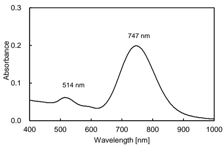
**Fig. S2** UV-vis-NIR spectra of as-prepared AuNRs in water.
