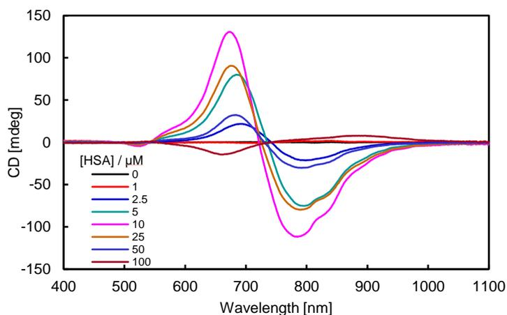
**Fig. S4** CD spectra of AuNRs assemblies with HSA in 20 % MeCNaq. Cell length: 1mm. The concentration of HSA and AuNRs is set to 0–100  $\mu\text{M}$  and 0.60 nM, respectively.
