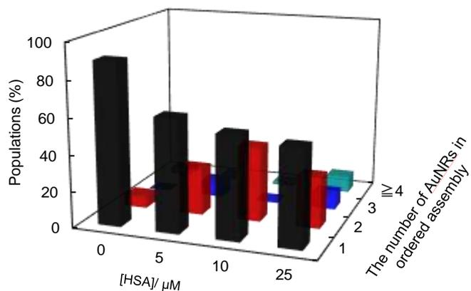
**Fig. S5** Yields of AuNRs assemblies with HSA in 20% MeCNaq, determined by FE-SEM. The concentration of HSA and AuNRs is set to 0-25  $\mu\text{M}$  and 0.60 nM, respectively.
