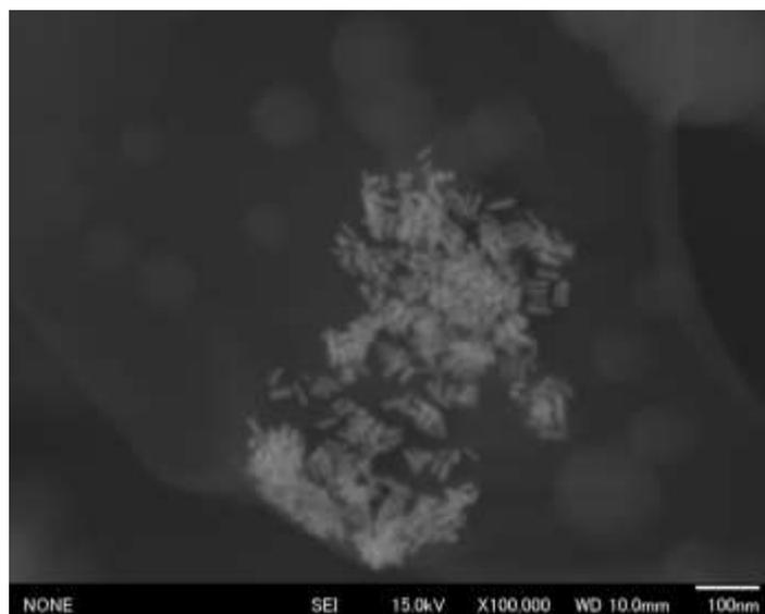
**Fig. S3** FE-SEM image of AuNRs assembly with HSA in the 20 % MeCNaq. The concentration of HSA and AuNRs is set to 100  $\mu\text{M}$  and 0.60 nM, respectively. The FE-SEM sample was prepared by freeze-drying process.
