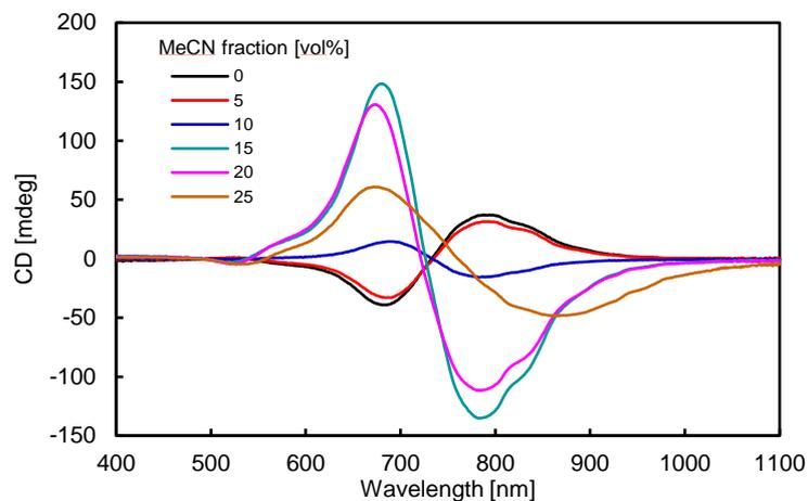
**Fig. S7** CD spectra of AuNRs assemblies with HSA in the MeCN/water mixture. Cell length: 1mm. The concentration of HSA and AuNRs is set to 10  $\mu\text{M}$  and 0.60 nM, respectively.
