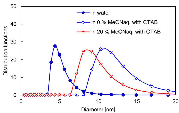
**Fig. S10** DLS measurements of 0.1 mM HSA in the absence and presence (40 mM) of CTAB in water and 20 % MeCNaq.
