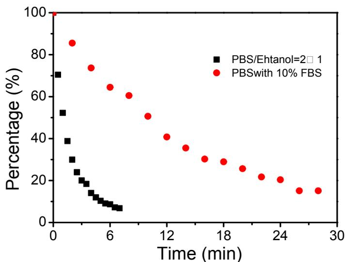
**Fig. S5.** Photo-stability of **pH-PTT** (25  $\mu\text{M}$ ) in PBS/ethanol and **BSA-pH-PTT** in PBS irradiated by 808 nm laser (2  $\text{W}/\text{cm}^2$ ) for different time. a) The percentage of absorbance decrease at 808 nm with irradiation time, which show enhanced photo-stability of **pH-PTT** in FBS medium.
