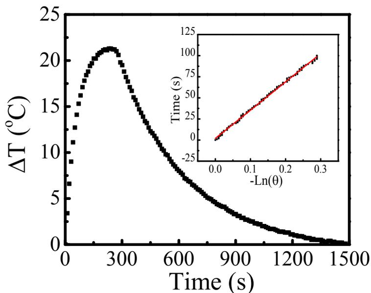
**Fig. S4.** The photo-thermal effect upon the irradiation of **BSA-pH-PTT** ( $20 \mu\text{M}$ ) with NIR laser, in which the irradiation lasted for 5 min, and then the laser was shut off. Inset: time constant for the heat transfer from the system is determined to be  $hA = 334$  s by applying the linear time data from the cooling period versus negative natural logarithm of driving force temperature, which is obtained from the cooling stage of panel.
