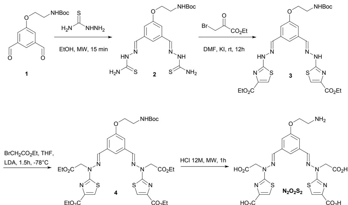
Figure 2. Synthesis of  $N_2S_2O_2$  ligand.
