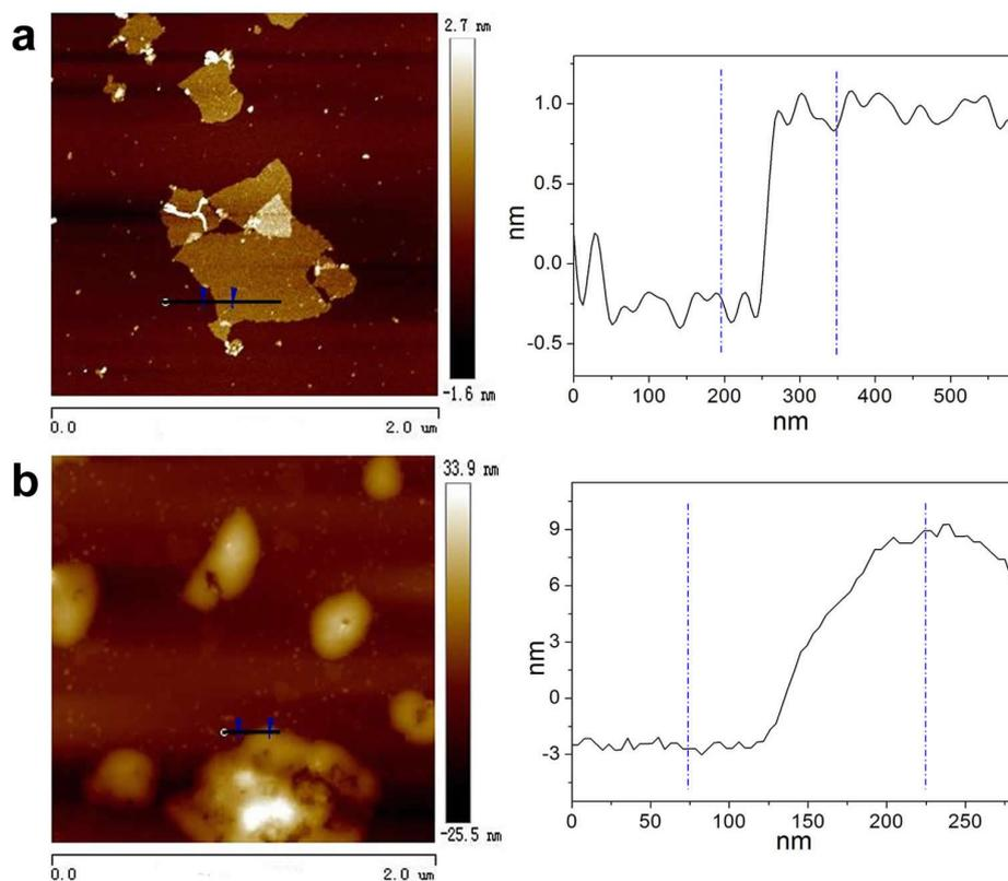
**Fig. S3** Tapping mode AFM images and corresponding height profiles of GO (a) and poly(NIPAm-*co*-ViEtImBr)-rGO (b).
