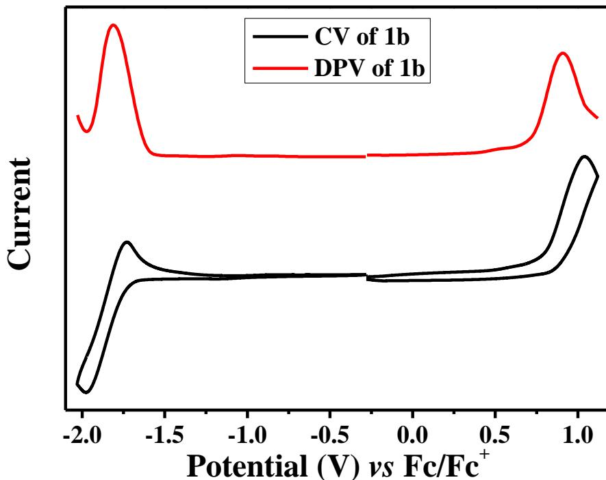
**Figure S4** Cyclic voltammograms (black) and differential pulse voltammograms (red) of **1b** in dry dichloromethane with 0.1 M  $\text{Bu}_4\text{NPF}_6$  as supporting electrolyte, Ag/AgCl as reference electrode, Au disk as working electrode, Pt wire as counter electrode, and scan rates at 50 mV/s.
