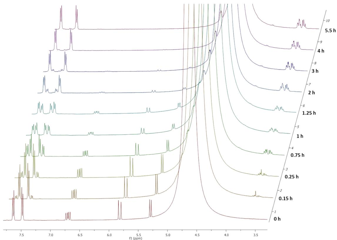
In aqueous medium ( $\text{D}_2\text{O}$ ) 40 mM substrate **1g**, 0.1 M citrate (pH5), 160 mM KBr, 170 mM  $\text{H}_2\text{O}_2$ , 100 nM CiVCPO was mixed at room temperature. The  $^1\text{H}$  NMR spectra were measured in 7 hours followed by time.
