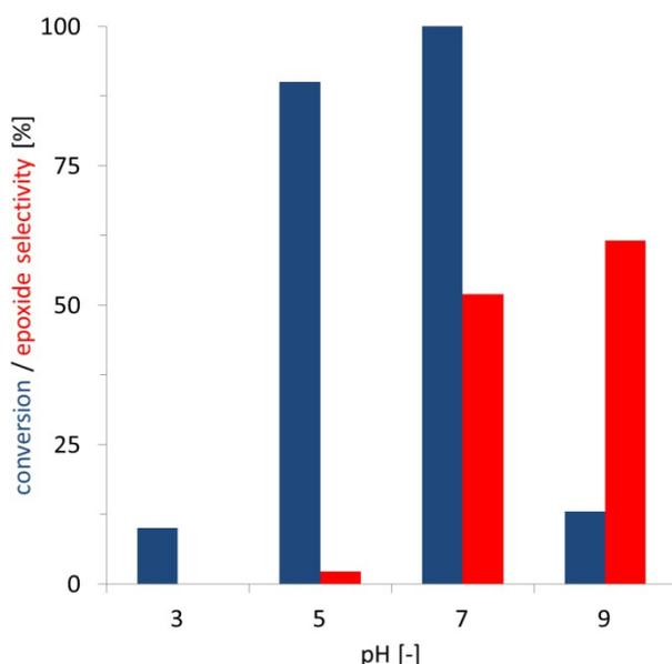
**Figure S1.** Activity and selectivity of the chemoenzymatic halohydroxylation of styrene at different pH values. General conditions:  $c(\text{CVCPO}) = 100 \text{ nM}$ ,  $c(\text{styrene}) = 40 \text{ mM}$ ,  $c(\text{KBr}) = 160 \text{ mM}$ ,  $c(\text{H}_2\text{O}_2) = 170 \text{ mM}$ ,  $T = 25 \text{ }^{\circ}\text{C}$ ,  $t = 20 \text{ h}$ .
