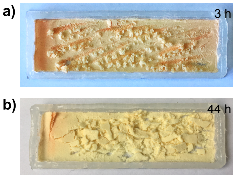
Figure S3. a) After 3 hours, only the surface layers of solid reaction mixture underwent the reaction (indicated by discolouration) whereas the colour of the inner layers suggested that the reaction was still in progress. b) In the case of 44 h exposure, scratching the surface with a spatula revealed a complete discolouration of the reaction mixture. This observation prompted us to develop a ball milling approach which facilitates mass transfer in the solid-state.
