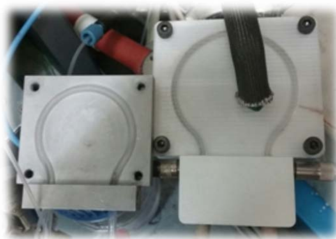
Fig. S7. Modified reactor design for multi-phase reaction. In order to achieve organic-aqueous phase separation during each oscillation pass, it is necessary to have a high cross-sectional velocity; because the carrier fluid is compressible, there is a delay between changing syringe direction and affecting droplet motion. Extending the length of the reactor by 4 cm after the optical detection point prevents the droplet from exiting the reactor during this delay. Additionally, in the multi-phase configuration, a higher flow rate is used when switching directions (e.g., 1500 \mu\text{L}/\text{min} ) before switching back to the target flow rate (e.g., 750 \mu\text{L}/\text{min} ) to decrease the delay between the reversal of syringe pump direction and the reversal of droplet motion. The aluminium chuck is further extended after the optical detection point to ensure that the slug remains at the desired reaction temperature even with partial overshooting.
