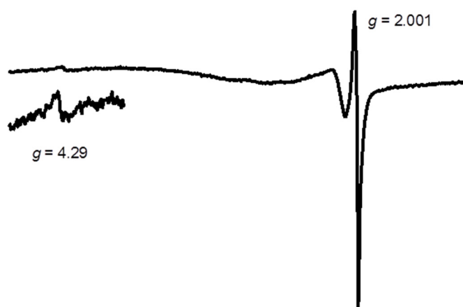
Fig. S21 EPR spectrum of Li + @C 60 C 1 recorded in PhCN at 4 K after photoexcitation showing the triplet signal of Li + @C 60 •- at g = 2.001 and g = 4.29 . The signal at g = 2.001 shows the formation of radicals as the result of a photoinduced electron transfer in the host-guest system, while the feature at g = 4.29 arise from the triplet excited states of Li + @C 60 . Although the latter signal is weak, it supports the conclusion that the charge separated state is driven by triplet excited states of Li + @C 60 , which was indeed directly monitored in the nanosecond transient spectra in Fig. S19, in which the radical species form at \lambda = 450, 800 and 1035 nm while the triplet states of Li + @C 60 decay at \lambda = 750 nm (Fig. S19, inset). The EPR spectra were used as supporting data in similar ET processes of Li + @C 60 with electron donors. S8,S9
