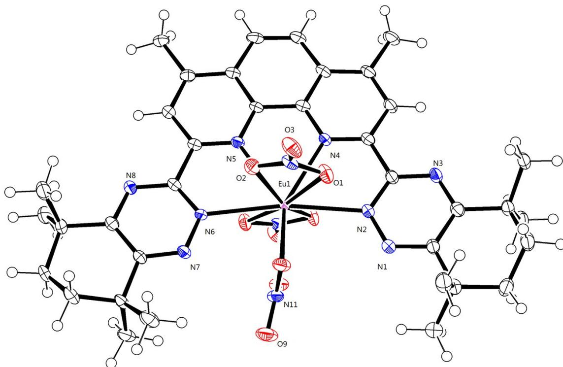
**Fig. S1.** X-ray crystallographic structure of 4,7-Me-CyMe<sub>4</sub>-BTPhen–Eu(NO<sub>3</sub>)<sub>3</sub> complex (*c-c* conformer). Thermal ellipsoids are shown at 50 % probability. Additional solvent molecules are omitted for clarity.
