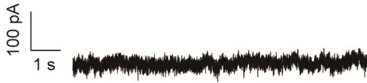
Figure S3. The raw current trace from antibody-modified nanopore in 1 M KCl.
