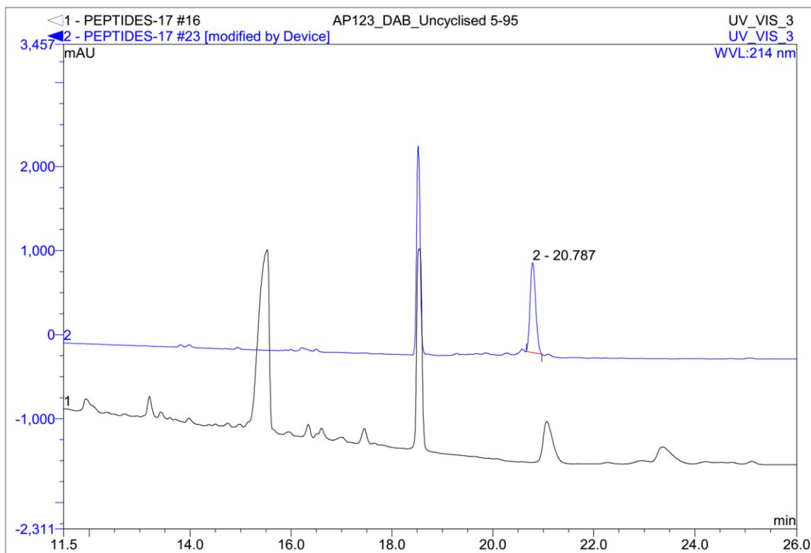
**Fig.11:** HPLC trace showing the progress of cyclisation reaction for analogue **5**: conversion of the uncyclized protected teixobactin analogue  $t_R = 15.527$  min (shown in black) to the cyclized protected teixobactin analogue  $t_R = 20.787$  min (shown in blue) (Gradient: 5-95% in 25 min)
