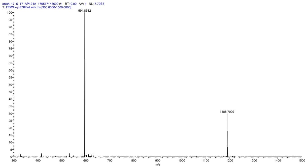
**Fig. 14:** HRMS spectra from LC-MS of HPLC purified teixobactin analogue **5**. Exact Mass calcd. for  $C_{56}H_{93}N_{13}O_{15} = 1187.6914$ , found  $M+H^+ = 1188.7009$  and  $M/2 + H^+ = 594.8532$
