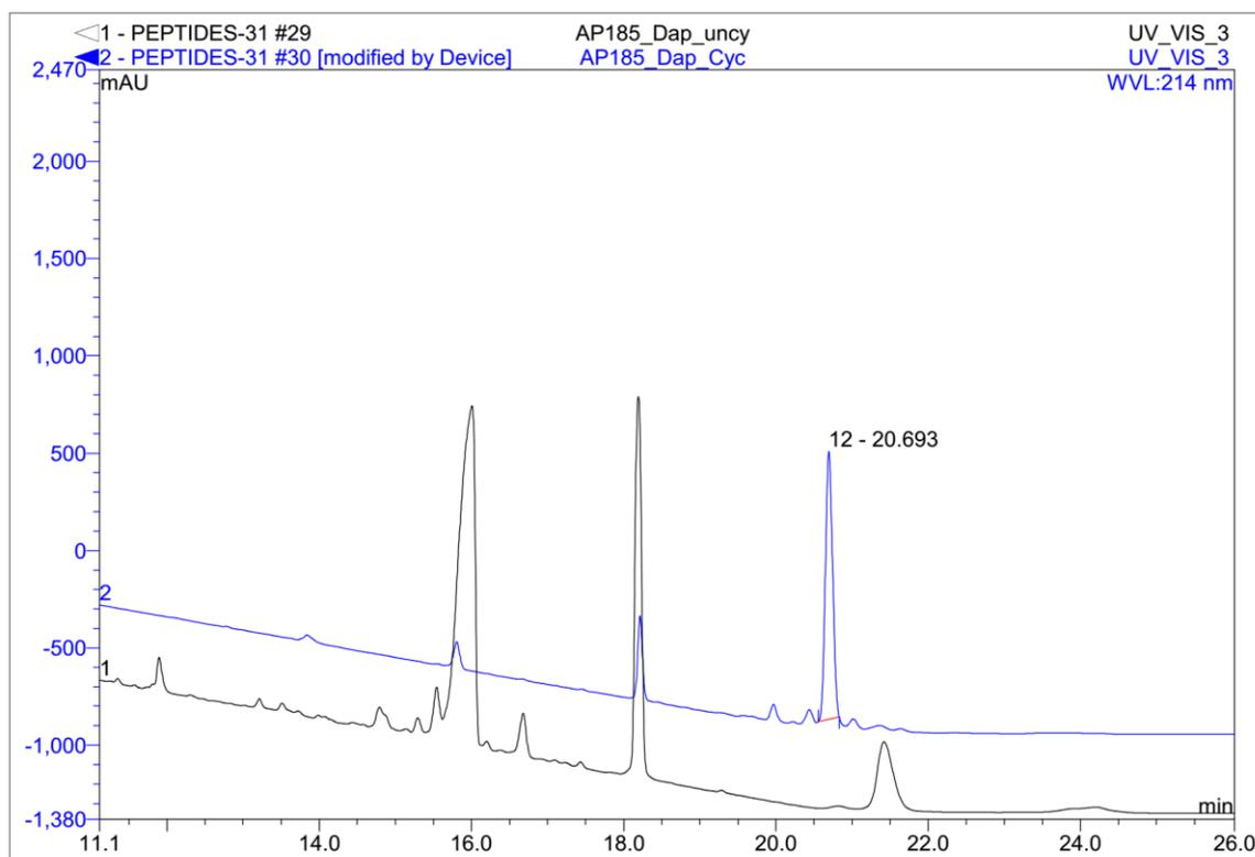
**Fig. 17:** HPLC trace showing the progress of cyclisation reaction of analogue **7**: conversion of the uncyclized protected teixobactin analogue  $t_R = 16.010$  min (shown in black) to the cyclized protected teixobactin analogue  $t_R = 20.693$  min (shown in blue) (Gradient: 5-95% in 25 min)
