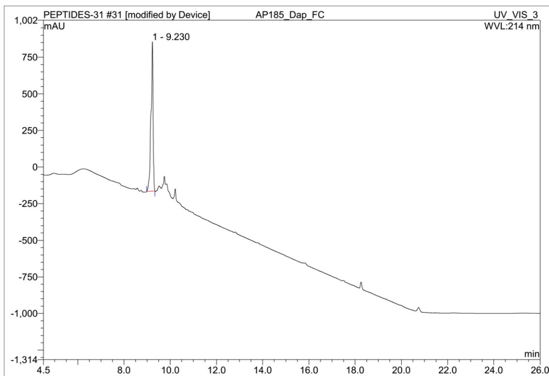
**Fig 18:** HPLC trace of crude teixobactin analogue **7**  $t_R = 9.230$  min (gradient: 5-95% ACN in 25 min using A: 0.1% HCOOH in water, B: ACN)
