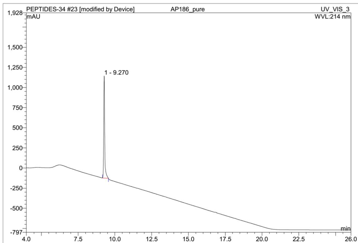
**Fig. 5:** HPLC trace of HPLC purified teixobactin analogue **2** (gradient: 5-95% ACN in 25 min using A: 0.1% HCOOH in water, B: ACN)
