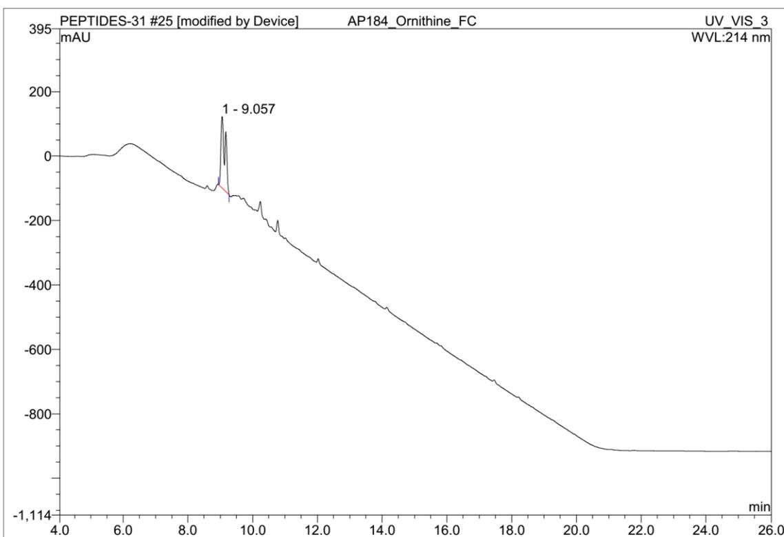
**Fig 8:** HPLC trace of crude teixobactin analogue **3**  $t_R = 9.057$  min (gradient: 5-95% ACN in 25 min using A: 0.1% HCOOH in water, B: ACN)
