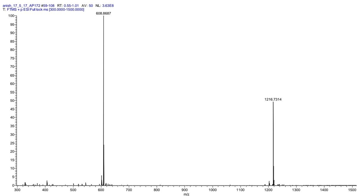
**Fig. 4:** HRMS spectra from of HPLC purified teixobactin analogue **1**. Exact Mass calcd. for  $C_{58}H_{97}N_{13}O_{15} = 1215.7227$ , found  $M+H^+ = 1216.7314$  and  $M/2 + H^+ = 608.8687$
