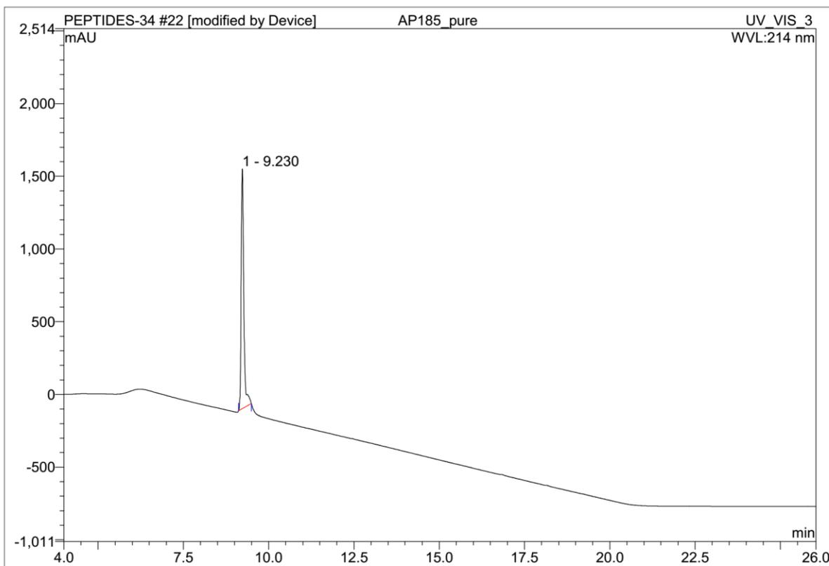
**Fig. 19:** HPLC trace of HPLC purified teixobactin analogue **7** (gradient: 5-95% ACN in 25 min using A: 0.1% HCOOH in water, B: ACN)
