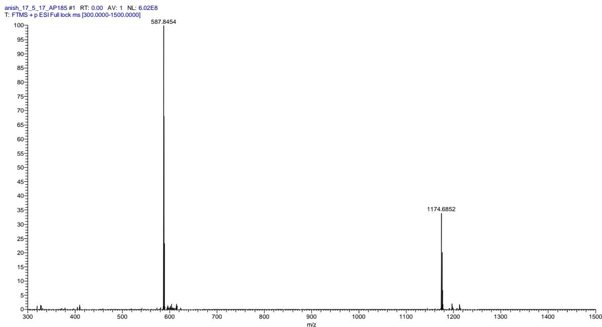
**Fig. 20:** ESI-MS spectra from LC-MS of HPLC purified teixobactin analogue **7**. Exact Mass calcd. for  $C_{55}H_{91}N_{13}O_{15} = 1173.6758$ , found  $M+H^+ = 1174.6852$  and  $M/2 + H^+ = 587.8454$
