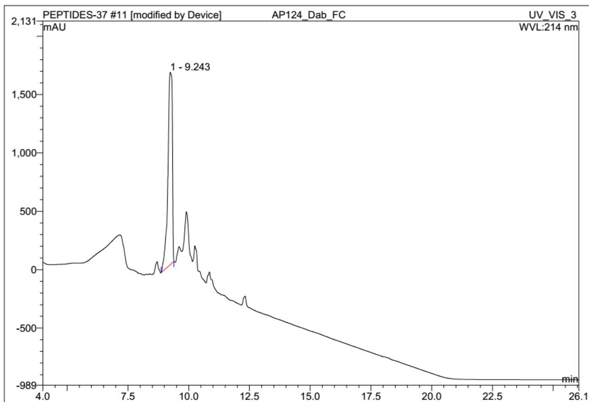
**Fig. 12:** HPLC trace of crude teixobactin analogue **5**  $t_R = 9.243$  min (gradient: 5-95% ACN in 25 min using A: 0.1% HCOOH in water, B: ACN)
