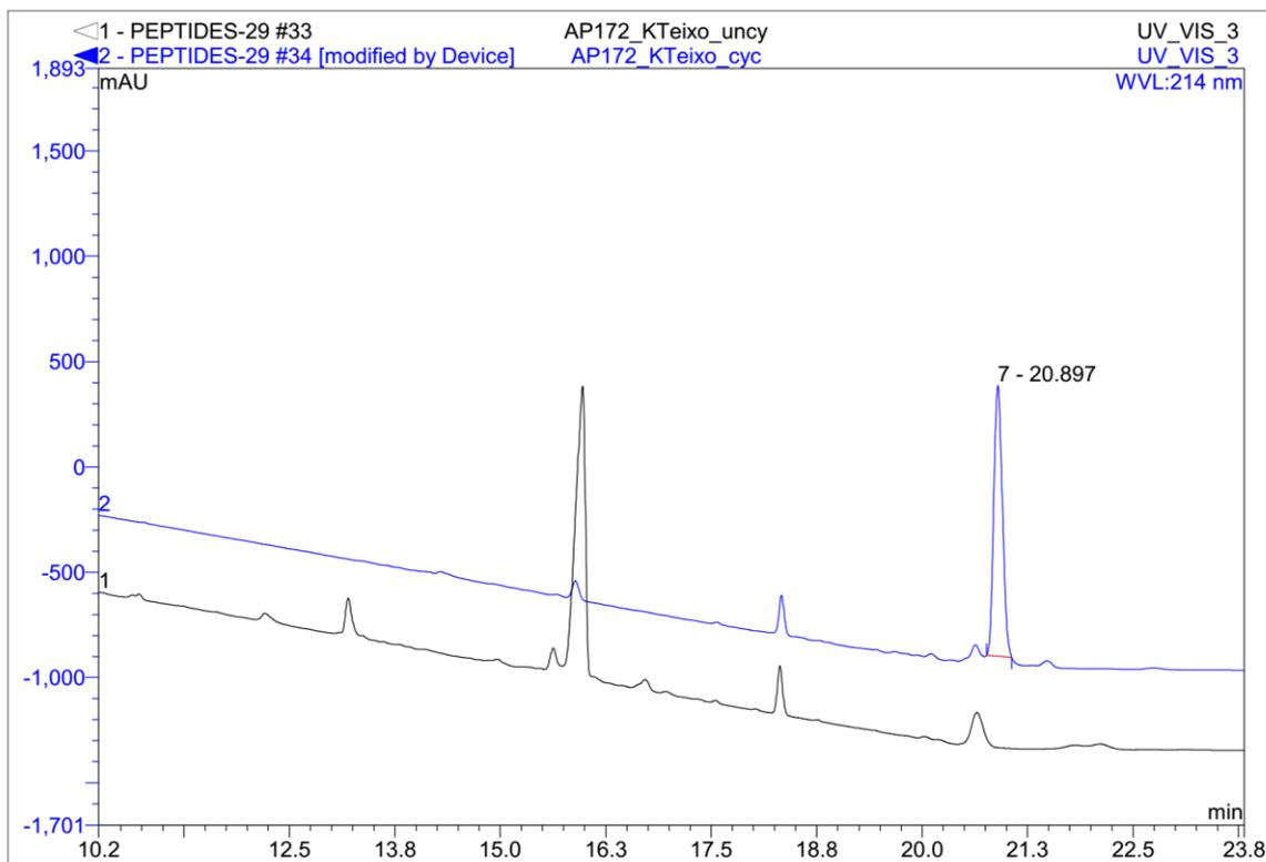
**Fig. 1:** HPLC trace showing the progress of the cyclisation reaction for analogue **1**: conversion of the uncyclized protected teixobactin analogue  $t_R = 15.977$  min (shown in black) to the cyclized protected teixobactin analogue  $t_R = 20.897$  min (shown in blue) (Gradient: 5-95% in 25 min)
