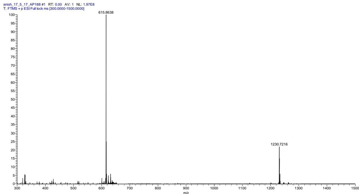
**Fig. 16:** ESI-MS spectra from LC-MS of HPLC purified teixobactin analogue **6**. Exact Mass calcd. for  $C_{57}H_{95}N_{15}O_{15} = 1229.7132$ , found  $M+H^+ = 1230.7216$  and  $M/2 + H^+ = 615.8638$
