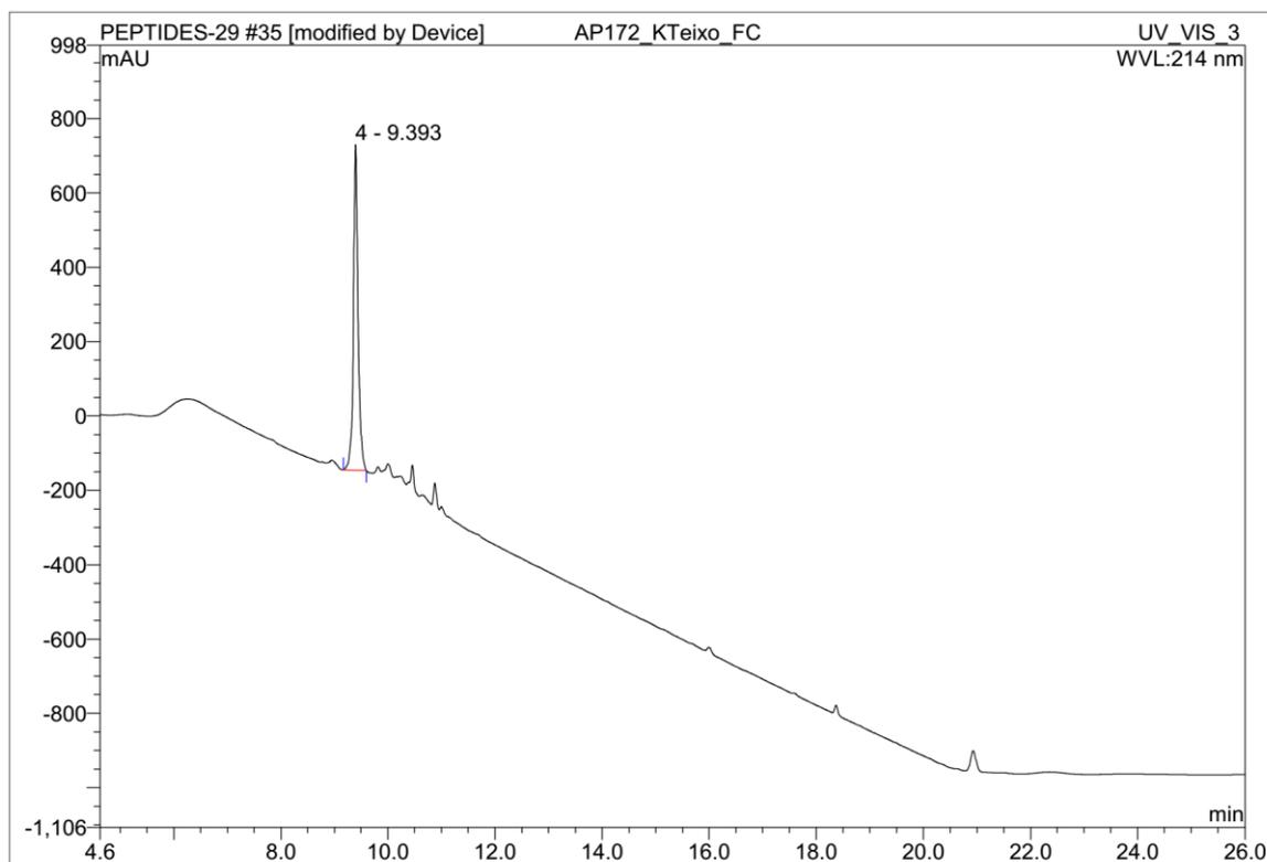
**Fig. 2:** HPLC trace of crude teixobactin analogue **1**  $t_R = 9.393$  min (gradient: 5-95% ACN in 25 min using A: 0.1% HCOOH in water, B: ACN)
