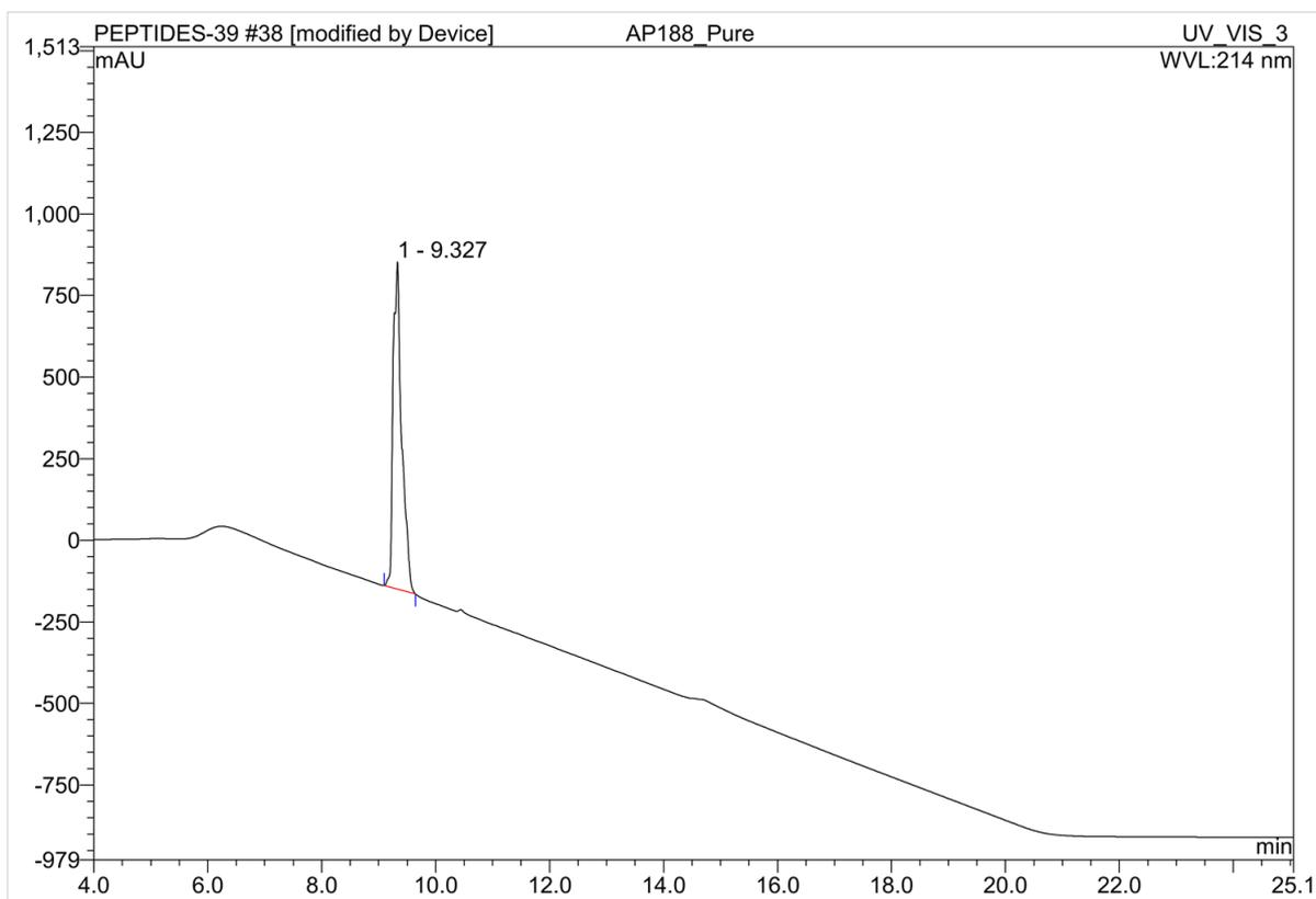
**Fig. 21:** HPLC trace of HPLC purified teixobactin analogue **8** (gradient: 5-95% ACN in 25 min using A: 0.1% HCOOH in water, B: ACN)
