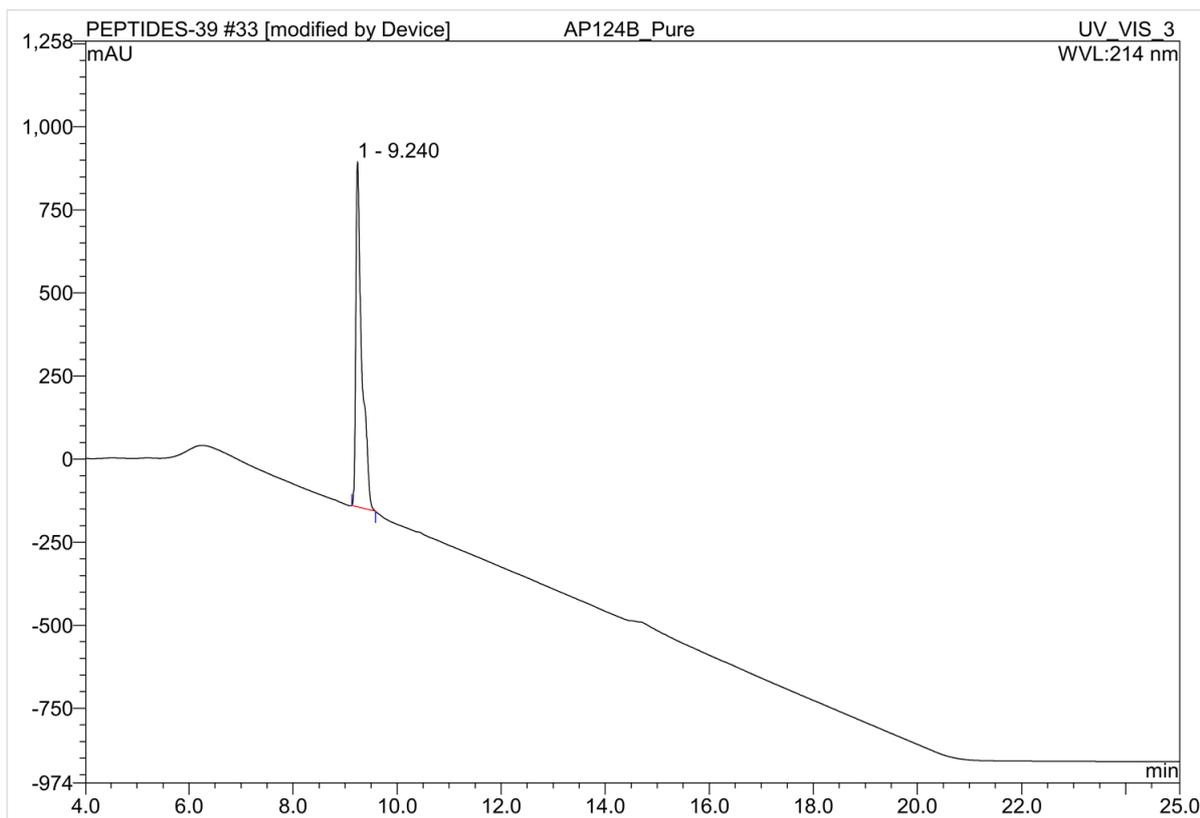
**Fig. 15:** HPLC trace of HPLC purified teixobactin analogue **6** (gradient: 5-95% ACN in 25 min using A: 0.1% HCOOH in water, B: ACN)
