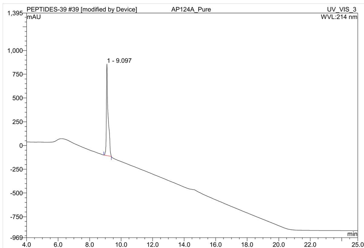
**Fig. 13:** HPLC trace of HPLC purified teixobactin analogue **5** (gradient: 5-95% ACN in 25 min using A: 0.1% HCOOH in water, B: ACN)
