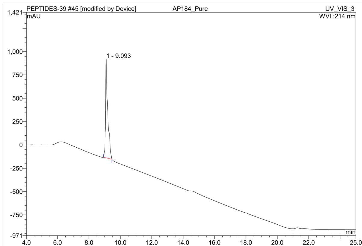
**Fig 9:** Ornithine HPLC trace of HPLC purified teixobactin analogue **3** (gradient: 5-95% ACN in 25 min using A: 0.1% HCOOH in water, B: ACN)
