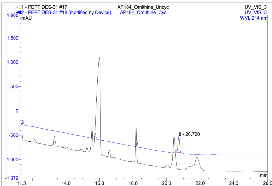
**Fig. 7:** HPLC trace showing the progress of the cyclisation reaction for analogue **3**: conversion of the uncyclized protected teixobactin analogue  $t_R = 16.000$  min (shown in black) to the cyclised protected teixobactin analogue  $t_R = 20.720$  min (shown in blue) (Gradient: 5-95% in 25 min)
