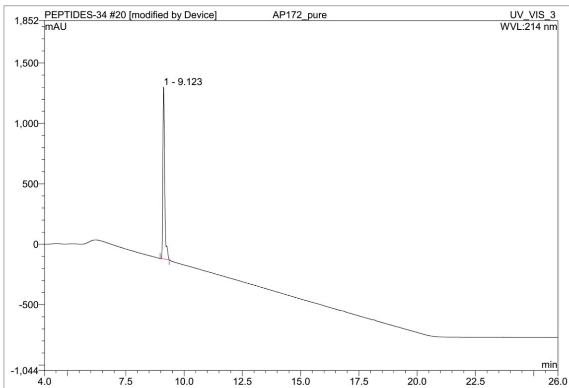
**Fig. 3:** HPLC trace of HPLC purified teixobactin analogue **1** (gradient: 5-95% ACN in 25 min using A: 0.1% HCOOH in water, B: ACN)
