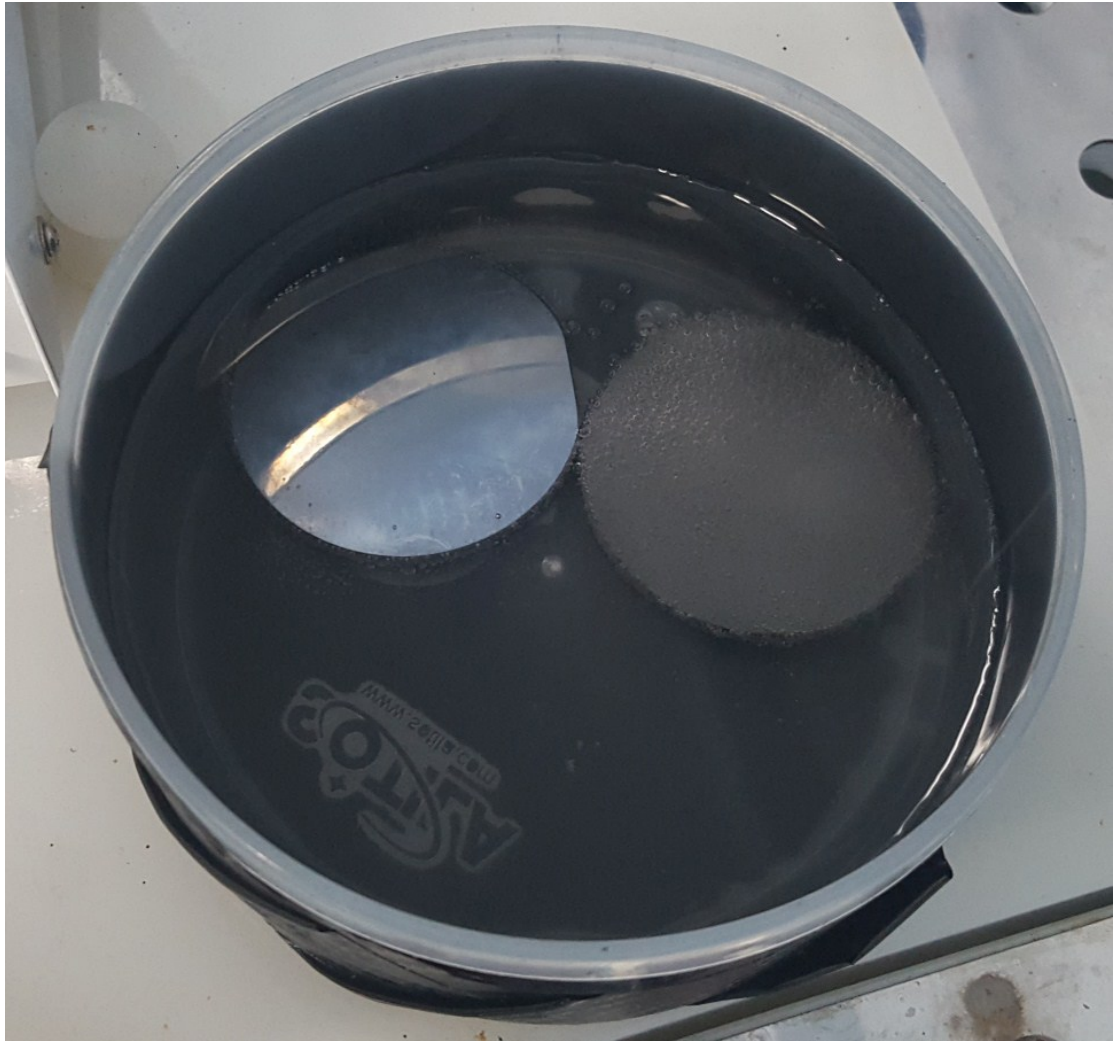
Fig. S6 Digital photos of HF/HNO 3 etching of control sample (left) and MACE treated wafer (right).
