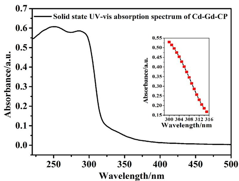
Figure S14. Solid state UV-visible absorption spectrum for Cd-Gd-CP.
