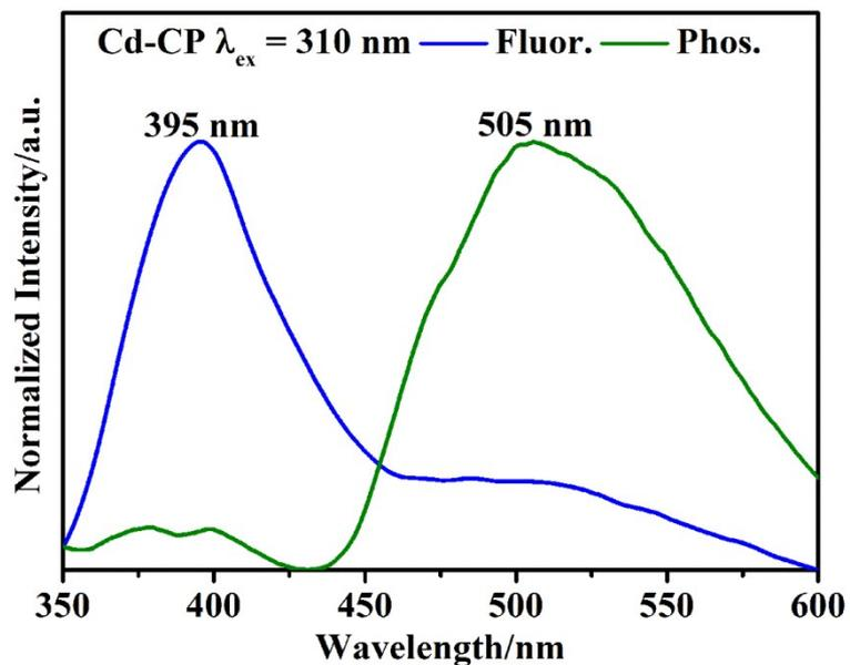
**Figure S7.** Room-temperature solid-state emission spectra of Cd-CP under excitation wavelength at 310 nm.
