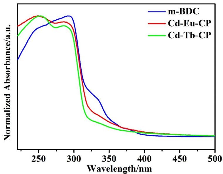
**Figure S8.** Solid-state UV-visible absorption spectra for m-BDC and Cd-Eu/Tb-CPs.
