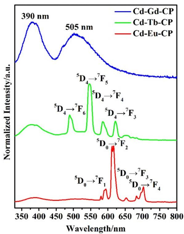
**Figure S6.** Room-temperature solid-state emission spectra of Cd-Eu\Tb\Gd-CPs under excitation wavelength at 310 nm.
