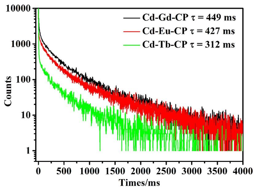
**Figure S10.** Time-resolved emission decay curves at 505 nm for Cd-Eu/Tb/Gd-CPs under ambient conditions.
