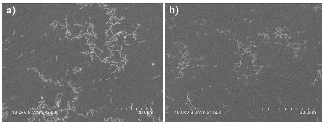
**Fig. S12** SEM images of samples obtained from drying the solutions of (a) *R*-BNS-BPP and (b) *S*-BNS-BPP in methanol-water (50:50 v/v). Concentration:  $1 \times 10^{-5}$  mol/L for BPP,  $0.5 \times 10^{-5}$  mol/L for BNS.
