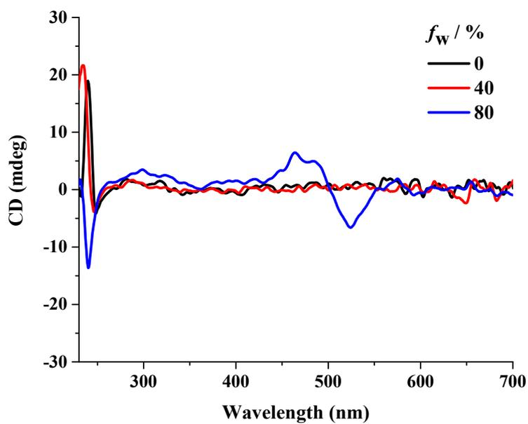
**Fig. S6** CD spectra of *R*-BNS-BPP in methanol-water. Concentration:  $1 \times 10^{-5}$  mol/L for BPP,  $0.5 \times 10^{-5}$  mol/L for BNS.
