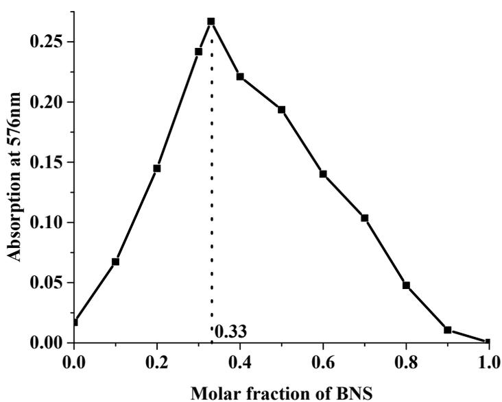
Fig. S2 The Job's plot of the absorption at 576 nm of BNS-BPP in methanol-water (50:50 v/v). The total concentration of BPP and BNS is fixed at  $2 \times 10^{-5}$  mol/L. The optimum mixing ratio of BNS: BPP is found to be 1.0 : 2.0.
