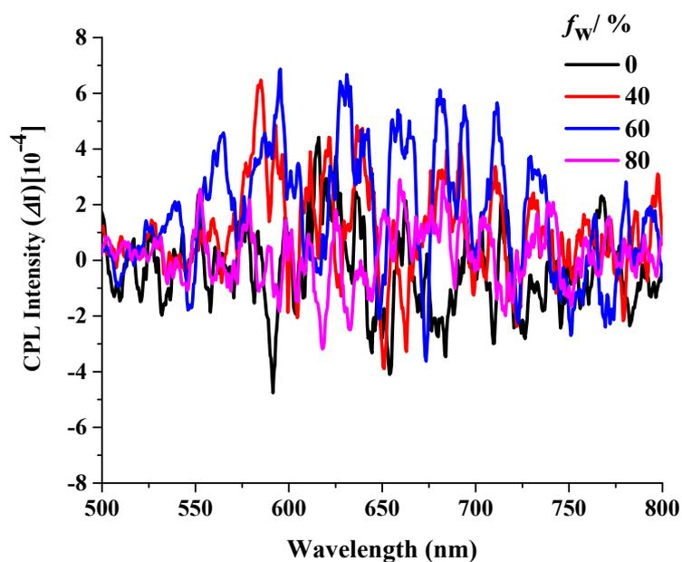
**Fig. S9** CPL spectra of *R*-BNS-BPP in methanol-water. Concentration:  $1 \times 10^{-5}$  mol/L for BPP,  $0.5 \times 10^{-5}$  mol/L for BNS.
