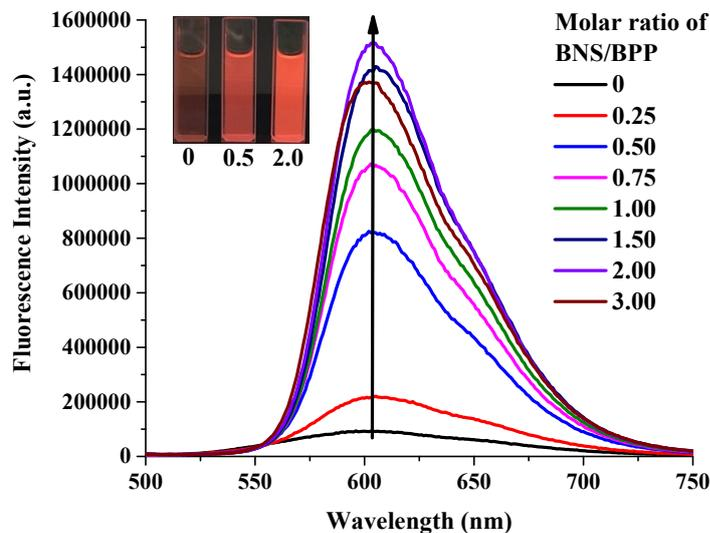
**Fig. S7** Fluorescent spectra of *R*-BNS-BPP in MeOH-H<sub>2</sub>O (50:50 v/v) solution (excitation: 467 nm). The concentration of BPP is fixed at  $1.0 \times 10^{-5}$  mol/L. Insert: photographs taken under UV illumination (365 nm).
