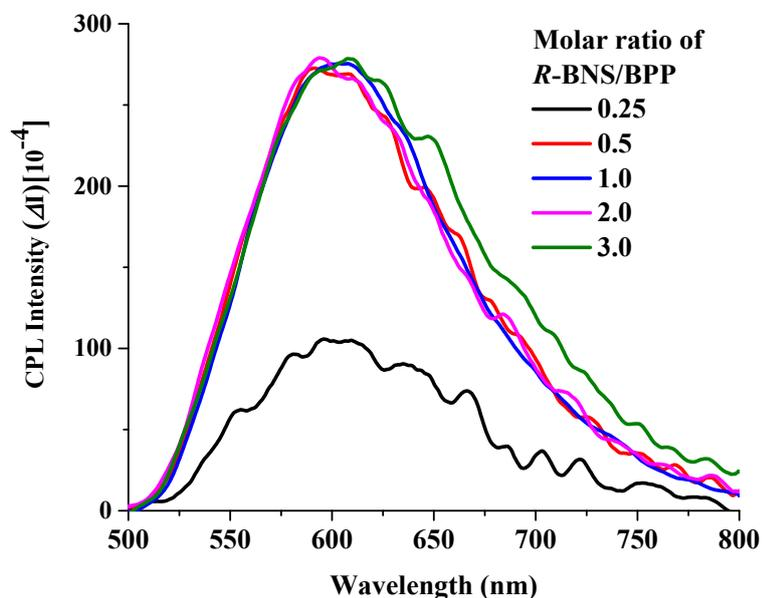
**Fig. S8** CPL spectra of *R*-BNS-BPP in methanol-water. Concentration:  $1 \times 10^{-5}$  mol/L for BPP, DC (intensity of the unpolarized emission) is fixed at 0.5.
