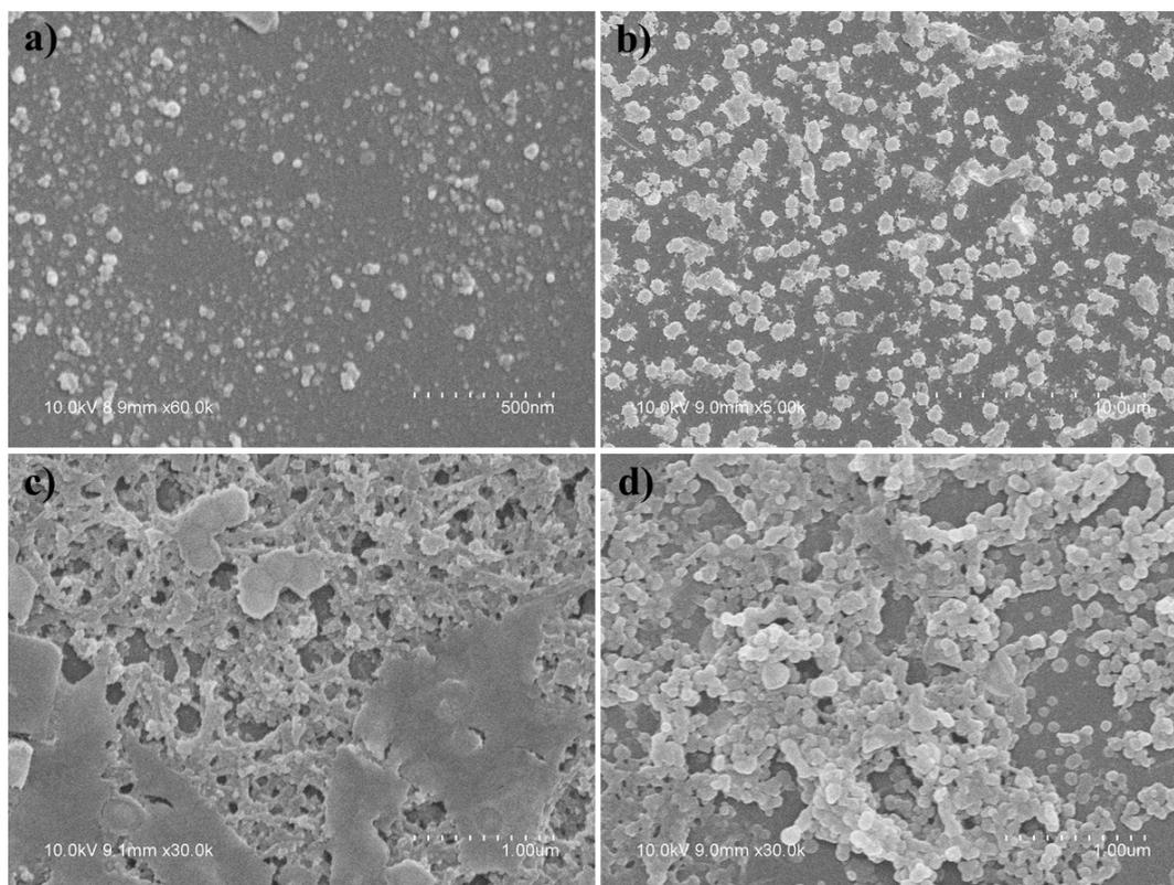
**Fig. S11** SEM images of samples obtained from drying the solutions of BNS-BPP in methanol-water (a, b, c and d for  $f_w = 0, 40\%, 60\%$  and  $80\%$ ). Concentration:  $1 \times 10^{-5}$  mol/L for BPP,  $0.5 \times 10^{-5}$  mol/L for BNS.
