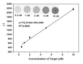
Fig. S6. Relationship between the relative CL intensity and catalyst concentration without H2. Inset: CL images of catalyst at different concentrations. Experimental conditions: 5  $\mu$ g of MMPs and 250 ng/mL SA-HRP.
