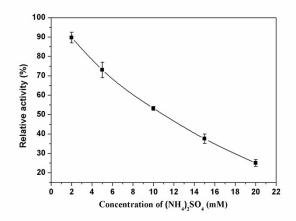
Fig. S8. Inhibition effects of  $(NH_4)_2SO_4$  on phosphorylation. Experimental conditions: 0.12 U/mL PNK, 5 µg MMPs, 50 nM PNK-H2, and 250 ng/mL SA-HRP.
