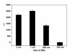
**Fig. S2.** Effects of the size of MMPs on the relative CL intensity of the sensing system. Experimental conditions: 5 μg of MMPs, 50 nM H2, and 200 ng/mL SA-HRP.
