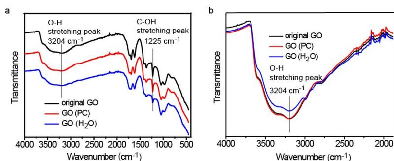
**Figure S9.** (a) FT-IR spectra of as-prepared GO sheets, and the GO sheets collected from GO (PC) or GO (H<sub>2</sub>O) dispersions after storing under ambient environments for two weeks, and (b) corresponding detailed FT-IR spectra between 4000–2000 cm<sup>-1</sup> of as-prepared GO sheets, GO (PC) and GO (H<sub>2</sub>O). The three spectra are normalized with respect to the 1723 cm<sup>-1</sup>.
