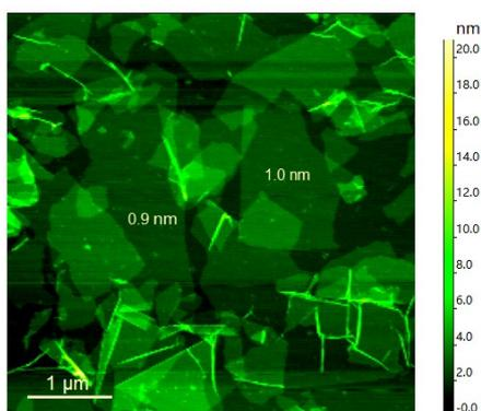
**Figure S2.** AFM image of GO sheets from GO (PC) dispersion.
