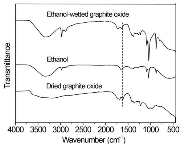
**Figure S4.** FT-IR spectra of ethanol-wetted graphite oxide, ethanol and dried graphite oxide.
