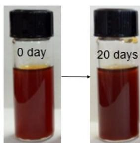
**Figure S3.** Stability test of concentrated GO (PC) dispersion.
