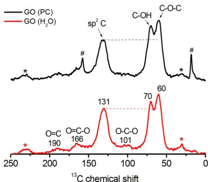
**Figure S10.** Solid-state  $^{13}\text{C}$  NMR spectra of the GO sheets collected from GO ( $\text{H}_2\text{O}$ ) and GO (PC) after storing under ambient environment for 28 days. Direct  $^{13}\text{C}$  pulse spectra obtained with 10.0 kHz MAS. The spectra are normalized with respect to the height of the signal at 60 ppm. Asterisks (\*) denote spinning sidebands. The weak signals indicated by pound sign (#) in the GO (PC) spectrum result from residual PC.
