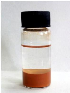
**Figure S1.** Insolubilization of graphite oxide in ethanol.
