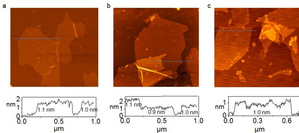
**Figure S6.** AFM images of GO sheets with thickness profiles; (a) GO (DMSO), (b) GO (EG), and (c) GO (DMF).
