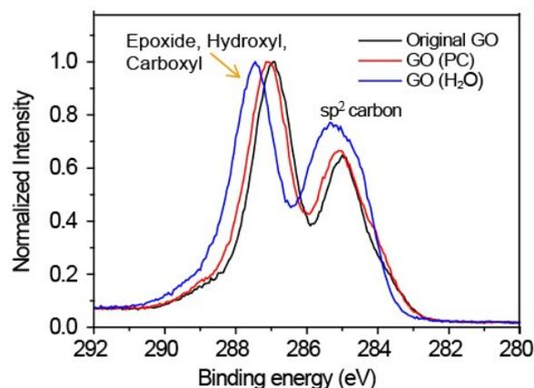
**Figure S8.** C 1s XPS spectra of as-prepared GO sheets and those collected from the GO (PC) or GO (H<sub>2</sub>O) dispersion after storing under ambient environment for two weeks.
