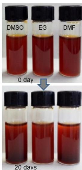
**Figure S7.** Stability of concentrated GO dispersions in DMSO, EG and DMF respectively. The photographs demonstrate that the organic dispersions of GO are also stable without serious aggregation after a long-term storage of 20 days; GO concentration =  $10 \text{ mg mL}^{-1}$ .
