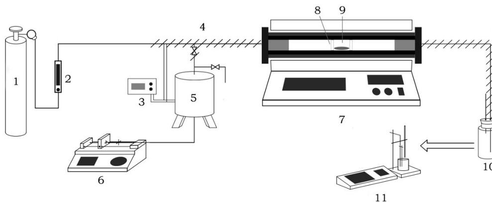
**Figure S2.** Schematic diagram of the AlN hydrolyzation setup: 1, Nitrogen cylinder; 2, flow meter; 3, thermoregulator; 4, heat type; 5, steam generator; 6, syringe pump; 7, tube furnace; 8, silica wool; 9, AlN and catalyst; 10, water; 11, pH meter.
