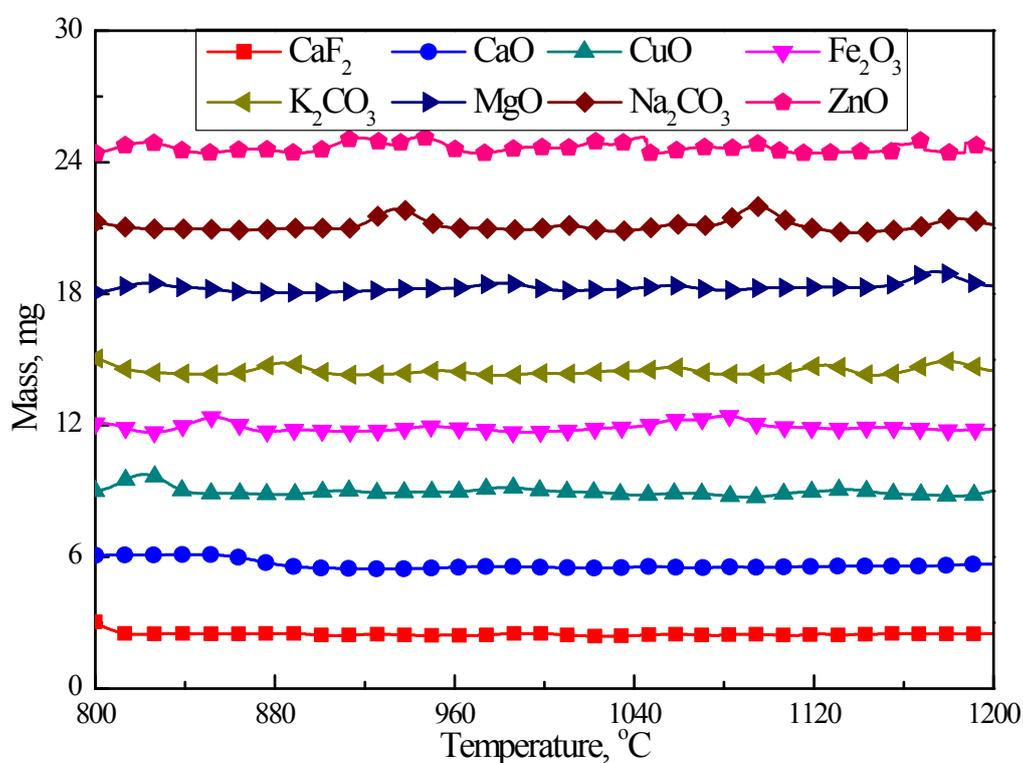
Fig.S1 The blank tests of different catalysts with TGA (sample loading: 30 mg; catalyst loading: 5 wt%; gas flow:  $0.5 \text{ L min}^{-1}$ ; heating rate:  $20 \text{ }^\circ\text{C min}^{-1}$ )
