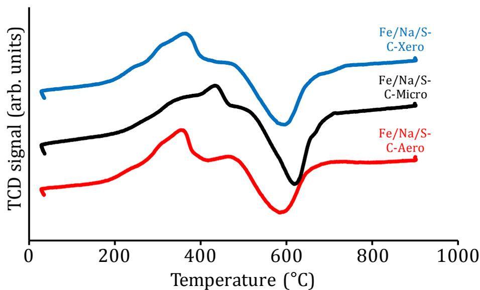
**Figure S5.** Hydrogen temperature programmed reduction ( $H_2$ -TPR) profiles of the calcined catalysts.
