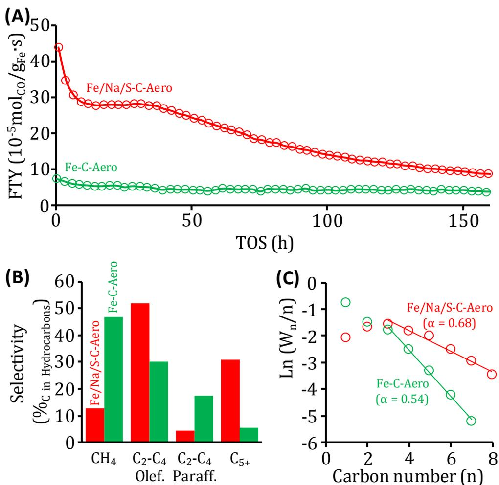
**Figure S7.** (A) Iron-weight based activity (FTY) over time on stream (TOS), (B) hydrocarbon product selectivity after 150 h TOS (CO conversion = 7.5 and 18 %; CO<sub>2</sub> selectivity = 43%<sub>C</sub> for both catalysts), and (C) corresponding Anderson–Schulz–Flory (ASF) plots of the C<sub>1</sub>-C<sub>8</sub> product fractions with chain growth probability ( $\alpha$ ) based on the C<sub>3</sub>-C<sub>8</sub> products of the Fe-C-Aero and Fe/Na/S-C-Aero catalysts.
