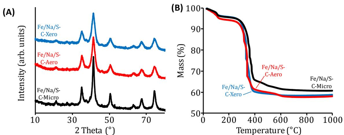
**Figure S4.** (A) X-ray diffraction patterns, and (B) thermogravimetric analysis under synthetic air atmosphere of the Fe/Na/S-C-Micro (black), Fe/Na/S-C-Xero (blue), and Fe/Na/S-C-Aero (red) catalysts.
