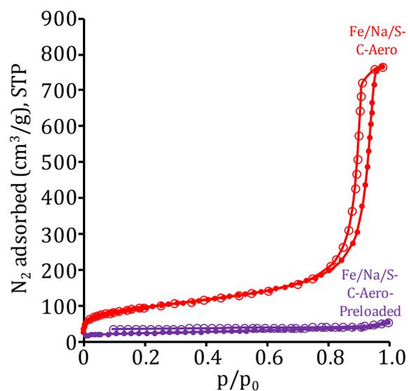
**Figure S9.** Nitrogen physisorption isotherms of the Fe/Ni/S-C-Aero and Fe/Ni/S-C-Aero-Preloaded catalysts measured at -196°C.
