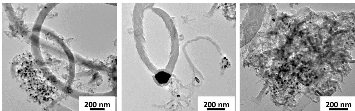
**Figure S11.** TEM images of the spent Fe/Ni/S-C-Aero catalyst after ~165 h TOS.
