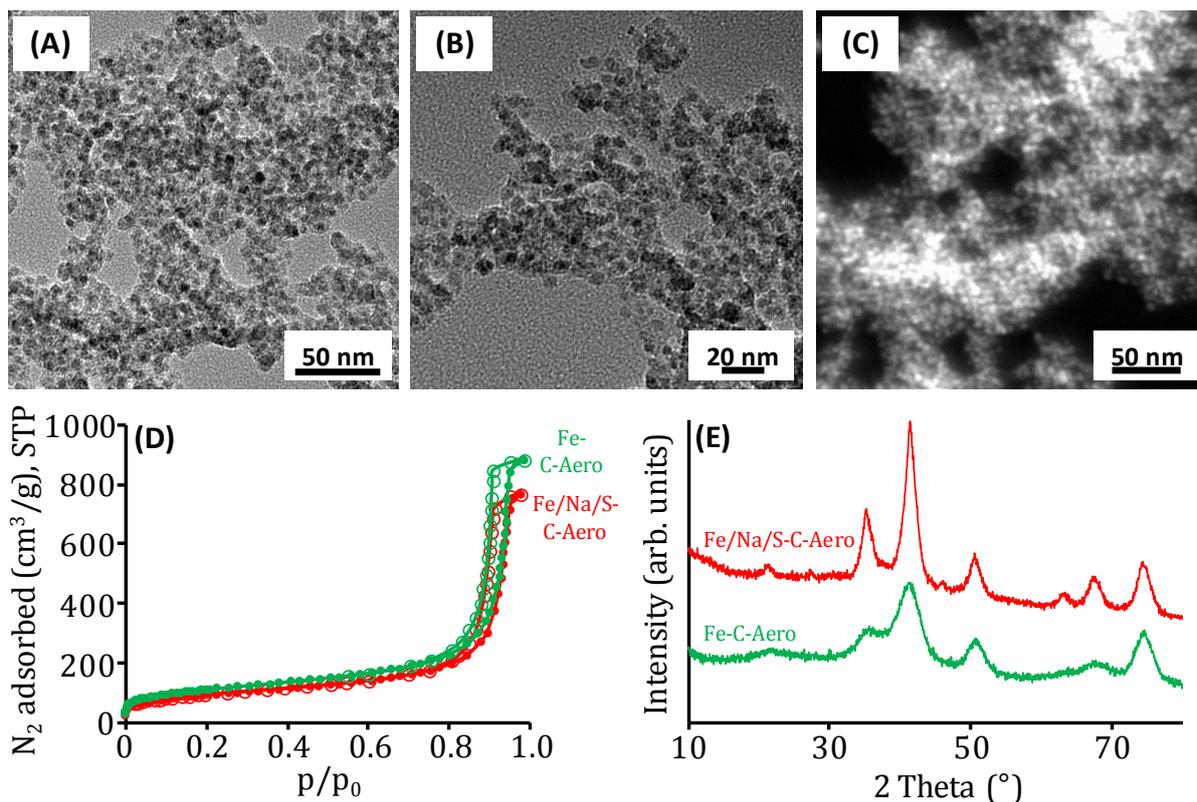
**Figure S6.** (A-C) TEM and HAADF-STEM images, (D) nitrogen physisorption isotherm measured at  $-196^\circ\text{C}$ , and (E) X-ray diffraction patterns of the unpromoted Fe-C-Aero catalyst. The curves of the promoted Fe/Na/S-C-Aero catalyst are shown for comparison in (D) and (E).
