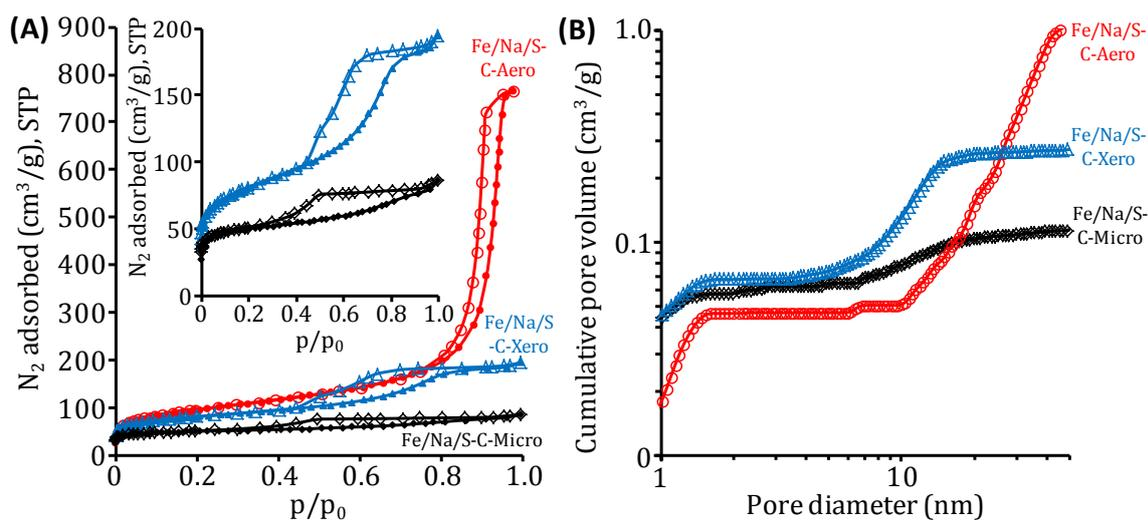
**Figure S2.** (A) Nitrogen physisorption isotherms measured at  $-196^\circ C$  and (B) corresponding cumulative QSDFT pore size distributions of the Fe/N a/S-C-Micro (black, diamonds), Fe/N a/S-C-Xero (blue, triangles), and Fe/N a/S-C-Aero (red, circles) catalysts.
