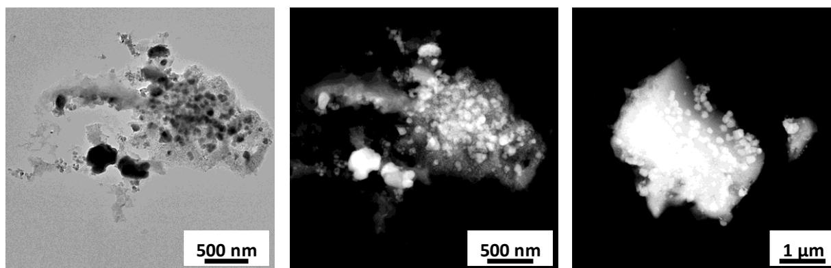
**Figure S8.** TEM and HAADF-STEM images of the catalyst “Fe-C-Aero-Preloaded” after pyrolysis.
