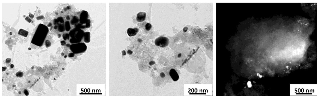
**Figure S10.** TEM and HAADF-STEM images of the spent Fe/Ni/S-C-Micro catalyst after ~165 h TOS.
