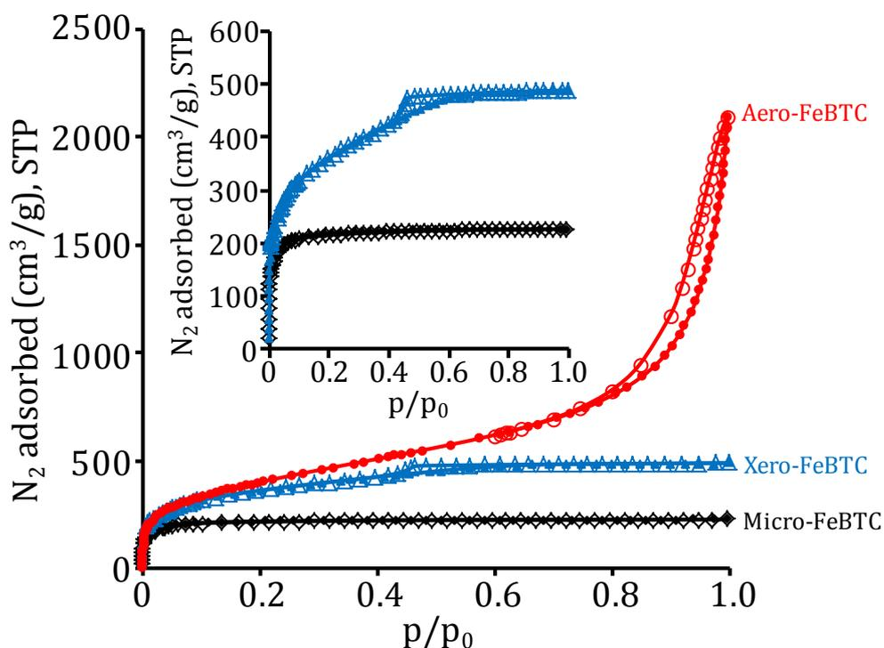
**Figure S1.** Nitrogen physisorption isotherms measured at  $-196^\circ C$  of the MOF precursors Micro-FeBTC (black, diamonds), Xero-FeBTC (blue, triangles), and Aero-FeBTC (red, circles).
