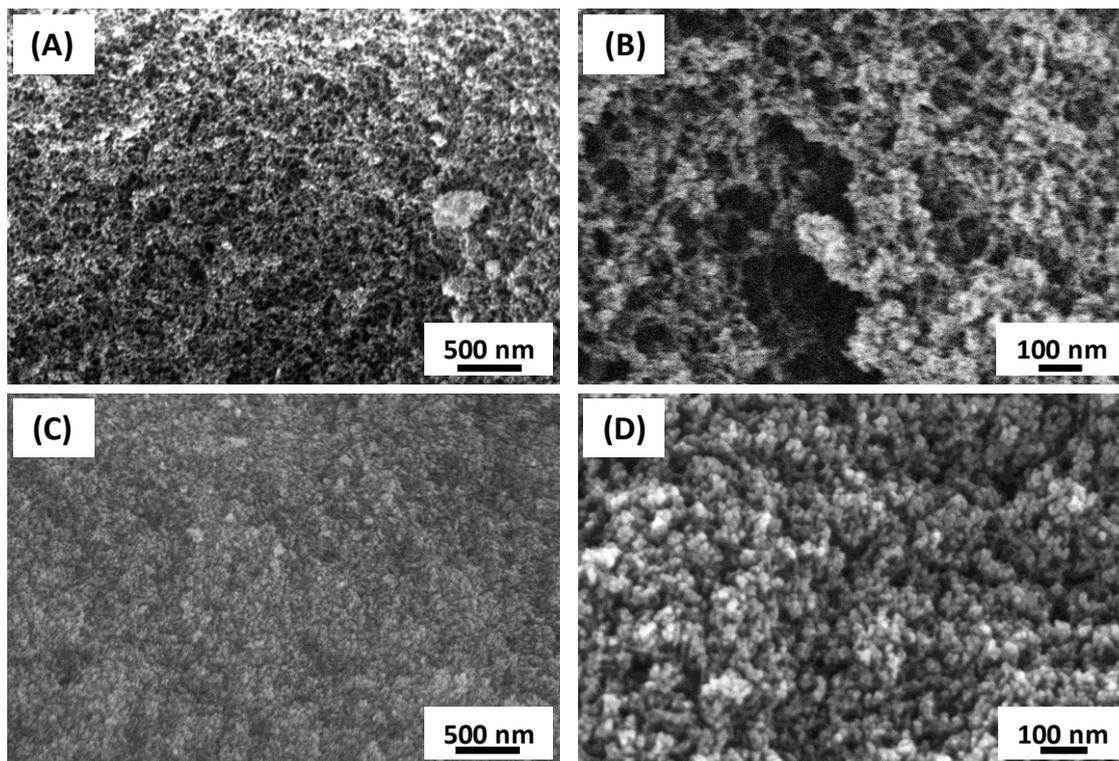
**Figure S3.** Scanning electron microscopy images of (A,B) Aero-FeBTC and (C,D) Fe/Na/S-C-Aero.
