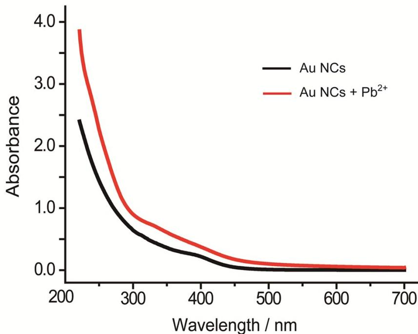
Fig. S5 UV-vis absorption spectra of Au-NCs in the absence and presence of  $\text{Pb}^{2+}$ .
