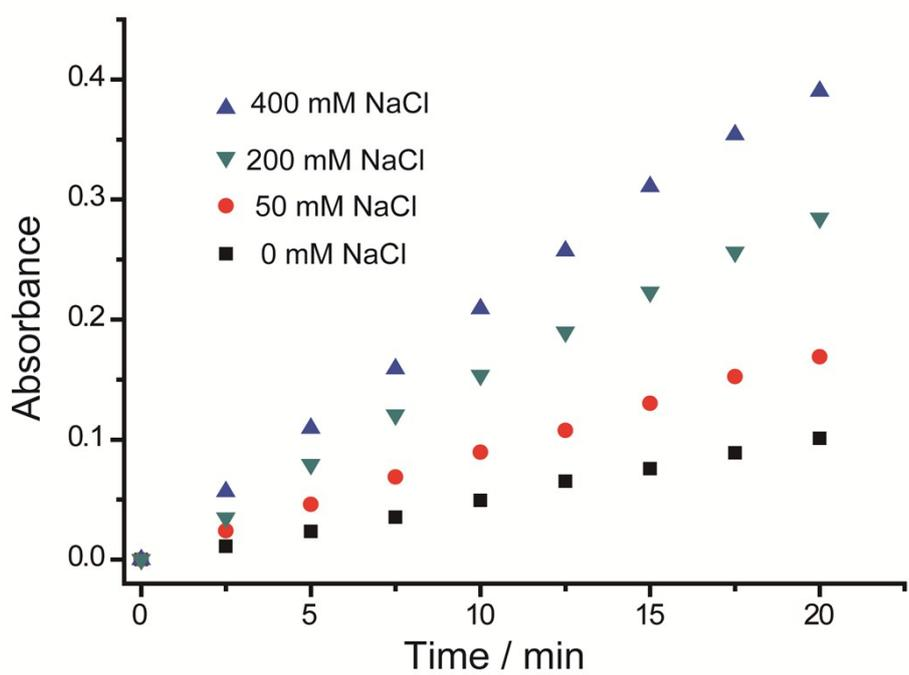
Fig. S7 Reaction kinetics of the system in the presence of different concentrations of NaCl.
