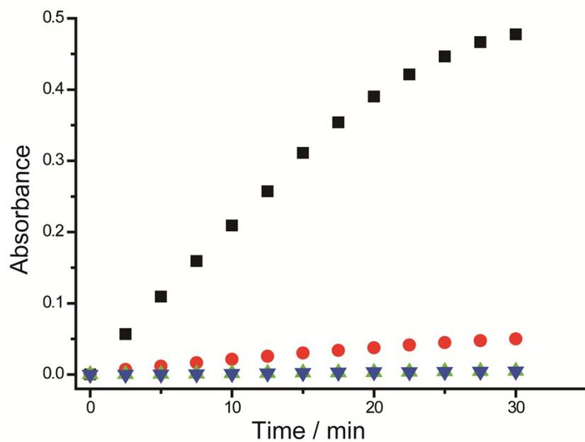
Fig. S3 The kinetic curves of TMB-H<sub>2</sub>O<sub>2</sub> (▼) and TMB-H<sub>2</sub>O<sub>2</sub> in the presence of Pb<sup>2+</sup> (▲), Au-NCs (●), and both the Pb<sup>2+</sup> and Au-NCs (★).
