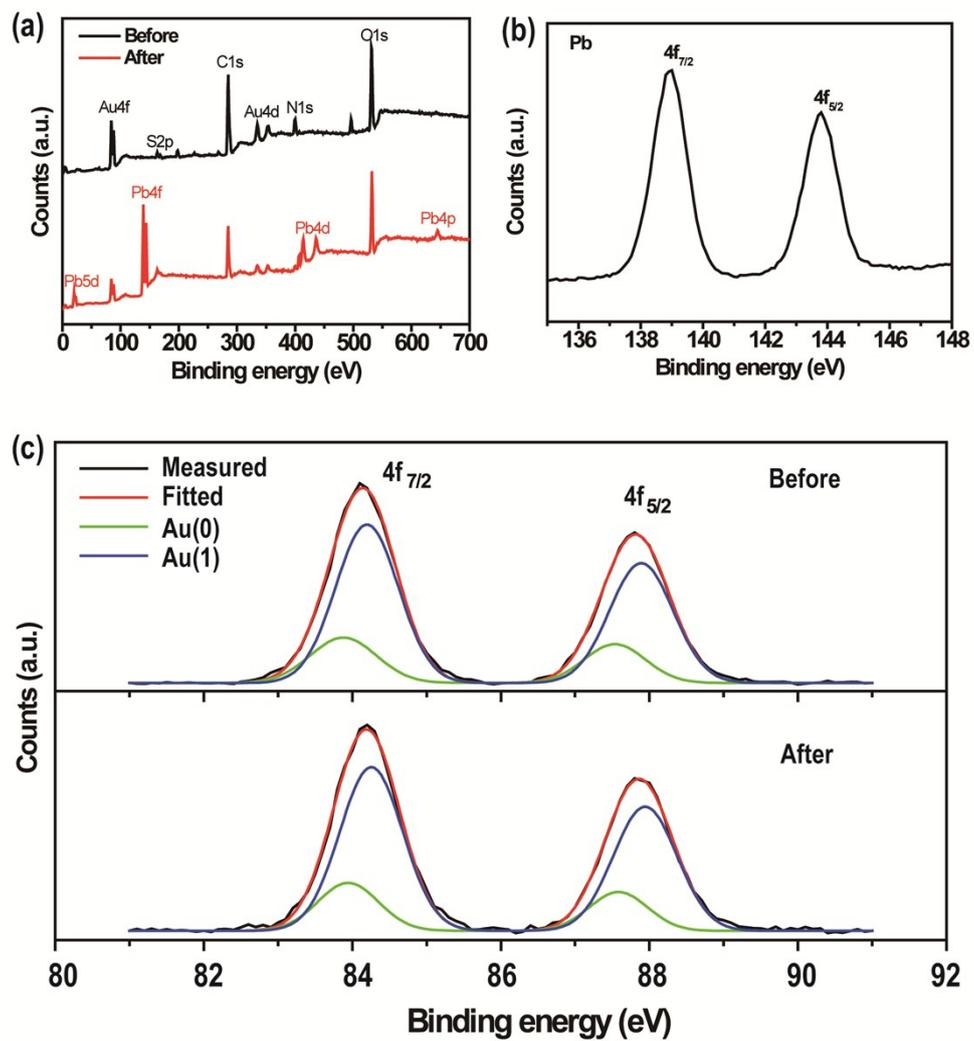
Fig.S8 XPS spectra of (a) all the surface elements of Au-NCs before and after the addition of  $Pb^{2+}$ , (b) high-resolution Pb 4f spectra of Au-NCs after the addition of  $Pb^{2+}$ , and (c) high-resolution Au 4f spectra before and after the addition of  $Pb^{2+}$ .
