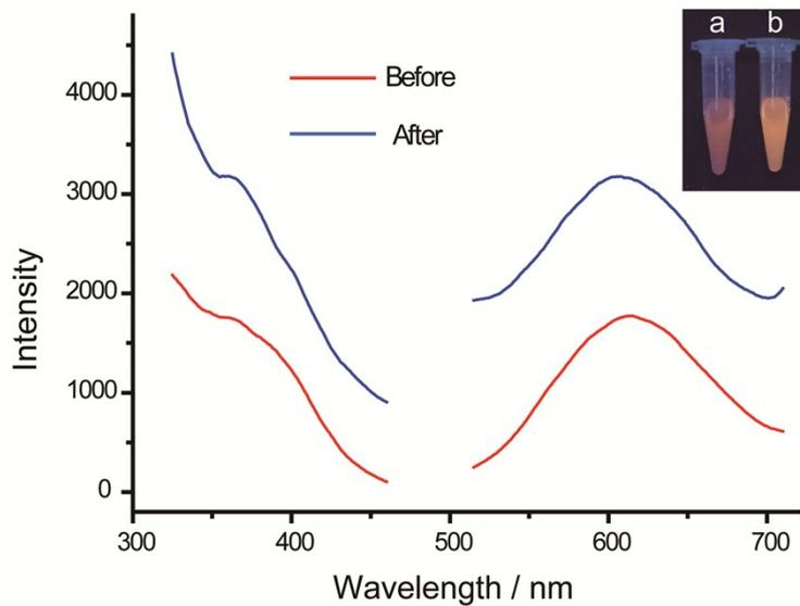
Fig. S1 Fluorescence excitation and emission spectra of glutathione stabilized Au-NCs before (red curves) and after (blue curves) the addition of Pb<sup>2+</sup>. Inset: digital photographs of Au-NCs in the absence (a) and presence (b) of Pb<sup>2+</sup> under 365 nm UV light.
