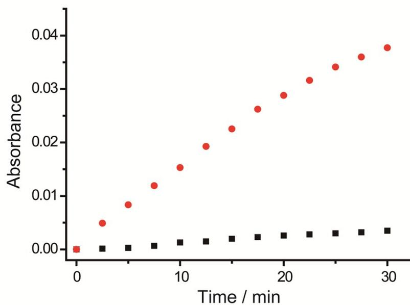
Fig. S10 Reaction kinetics of TMB-H<sub>2</sub>O<sub>2</sub> system in the presence of Au(I)-thiolate complexes (■), and Au(I)-thiolate complexes with Pb<sup>2+</sup> (●).
