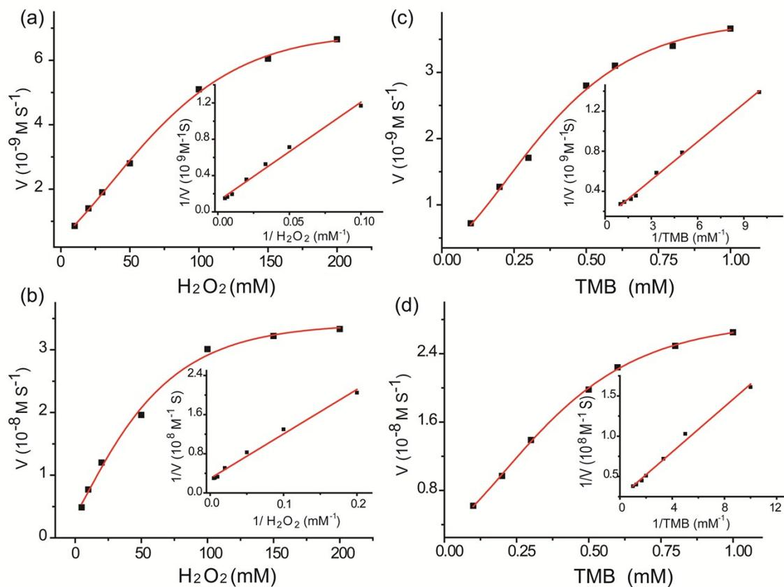
Fig. S4 Steady-state kinetic assays of the Au-NCs in the absence (a, c) and presence (b, d) of  $\text{Pb}^{2+}$ . The kinetic data were obtained by varying one substrate concentrations while keeping the other substrate concentration constant (0.5 mM TMB or 50 mM  $\text{H}_2\text{O}_2$ ). Insets are the Lineweaver-Burk plots of the double reciprocal of the Michaelis-Menten equations.
