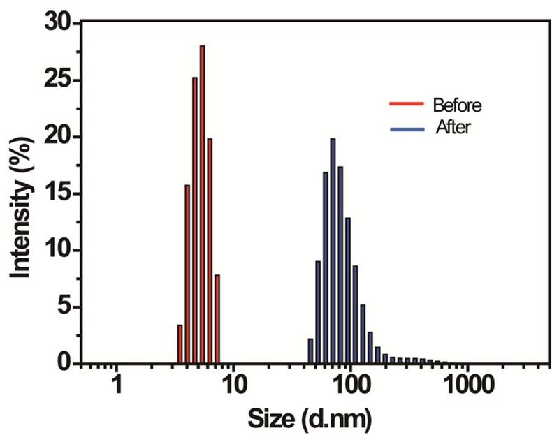
Fig. S6 The hydrodynamic size distribution of Au-NCs before (red) and after (blue) the addition of  $Pb^{2+}$ .
