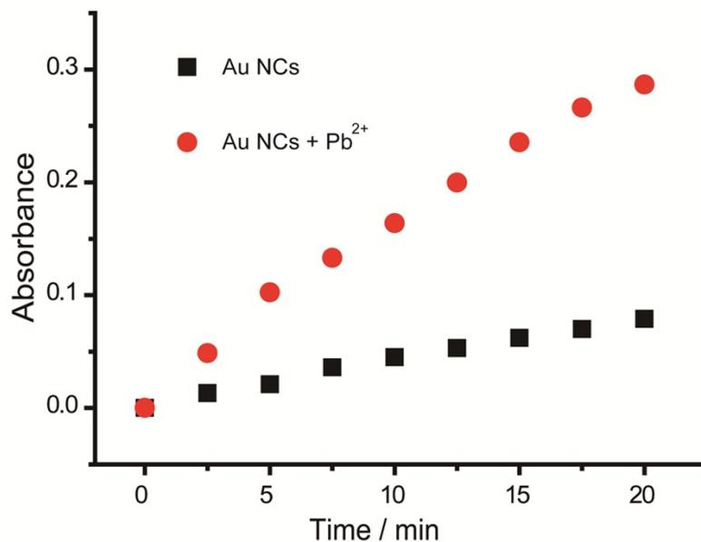
Fig. S9 The kinetic curves of Au-NCs toward ABTS (0.5 mM) oxidation in the presence of H<sub>2</sub>O<sub>2</sub> (10 mM) in the absence (■) and presence (●) of Pb<sup>2+</sup> (0.2 mM).
