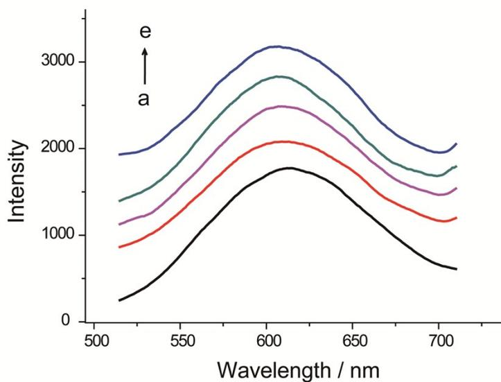
Fig. S2 Fluorescence emission spectra of Au-NCs in the presence of different concentrations of Pb<sup>2+</sup> (from a to e: 0 μM, 50 μM, 100 μM, 200 μM, 300 μM)
