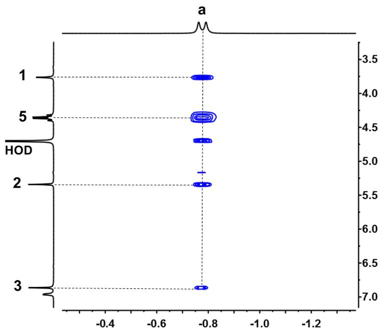
**Fig. S16** 2D ROESY spectrum (500 MHz, 298K, D<sub>2</sub>O) of the complex based on **H3** and **P1** (25.00 mM for each).
