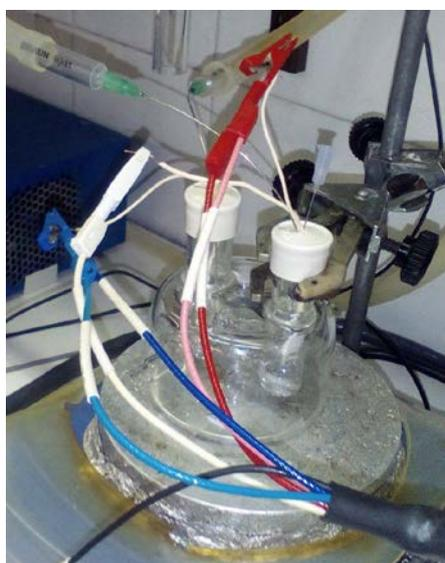
**Fig. S11** Picture of the CPE cell and the Ru/MeOH/THF nanomaterial deposited onto ITO electrode.
