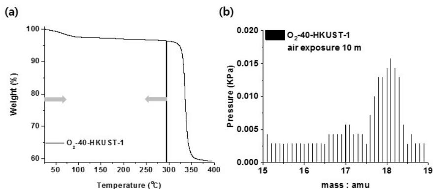
**Figure S17.** (a) TGA thermograph of O<sub>2</sub>-40-HKUST-1 after air exposure for 10 min. (b) The TGA-MS data. The displayed MS histogram was recorded during the temperature increment from RT to 280 °C.
