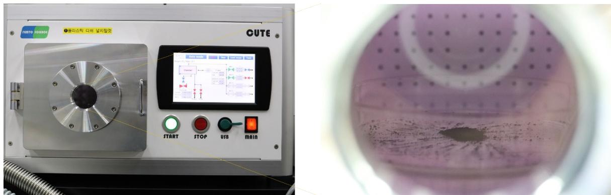
**Figure S1.** Experimental setup for O<sub>2</sub> plasma treatment. O<sub>2</sub> plasma exposure condition: Pressure (0.7-0.8 torr) and power (100 W).
