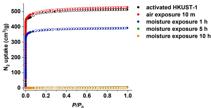
**Figure S4.**  $N_2$  adsorption and desorption isotherms of activated HKUST-1 (black) and  $O_2$ -10-HKUST-1 upon air exposure for 10 min (red dots) and moisture exposure for 1 h (blue dots), 5 h (green dots), and 10 h (orange dots).
