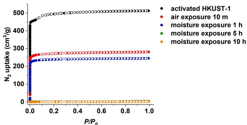
Figure S3. N<sub>2</sub> adsorption and desorption isotherms of activated HKUST-1 (black) and O<sub>2</sub>-0-HKUST-1 upon air exposure for 10 min (red dots) and moisture exposure for 1 h (blue dots), 5 h (green dots), and 10 h (orange dots).
