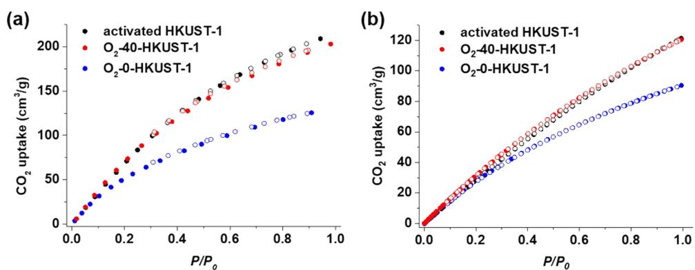
**Figure S13.** CO<sub>2</sub> adsorption and desorption isotherms of activated HKUST-1 (black dots), O<sub>2</sub>-0-HKUST-1 (blue) and O<sub>2</sub>-40-HKUST-1 (red). (a) 273 K and (b) 298 K.
