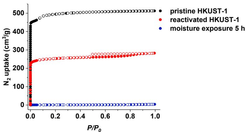
**Figure S12.** N<sub>2</sub> adsorption and desorption isotherms of pristine HKUST-1 (black dots), HKUST-1 after exposure to moisture for 5 h (blue dots), and reactivated HKUST-1 (red dots).
