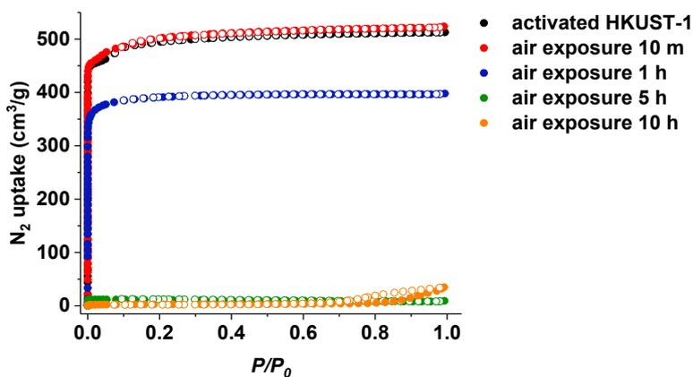
**Figure S8.** N<sub>2</sub> adsorption and desorption isotherms of activated HKUST-1 (black) and O<sub>2</sub>-40-HKUST-1 upon air exposure for 10 min (red dots), 1 h (blue dots), 5 h (green dots), and 10 h (orange dots).
