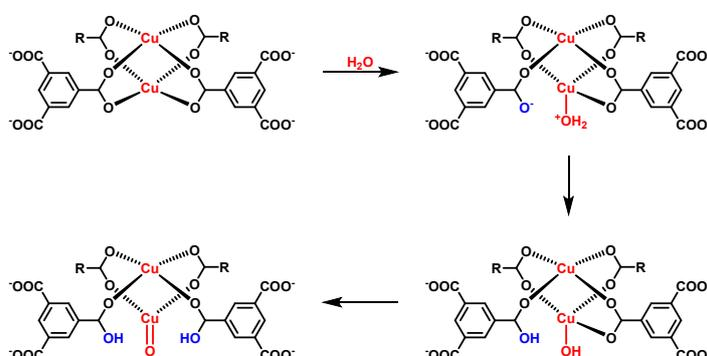
**Figure S21.** Proposed mechanism of the hydrolysis of Cu<sub>2</sub>-unit in HKUST-1. (US 8633331 B2, nanocomposite materials comprising metal-organic-framework units and methods of using same)
