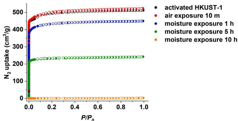
**Figure S5.**  $N_2$  adsorption and desorption isotherms of activated HKUST-1 (black) and  $O_2$ -40-HKUST-1 upon air exposure for 10 min (red dots) and moisture exposure for 1 h (blue dots), 5 h (green dots), and 10 h (orange dots).
