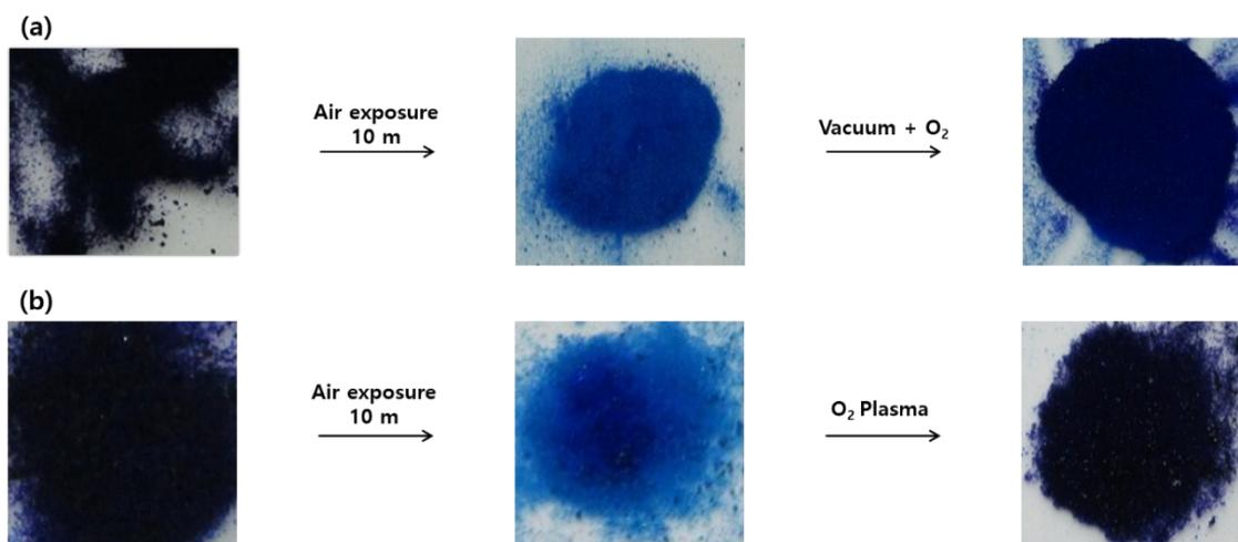
**Figure S20.** (a) Color change of activated HKUST-1 (left) upon air exposure (middle) and then O<sub>2</sub> blowing under 0.701 torr (right). (b) Color change of activated HKUST-1 (left) upon air exposure for 10 min (middle) and then O<sub>2</sub> Plasma treatment for 40 min (right).
