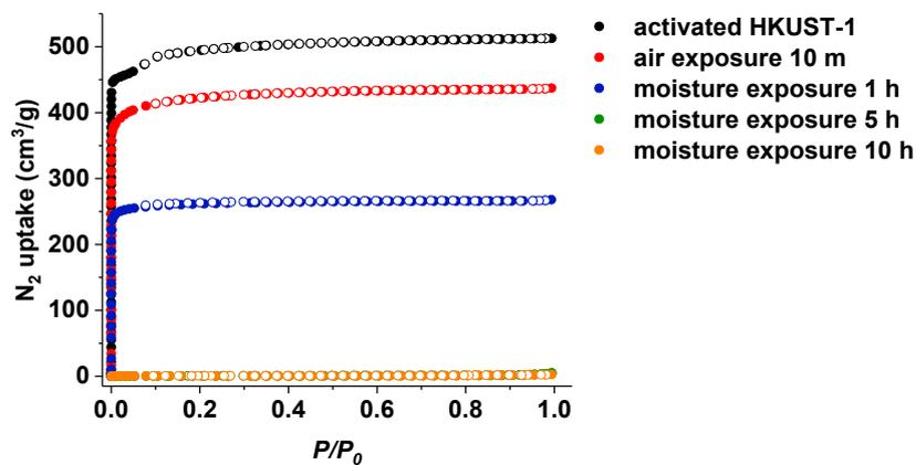
**Figure S6.**  $N_2$  adsorption and desorption isotherms of activated HKUST-1 (black) and  $O_2$ -60-HKUST-1 upon air exposure for 10 min (red dots) and moisture exposure for 1 h (blue dots), 5 h (green dots), and 10 h (orange dots).
