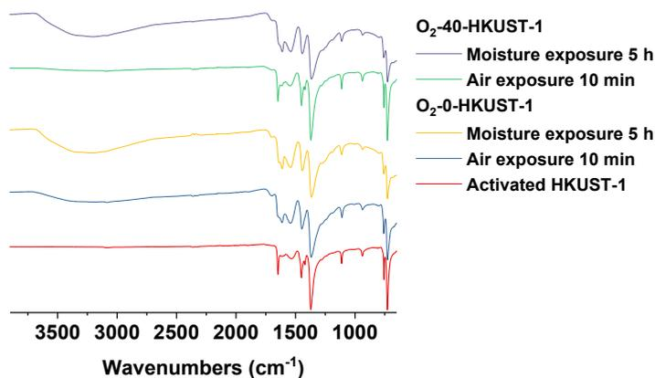
**Figure S15.** IR spectrum of activated HKUST-1 (red), O<sub>2</sub>-0-HKUST-1 upon air exposure for 10 min (blue) and moisture exposure for 5 h (yellow), and O<sub>2</sub>-40-HKUST-1 upon air exposure for 10 min (green) and moisture exposure for 5 h (navy).
