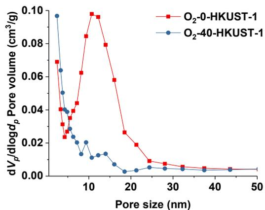
**Figure S11.** Meso-pore size distribution (BJH plot) of reactivated O<sub>2</sub>-0-HKUST-1 (red) and O<sub>2</sub>-40-HKUST-1 (blue) after moisture exposure for 5 h. the samples were reactivated at 100 °C under vacuum for 24 h.
