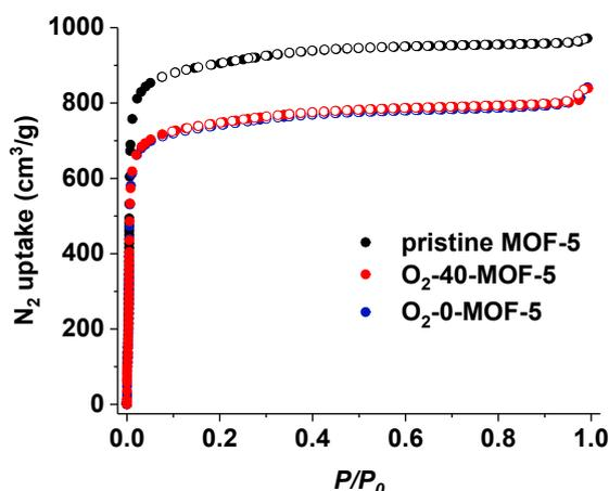
**Figure S22.** N<sub>2</sub> adsorption and desorption isotherms of pristine MOF-5 (black dots), and O<sub>2</sub>-0-MOF-5 (blue dots) and O<sub>2</sub>-40-MOF-5 (red dots) after air exposure 10 min.
