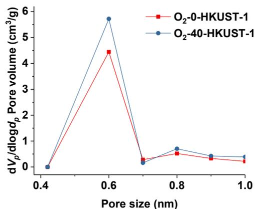
**Figure S10.** Micro-pore size distribution (MP plot) of reactivated O<sub>2</sub>-0-HKUST-1 (red) and O<sub>2</sub>-40-HKUST-1 (blue) after moisture exposure for 5 h. the samples were reactivated at 100 °C under vacuum for 24 h.
