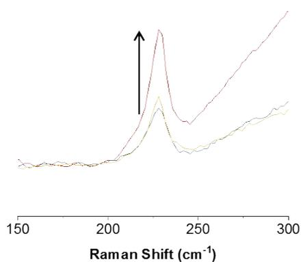
**Figure S19.** Raman spectra of O<sub>2</sub>-0-HKUST-1 (moisture exposure for 5 h). The peak intensity at 229 cm<sup>-1</sup> was restored after exposure of laser light (532 nm). Raman spectroscopy was performed under inert conditions to prevent the coordination of additional water molecules during the acquisitions of the spectra. The sample was exposed to the 532-nm laser light at 10% of its nominal power (25 mW). Regeneration took place after 32 scans, where one scan requires 5 s.
