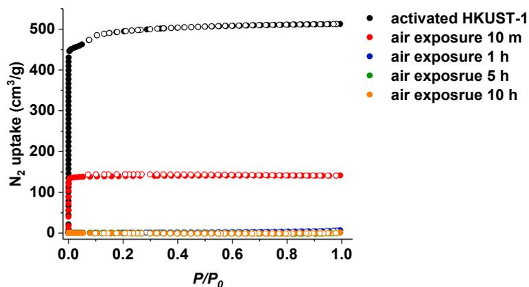
**Figure S7.** N<sub>2</sub> adsorption and desorption isotherms of activated HKUST-1 (black) and O<sub>2</sub>-0-HKUST-1 upon air exposure for 10 min (red dots), 1 h (blue dots), 5 h (green dots), and 10 h (orange dots).
