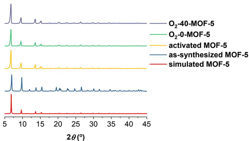
**Figure S23.** PXRD patterns of simulated MOF-5 (red), as-synthesized MOF-5 (blue), activated MOF-5 (yellow), and O<sub>2</sub>-0-MOF-5 (green) and O<sub>2</sub>-40-MOF-5 (purple) after air exposure 10 min.
