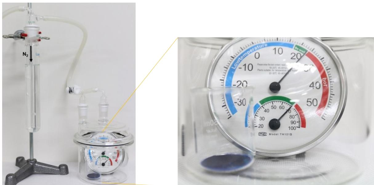
**Figure S2.** Experimental setup for 70% humidity exposure.
