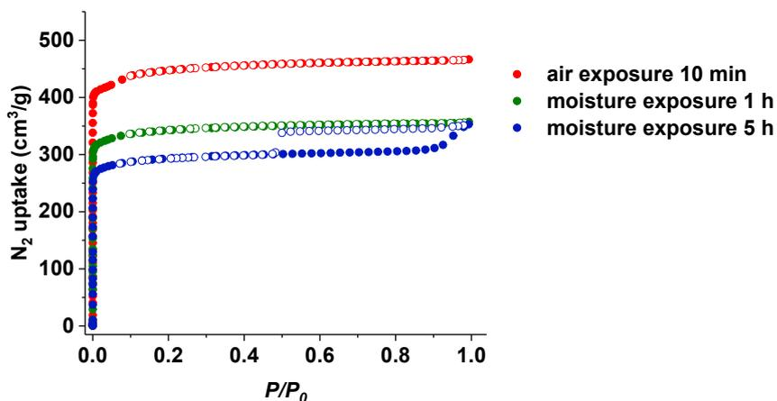
**Figure S9.** N<sub>2</sub> adsorption and desorption isotherms of O<sub>2</sub>-60-HKUST-1 after reactivation process at 100 °C for 24 h. Red, green, and blue dots are for 10 min air exposed and 1 h and 5 h moisture exposed samples, respectively.
