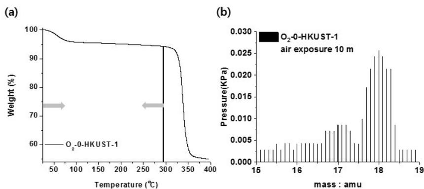
**Figure S16.** (a) TGA thermograph of O<sub>2</sub>-0-HKUST-1 after air exposure for 10 min. (b) The TGA-MS data. The displayed MS histogram was recorded during the temperature increment from RT to 280 °C.
