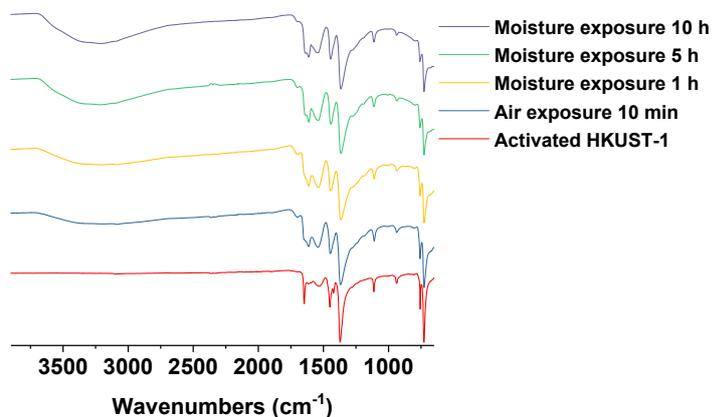
**Figure S14.** IR spectrum of activated HKUST-1 (red) and O<sub>2</sub>-0-HKUST-1 upon air exposure for 10 min (blue) and moisture exposure for 1 h (yellow), 5 h (green), and 10 h (navy).
