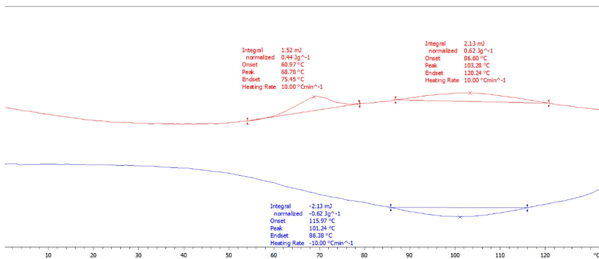
**Figure S5.** DSC thermograms obtained for **7a** on heating and cooling cycles at a scan rate of 10°C/min.
