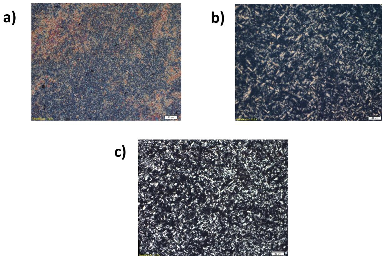
**Figure S4.** Birefringence texture observed under POM: a) compound **7b** at room temperature and b) compound **7b** mosaic texture observed on cooling from the isotropic phase at 103 °C. c) compound **7c**, mosaic texture observed on cooling from the isotropic phase at 60 °C.
