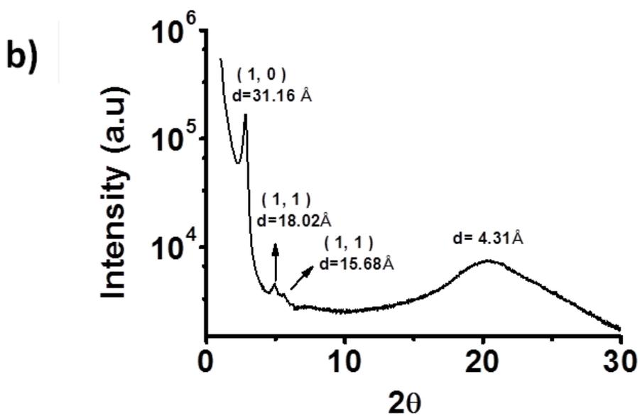
**Figure S2.** The one-dimensional intensity versus  $2\theta$  profile derived from X-ray diffraction. **a)** **7a** at room temperature, **b)** **7b** at room temperature **c)** **7b** at 80 °C.
