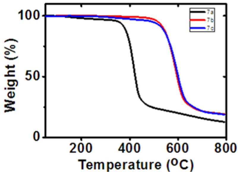
**Figure S3.** TGA spectra of **7a**, **7b** and **7c** which show excellent thermal stability of the three compounds.
