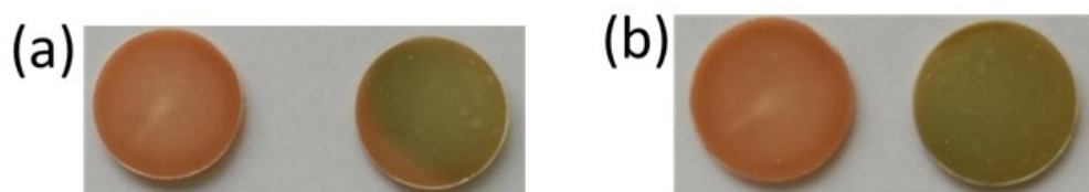
Figure S6. The photographs of Zn-BTDC-M1 before and after irradiation. ((a): before and after under irradiation in 5 min; (b): before and after under irradiation in 25 min).
