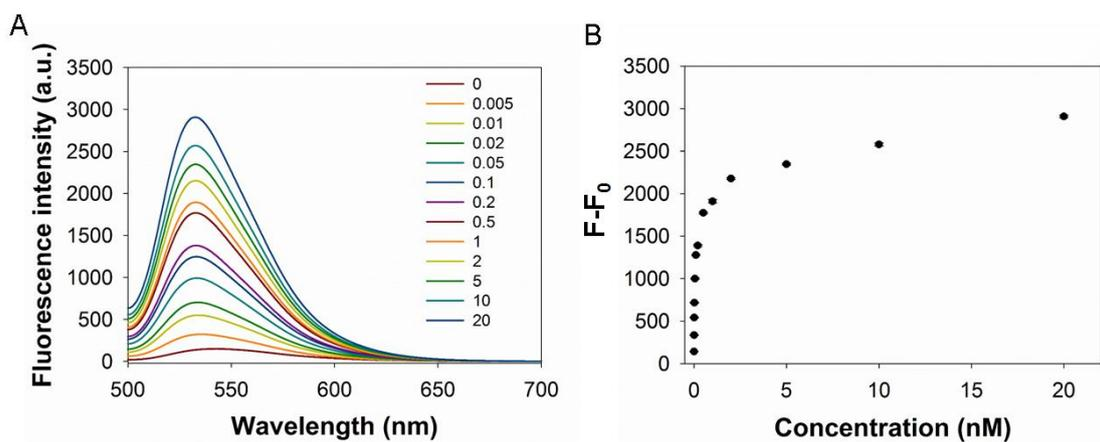
**Figure S7.** Fluorescence measurements of the SYBR Green I-stained PCR products prepared with different concentrations of split apt-a. (A) Fluorescence spectra recorded at various concentrations of split apt-a (nM). (B) Corresponding calibration curve illustrating the relationship between the detected fluorescence signal increase ( $F - F_0$ ) and the concentration of split apt-a. (Error bars: standard deviations from three repeated experiments.)
