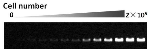
**Figure S8.** Characterization of the PCR products from SMMC-7721 cell samples with different cell numbers treated by split apt-a/split apt-b, using 3% agarose gel electrophoresis.
