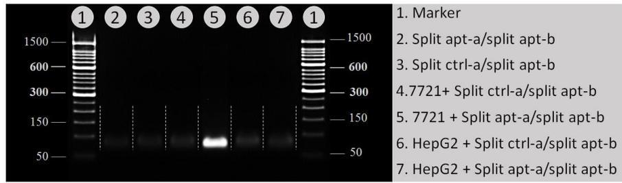
**Figure S6.** Characterization of the PCR products via different samples using 3% agarose gel electrophoresis, showing feasibility of the thermosensitive split apta-PCR strategy for detecting target SMMC-7721 cells.
