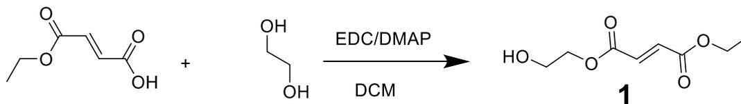
**Scheme S2.** Synthesis of 2-hydroxyethyl-ethyl fumarate for **BB** synthesis.
