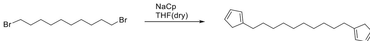
**Scheme S1.** Synthesis of 1,10-di(cyclopentadienyl)-decane monomer **AA**.
