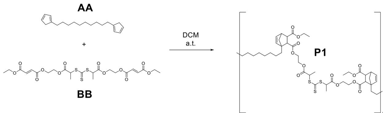
**Scheme S7.** Step-growth polymerization by Diels-Alder reaction using monomer **AA** and **BB** in DCM at ambient temperature.
