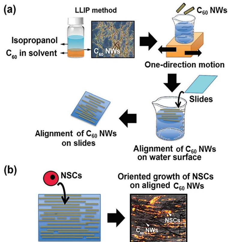
**Figure S4.** Schematic illustration for the preparation of highly aligned C<sub>60</sub> NWs and growing neural stem cells (NSCs) on the NW scaffolds. (a) The alignment of C<sub>60</sub> NWs was obtained at an air–water interface by the
