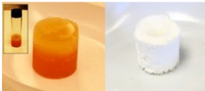
Figure S1. Photos of (left) PU-IL resin gel and (right) IL-free PU-control gel prior to removal of solvent in vacuo; (inset) photo of PU-IL resin after polymerization at room temperature; vial outer diameter is 15 mm.
