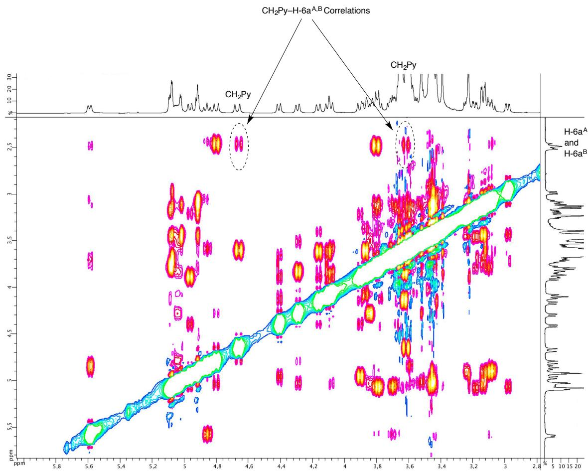
Part of the  $^1\text{H}$ - $^1\text{H}$  ROESY NMR spectrum of **13** showing cross-peaks (circled) arising from through-space correlations between  $\text{CH}_2\text{Py}$  protons and H-6 protons of the AB bridged glucose units
