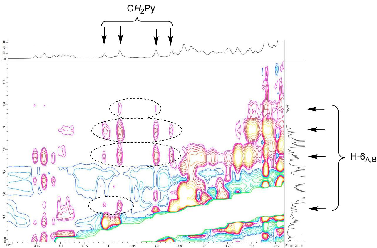
Part of the ROESY spectrum of **11a** showing cross-peaks (circled) for H-6<sub>A,B</sub>-CH<sub>2</sub>Py interactions
