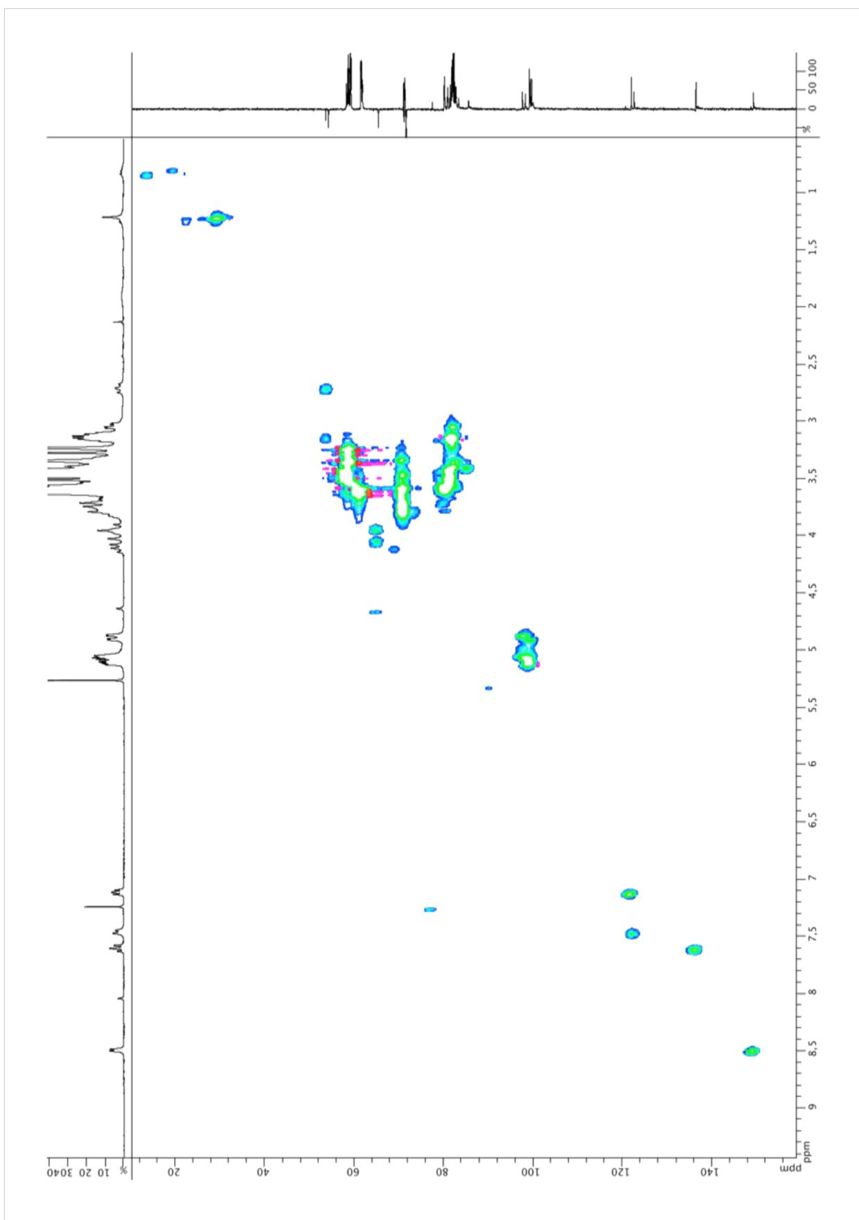
$^1\text{H}$ - $^{13}\text{C}$  HSQC NMR spectrum of **12a/b**
