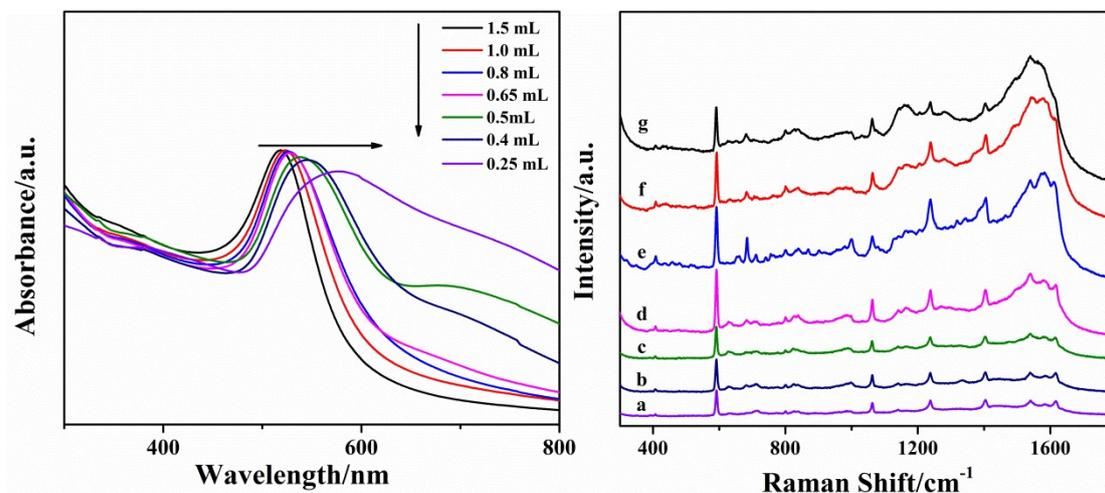
Figure S5 (A) UV-Vis spectra of Au NPs prepared with the solution of sodium citrate (0.1%, w/v) with different volumes; (B) Raman spectra of  $10^{-5}$  M PYR obtained by using the AuNPs/SNW-1 as substrate fabricated with Au NPs prepared with the solution of sodium citrate (0.1%, w/v) with different volumes (a-g: 0.25, 0.4, 0.5, 0.65, 0.8, 1.0 and 1.5 mL).
