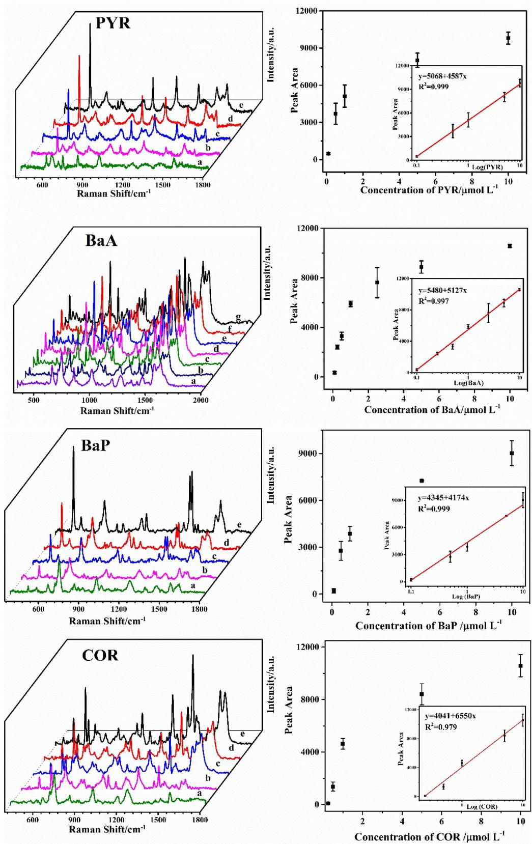
Figure S7 Left: Raman spectra by using the AuNPs/SNW-1 as the SERS substrate obtained from: AcPy of 1.0, 2.5, 5.0, 10, and 25.0 μM (a-e); ANT of 0.25, 0.5, 1.0, 2.5, 5.0 and 10.0 μM (a-f); PHE of 0.5, 1.0, 2.5, 5.0 and 10.0 μM (a-e); PYR of 0.1, 0.5, 1.0, 5.0, 10.0 and 50.0 μM (a-f); BaA of 0.1, 0.25, 0.5, 1.0, 2.5, 5.0 and 10.0 μM (a-g); BaP of 0.1, 0.5, 1.0, 5.0 and 10.0 μM (a-e); COR of 0.25, 0.5, 1.0, 5.0 and 10.0 μM (a-e). Right: scatter plots of peak area
