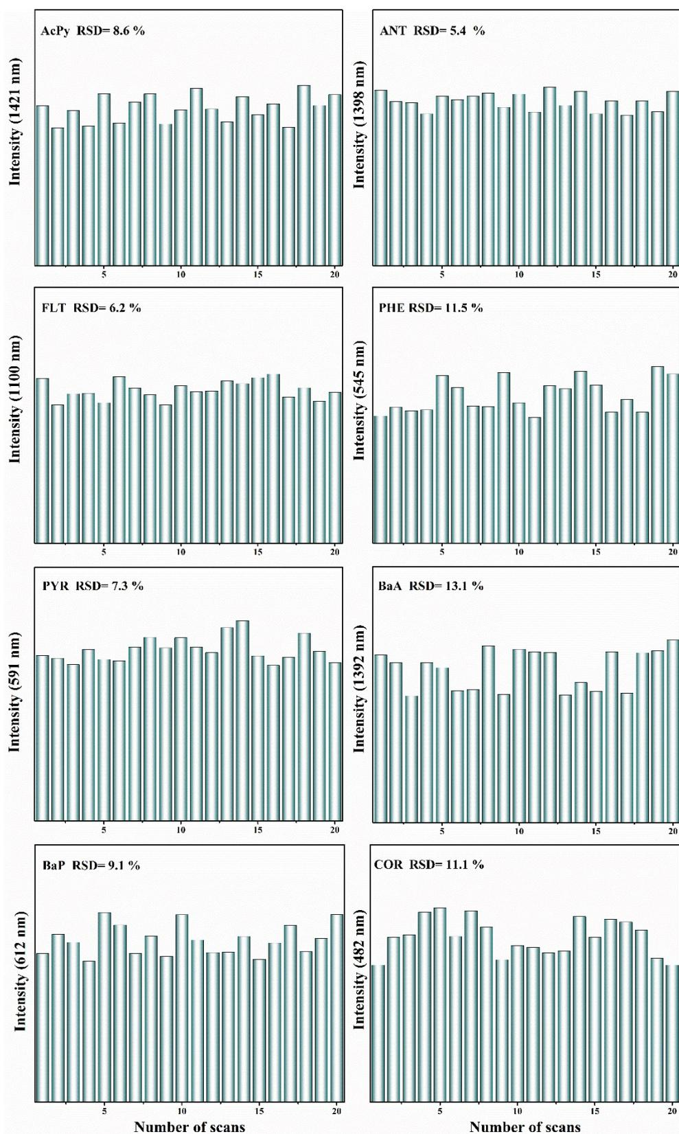
Figure S8 The intensity of one characteristic Raman peak (for demonstration) of each PAHs collected from 20 randomly selected spots on the same AuNPs/SNW-1 substrate (inset: calculated relative standard deviation of the intensity).
