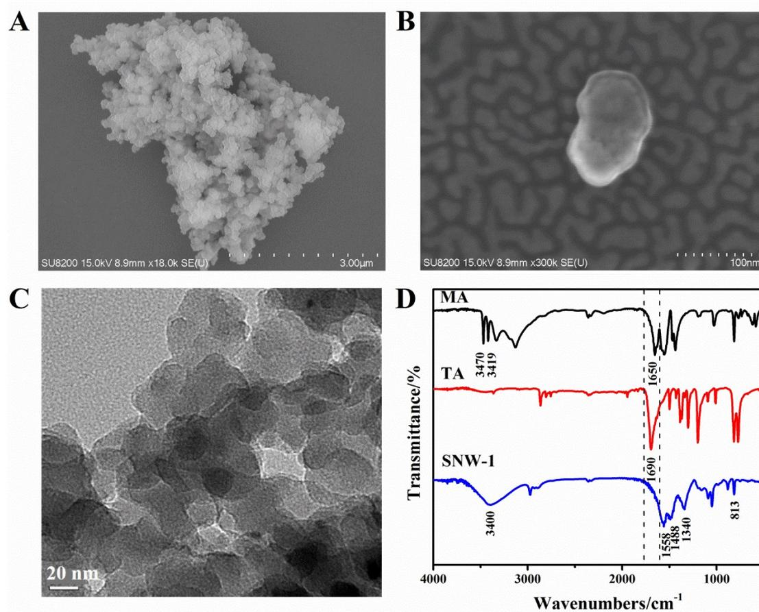
Figure S1 SEM (A&B) and TEM (C) image of SNW-1 NPs; (D) FT-IR spectra of MA, TA and SNW-1.
