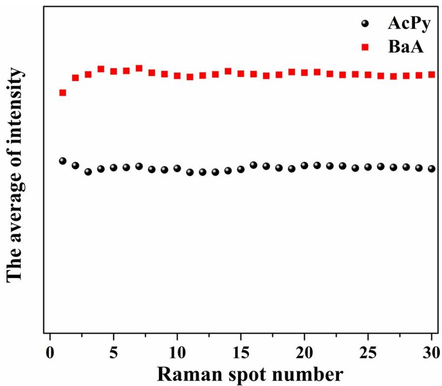
Figure S9 Averaged intensity of Raman signals obtained from randomly selected spots on the same substrate of AuNPs/SNW-1.
