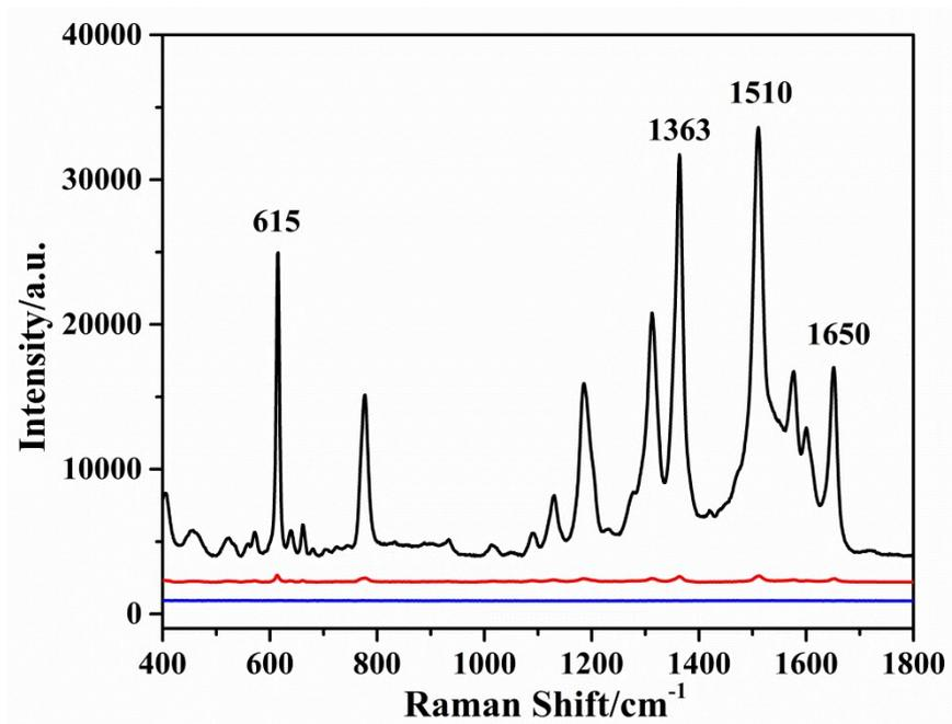
Figure S3. Raman spectra of R6G ( $10^{-5}$  M) obtained by using SNW-1 (blue), Au NPs (red) and AuNPs/SNW-1 (black) as SERS substrate, respectively.
