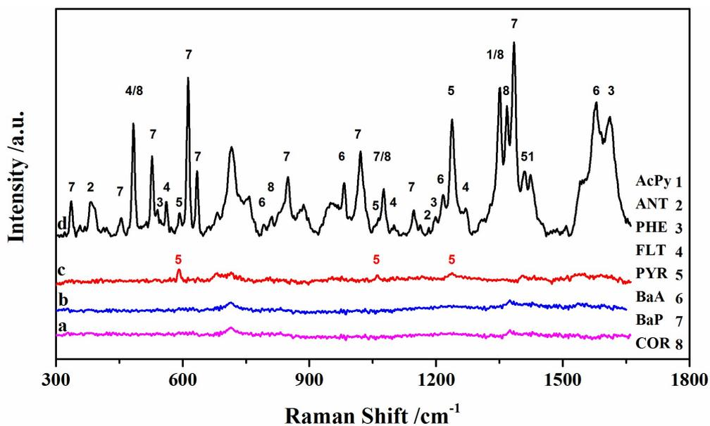
Figure S10 Raman spectra by using the AuNPs/SNW-1 as the SERS substrate obtained from blank (a), tap water sample (b), pond water sample (c) and mixture of the eight PAHs with each PAHs at a concentration of  $5 \times 10^{-6}$  M.
