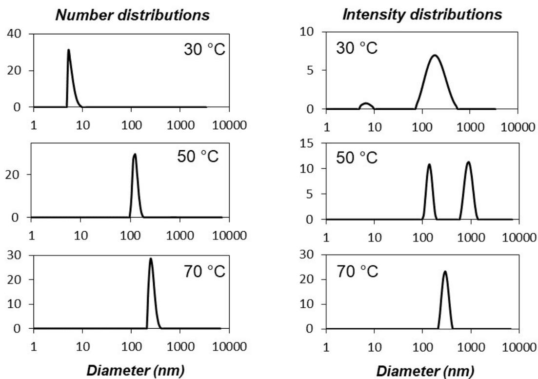
**Figure S8.** DLS measurements of aqueous solution of the block copolymer P7 at a concentration of 10 mg mL<sup>-1</sup>.
