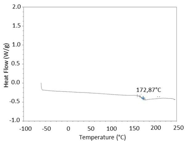
**Figure S4.** DSC traces of alternating poly(peptide-*alt*-peptoid) copolymers **P<sub>1-3</sub>**.
