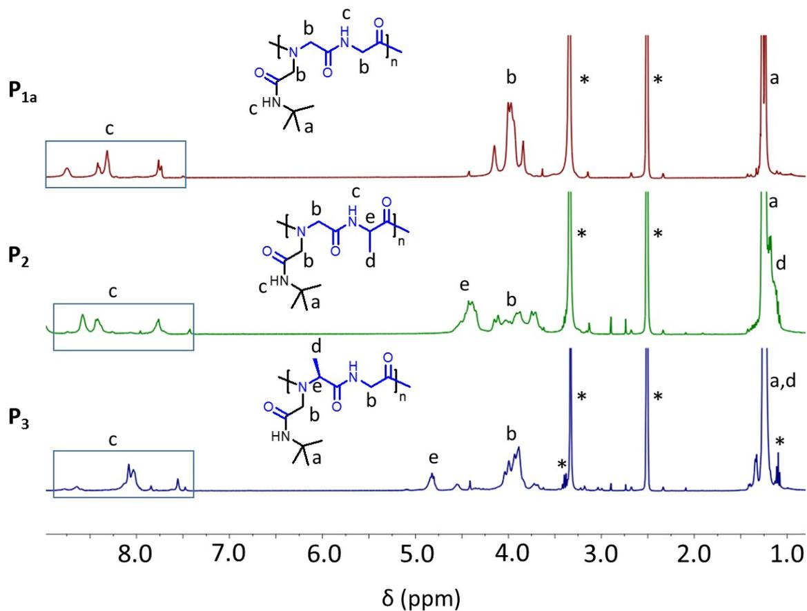
**Figure S1.**  $^1\text{H}$  NMR spectra of alternating poly(peptide-*alt*-peptoid) copolymers  $\text{P}_{1-3}$  in  $\text{DMSO-d}_6$ . \*corresponds to residual pics of water (3.3 ppm),  $\text{DMSO}$  (2.5 ppm) and  $\text{Et}_2\text{O}$  (3.4 and 1.1 ppm) .
