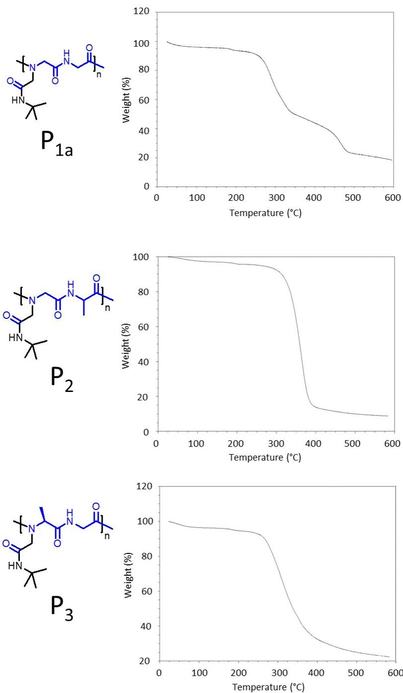
**Figure S3.** Thermogravimetric analysis of alternating poly(peptide-*alt*-peptoid) copolymers **P<sub>1-3</sub>**.
