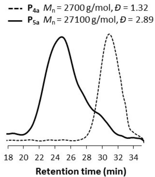
**Figure S6.** SEC chromatograms for the synthesis of the poly[DMA-graft-(peptoid-alt-peptide)]copolymer P5.
