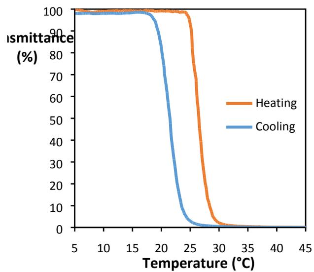
**Figure S7.** Turbidimetry measurements of aqueous solution of  $P_1$  at a concentration of 2 mg/mL (heating and cooling rate = 2 °C/min). The cloud point temperature measured upon heating is equal to 27 °C (temperature corresponding to 50 % loss of transmittance).
