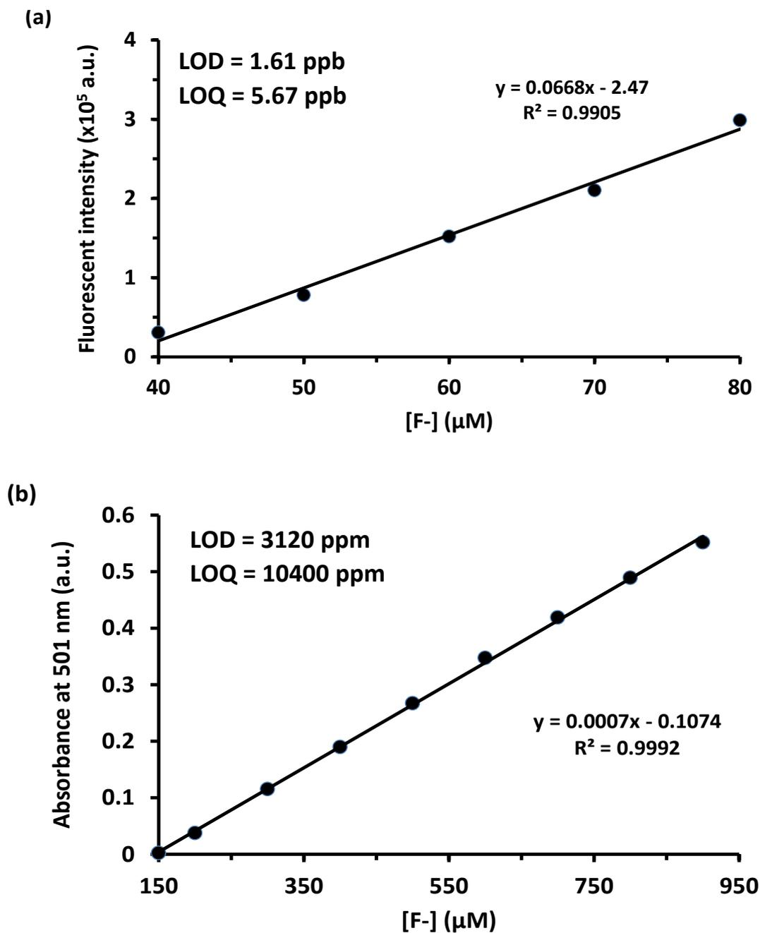
**Figure. S10** The calibration curve (a) from fluorescence data of PySQ at 5.6  $\mu\text{M}$  in DMSO at excitation wavelength 351 nm and emission wavelength 395 nm, (b) The calibration curve of PySQ from UV-Vis data of PySQ at 56  $\mu\text{M}$  in THF.
