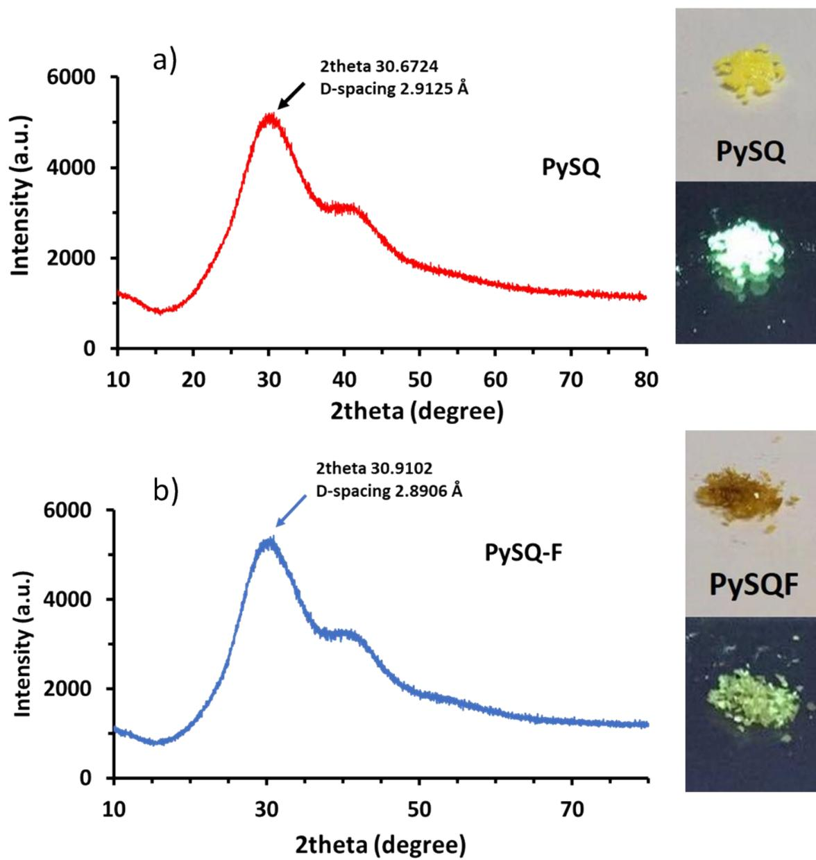
Figure. S19. X-ray Powder Diffraction (XRD) of PySQ and PySQ-F
