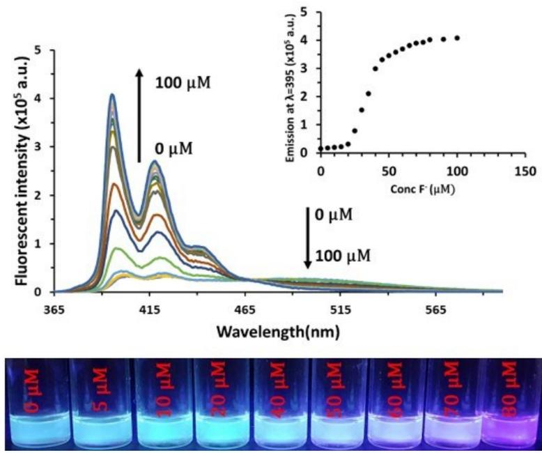
**Figure. S4** The emission spectra of PySQ (5.6  $\mu\text{M}$  in DMSO) upon addition of TBAF with excitation wavelength at 351 nm.
