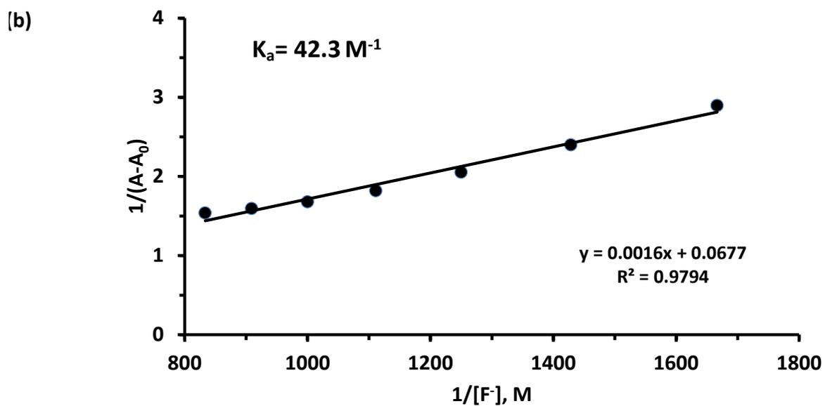
**Figure. S6** Benesi–Hildebrand plot from (a) Fluorescence titration data of PySQ at 5.6  $\mu\text{M}$  in DMSO and (b) from Uv-vis titration data of PySQ at 56  $\mu\text{M}$  in THF
