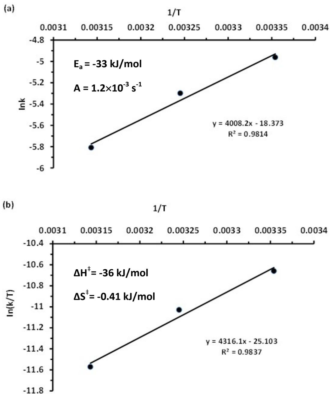
**Figure. S5** (top) Arrhenius plot of PySQ between  $\ln k$  against  $1/T(\text{K})$ , (bottom) Eyring–Polanyi plot of PySQ between  $\ln k/T$  against  $1/T(\text{K})$ .
