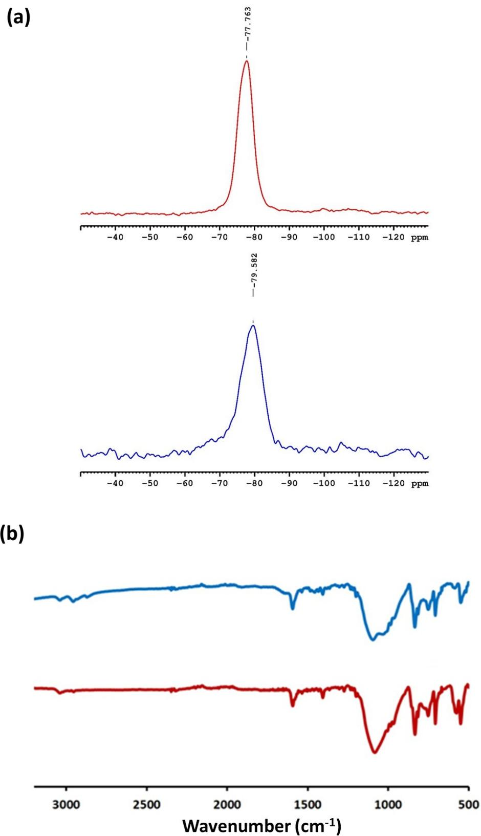
**Figure. S9** (a)  $^{29}\text{Si}$  CP/MAS NMR spectra of PySQ (top) and PySQ-F $^-$  (bottom), (b) IR spectra of PySQ (bottom) and PySQ-F $^-$  (top).
