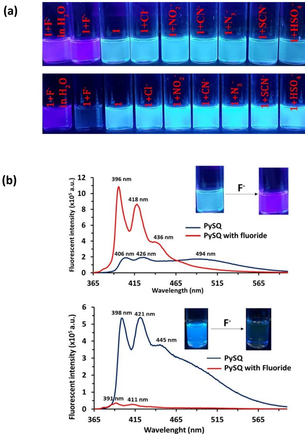
**Figure. S2** (a) Selectivity tests of PySQ in DMSO (top) and in THF (bottom) in different ions at the same concentration (150 eq) under UV-lamp(bottom), (b) The Emission
