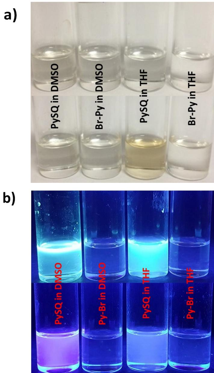
**Figure. S18.** Comparison of PySQ and 1-bromopyrene solutions at the same concentration (56 $\mu$ M), a) (top) before and (bottom) after addition of TBAF (1 eq) under room light; b) (top) before and (bottom) after addition of TBAF (1 eq) under UV lamp.
