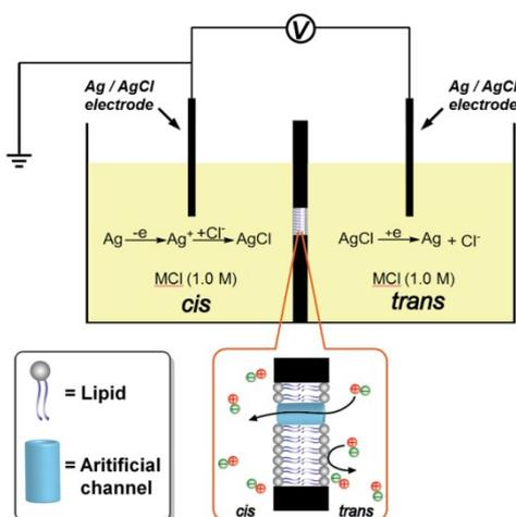
**Fig. S35.** Schematic representation for the patch clamp experiments with planar lipid bilayer. The redox reactions on both Ag/AgCl electrodes are inserted to illustrate the nature of charge balance during M<sup>+</sup> transmembrane transport.
