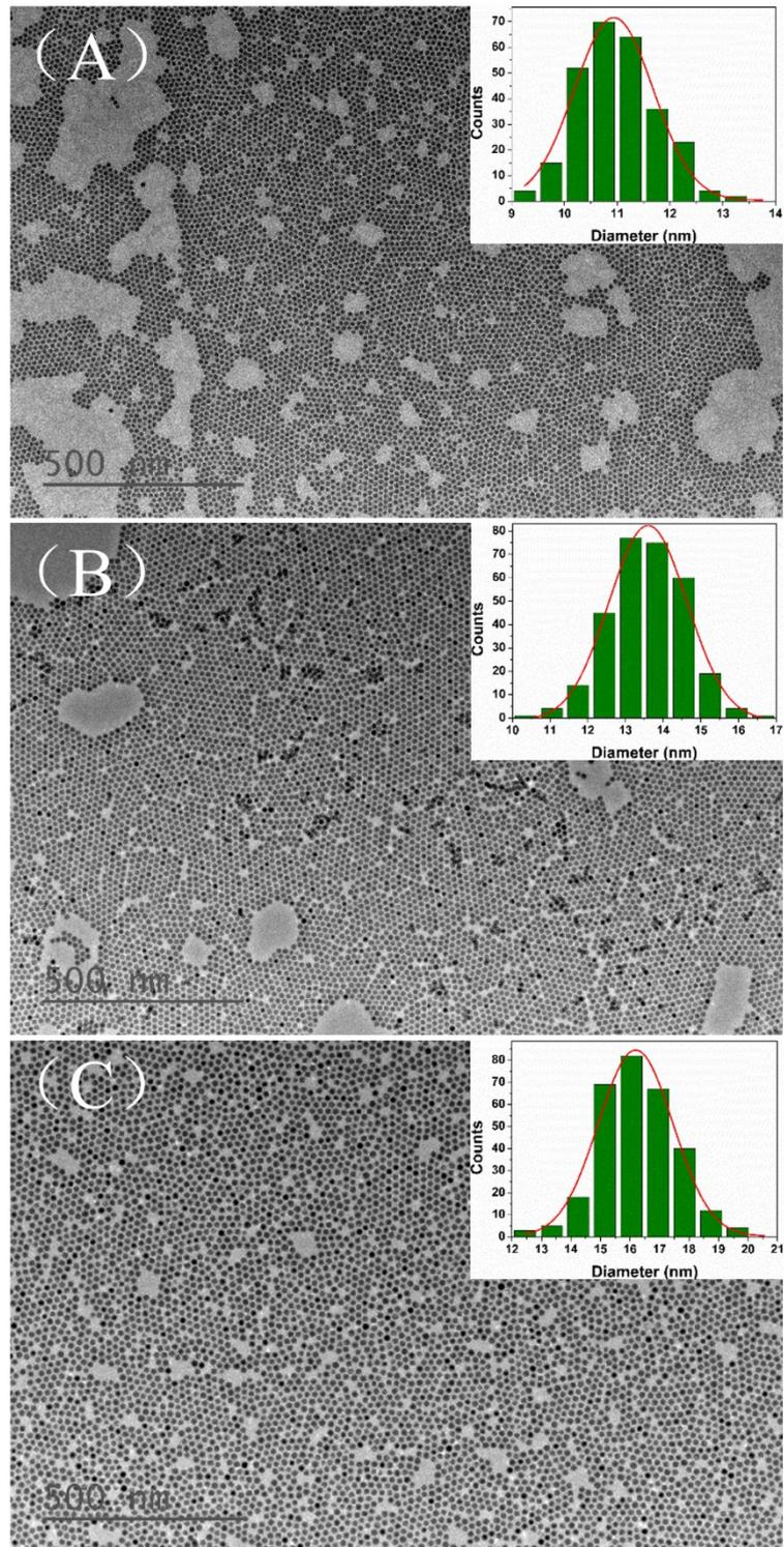
**Fig. S1** TEM images and size statistics for Sn NCs with different diameters.
