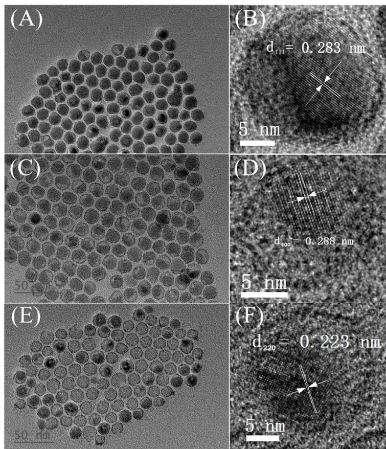
**Fig. S7** (A) TEM and (B) HRTEM images for yolk-shell SnS NCs. (C) TEM and (D) HRTEM images for yolk-shell SnSe NCs. (E) TEM and (F) HRTEM images for yolk-shell SnTe NCs.
