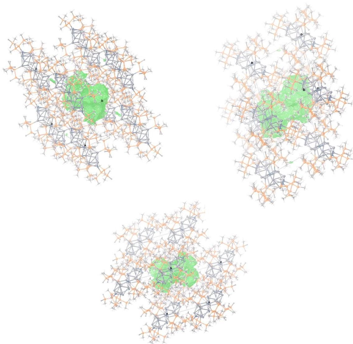
**Figure S1:** Picture of the void (green), localized at -0.121, 0.5, 0.5 within the solid state of  $[\text{Li}(\text{TMEDA})_2][\text{Au}_3\text{Sn}_{18}(\text{Hyp})_8]$  **1**; view from different directions.
