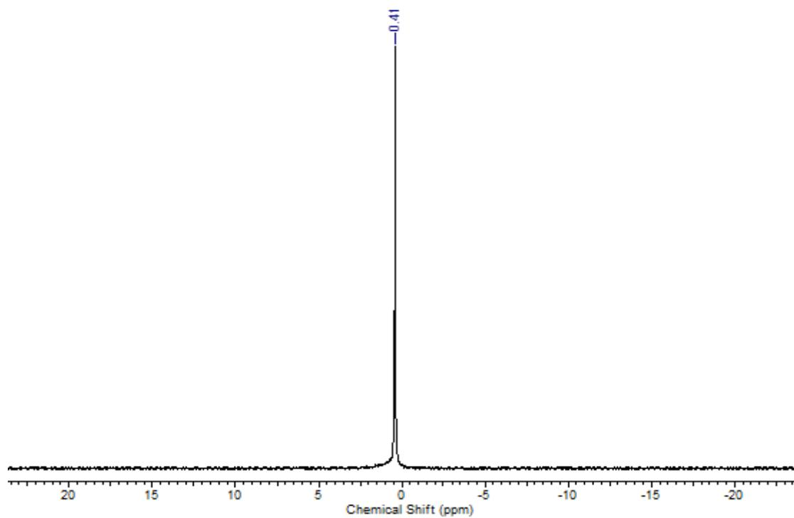
**Figure S5:**  $^7\text{Li}$ -NMR of  $[\text{Li}(\text{TMEDA})_2][\text{Au}_3\text{Sn}_{18}(\text{Hyp})_8]$  **1** dissolved in  $\text{THF-d}_8$  shows a singlet at  $\delta = 0.41$  ppm, which can be seen as prove for the presence of  $[\text{Li}(\text{TMEDA})_2]^+$  in the crystals.
