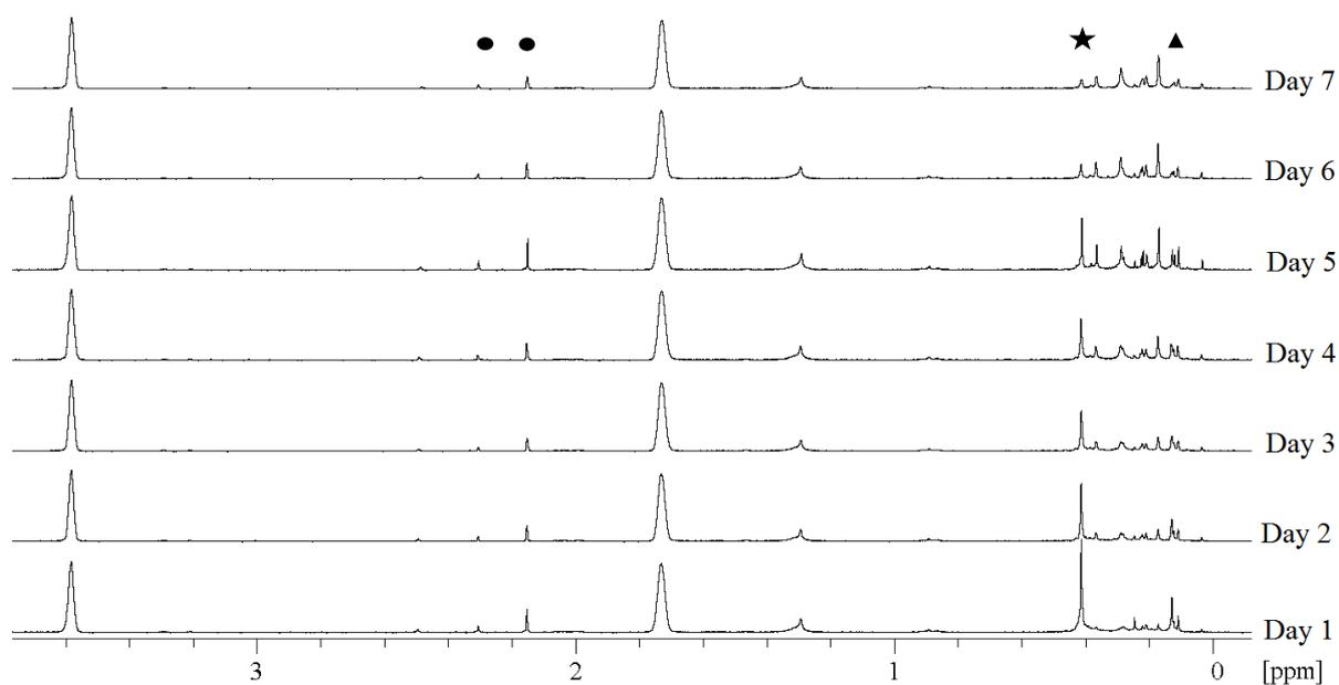
**Figure S3:**  $^1\text{H-NMR}$  of  $[\text{Li}(\text{TMEDA})_2][\text{Au}_3\text{Sn}_{18}(\text{Hyp})_8]$  **1** dissolved in  $\text{THF-d}_8$  shows a fast degradation of **1** within 7 days. The TMEDA signals at  $\delta = 2.15$  ppm and  $\delta = 2.13$  ppm doesn't change during that period, whereas the two Hyp signals at  $\delta = 0.13$  ppm and  $\delta = 0.41$  ppm nearly disappears at day 7.
