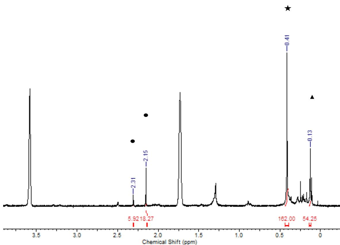
**Figure S2:** <sup>1</sup>H-NMR of [Li(TMEDA)<sub>2</sub>][Au<sub>3</sub>Sn<sub>18</sub>(Hyp)<sub>8</sub>] **1** dissolved in THF-d<sub>8</sub>. The signal at δ = 0.13 ppm shows the Hyp ligand bound to the gold atoms, whereas the signal at δ = 0.41 ppm could be assigned to the Hyp ligand bound to the tin atoms. The integrals shows a ratio of cluster to TMEDA of 1:1.5. ( ● TMEDA, ★ SnHyp, ▲ AuHyp).
