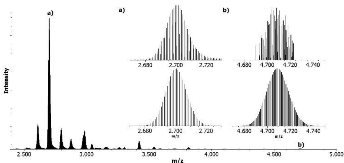
**Figure S6:** Mass spectrum of a solution of  $[\text{Au}_3\text{Sn}_{18}(\text{Hyp})_8]^-$  **1** in THF after electrospray ionization (ESI). Inset measured and calculated isotopic pattern for a)  $[\text{Au}_3\text{Sn}_{18}(\text{Hyp})_8]^-$  **1** and b)  $[\text{Au}_2\text{Sn}_9(\text{Hyp})_5]^-$
