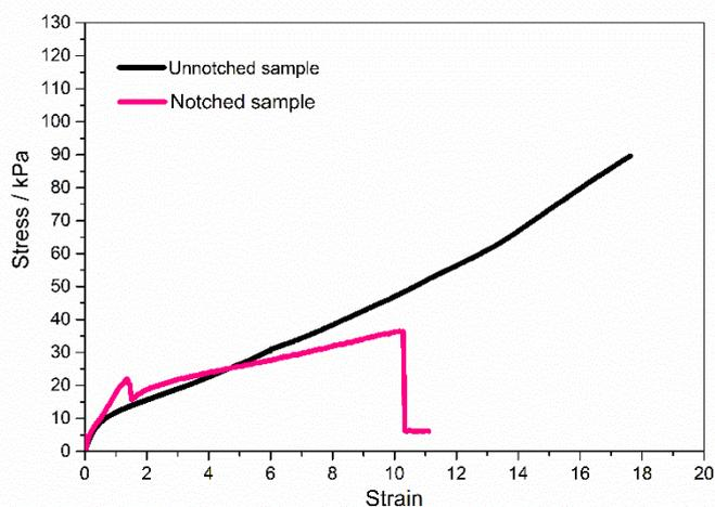
Figure S6. Representative force-extension curve of pure shear test for the unnotched (black) and notched (pink) nDMA/AAPBA-20 hydrogel.
