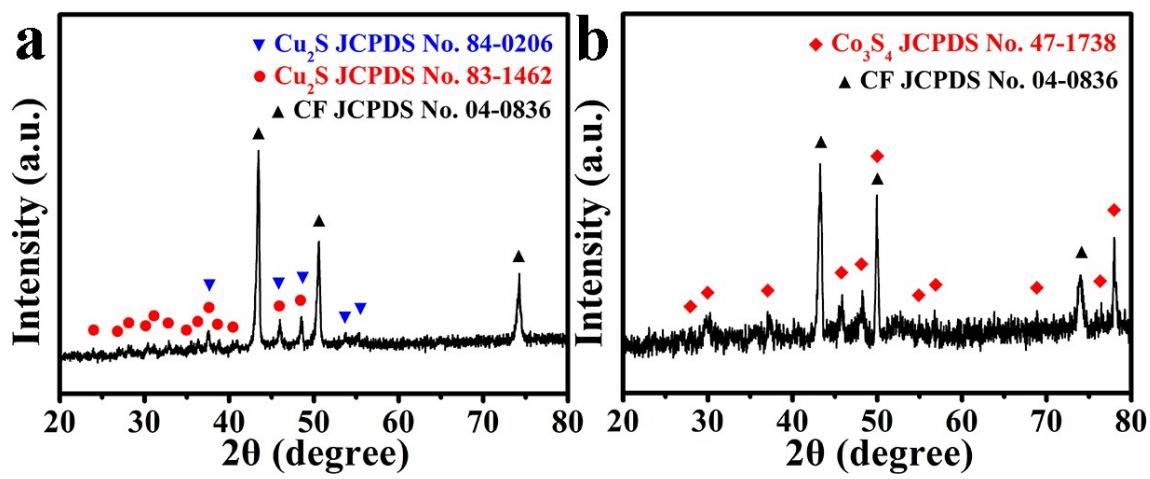
**Fig. S1.** XRD patterns for (a) Cu–S/CF and (b) Co–S/CF.
