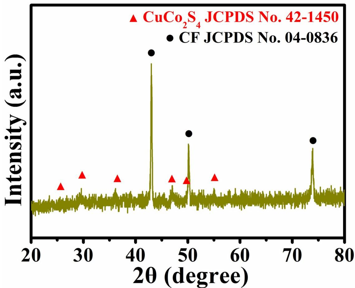
**Fig. S9.** XRD pattern for  $\text{CuCo}_2\text{S}_4/\text{CF}$  after water oxidation electrolysis.
