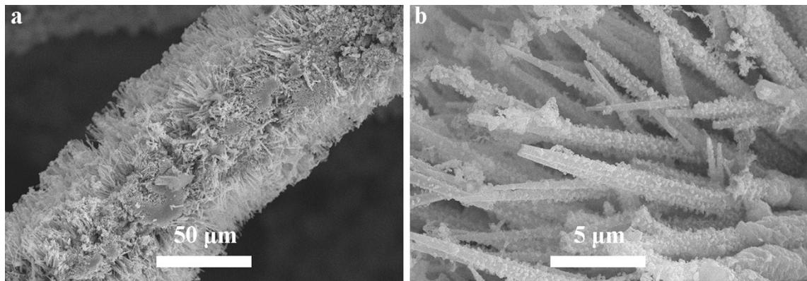
**Fig. S8.** (a) Low- and (b) magnification SEM images for CuCo<sub>2</sub>S<sub>4</sub>/CF after water electrolysis.
