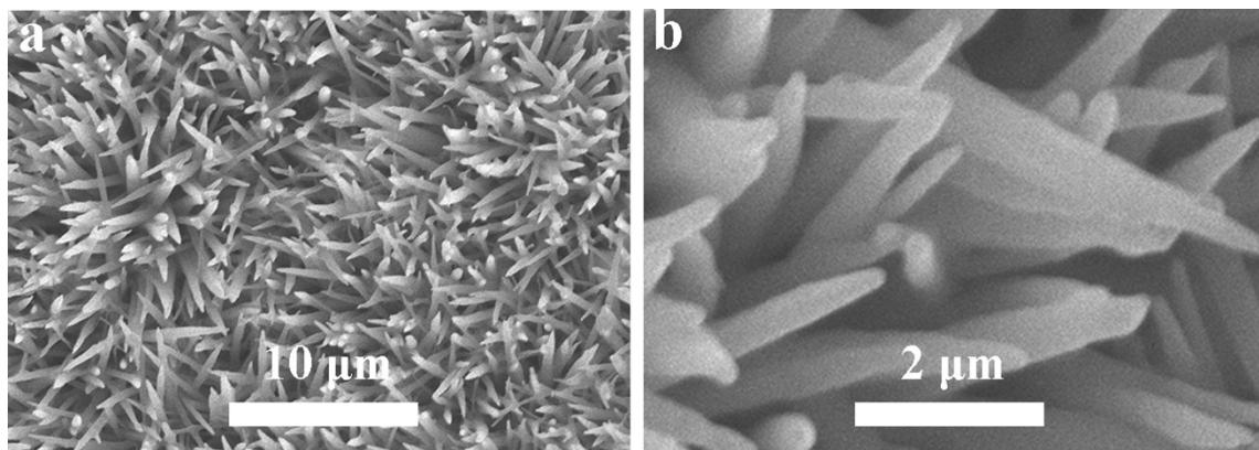
**Fig. S2.** SEM images for CuCo<sub>2</sub>-hydroxide precursor on CF.
