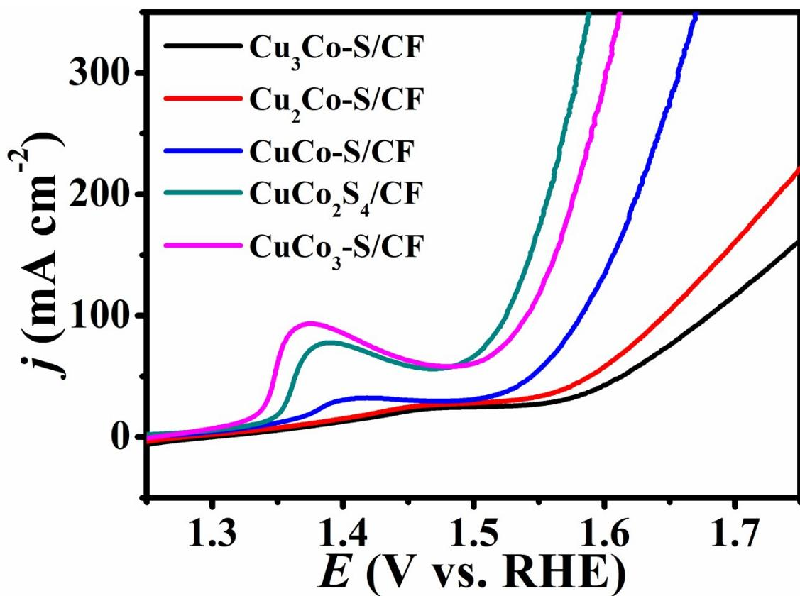
**Fig. S7.** LSV curves of  $\text{Cu}_3\text{Co-S/CF}$ ,  $\text{Cu}_2\text{Co-S/CF}$ ,  $\text{CuCo-S/CF}$ ,  $\text{CuCo}_2\text{S}_4/\text{CF}$ , and  $\text{CuCo}_3\text{-S/CF}$  with a scan rate of  $5 \text{ mV s}^{-1}$  for water oxidation.
