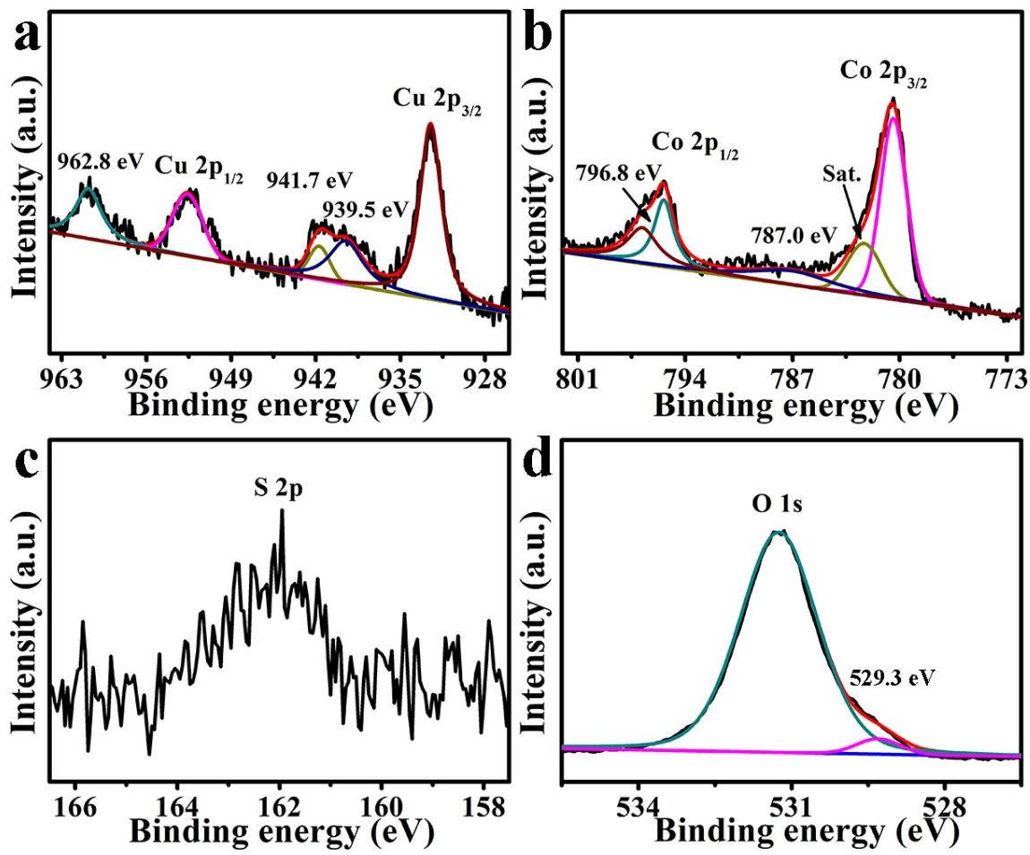
**Fig. S11.** XPS spectra for CuCo<sub>2</sub>S<sub>4</sub> in the (a) Cu 2p, (b) Co 2p, (c) S 2p, and (d) O 1s regions after water oxidation electrolysis.
