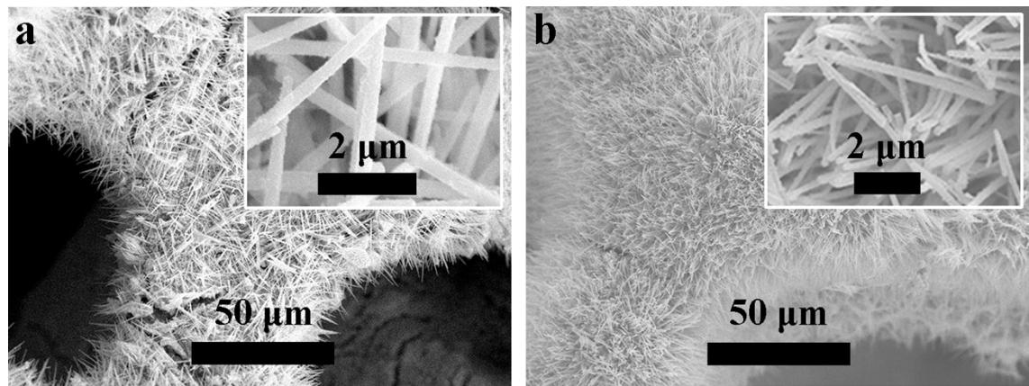
**Fig. S3.** SEM images for (a) Cu–S/CF and (b) Co–S/CF.
