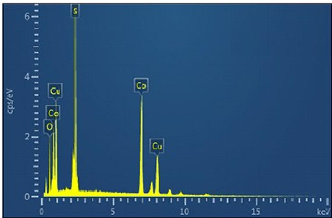
**Fig. S5.** EDX spectrum for  $\text{CuCo}_2\text{S}_4/\text{CF}$ .
