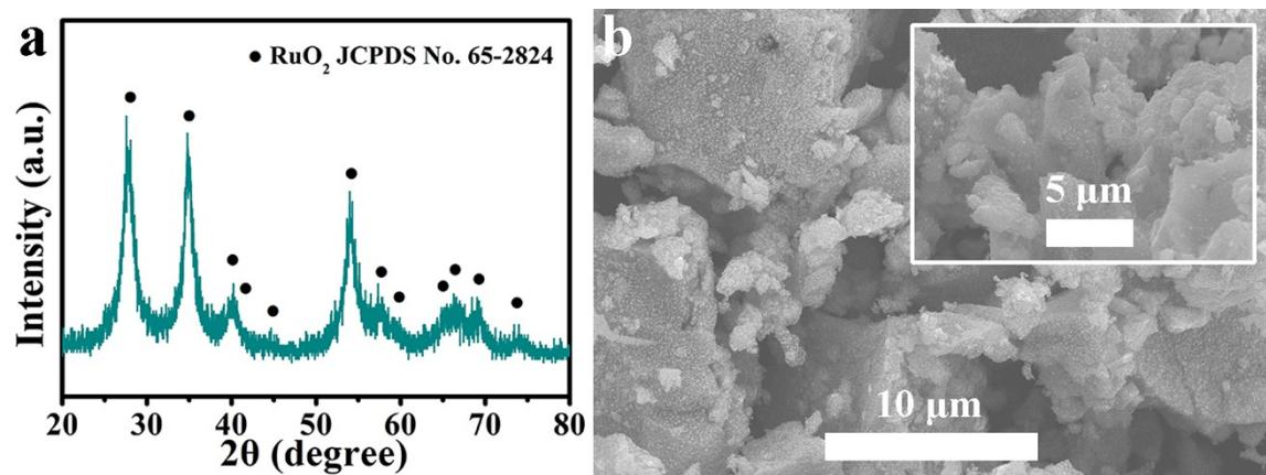
**Fig. S6.** (a) XRD pattern and (b) SEM images for RuO<sub>2</sub>.
