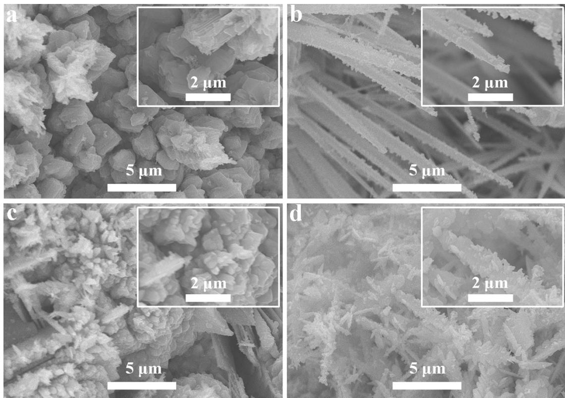
**Fig. S4.** SEM images for (a)  $\text{Cu}_3\text{Co}-\text{S}/\text{CF}$ , (b)  $\text{Cu}_2\text{Co}-\text{S}/\text{CF}$ , (c)  $\text{CuCo}-\text{S}/\text{CF}$ , and (d)  $\text{CuCo}_3-\text{S}/\text{CF}$ .
