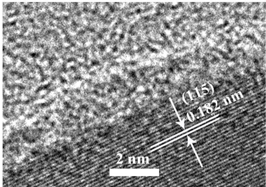
**Fig. S10.** HRTEM image for CuCo<sub>2</sub>S<sub>4</sub> after water oxidation electrolysis.
