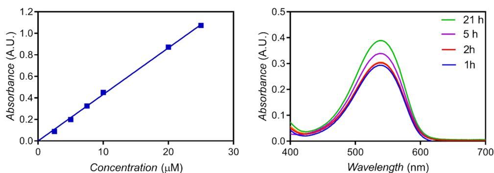
Fig. S6. Calibration curve (left) and a typical UV-Vis absorption spectrum of the azo dye (right) generated in the Griess assay at different concentrations of nitric oxide.
