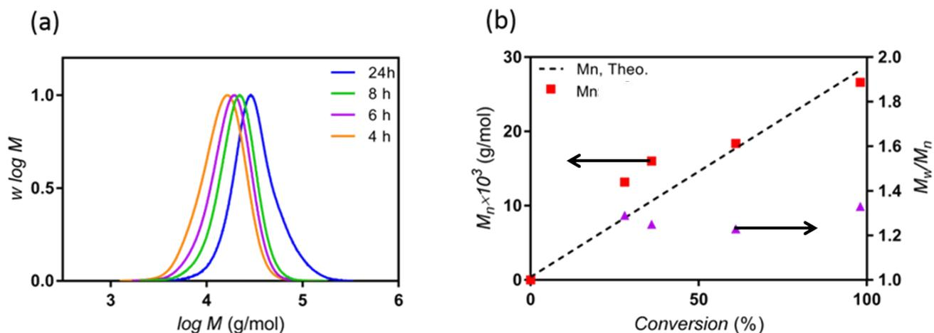
**Fig. S1.** Characterization data for PGMA homopolymers synthesized using PET-RAFT polymerization showing the evolution of: (A) molecular weight chromatograms and (B) number-average molecular weight and dispersity with monomer conversion. Polymerizations were performed under red light ( $\lambda_{\max} = 635$  nm,  $2.2$  mW/cm<sup>2</sup>) using [GMA]:[CDTPA]:[ZnTTP]= 200:1:0.02 at a total solids content of 50 wt% in DMSO
