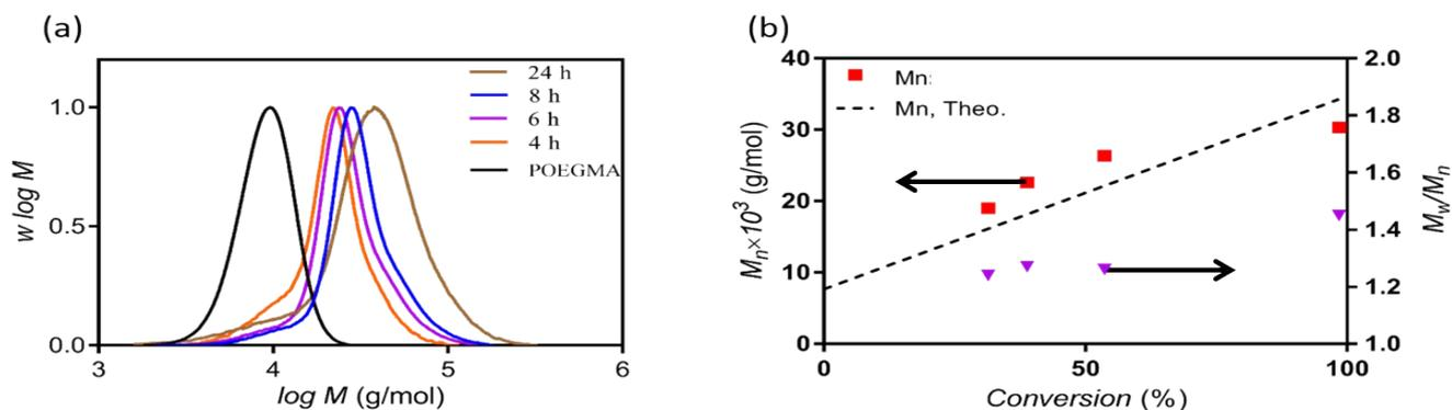
**Fig. S3.** Model kinetic study of the PET-RAFT dispersion polymerization of GMA in ethanol showing the evolution of (a) GPC molecular weight distribution and (b) number average molecular weight and dispersity with monomer conversion. Polymerization was performed using a [GMA]: [POEGMA]:[ZnTPP]= 200:1:0.002 under red light ( $\lambda_{\max} = 635$  nm, 2.2 mW/cm<sup>2</sup>) and at a total solids content of 10 wt% in ethanol.
