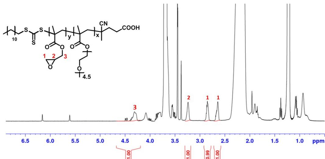
**Fig. S4.** Typical <sup>1</sup>H NMR spectra of crude POEGMA-*b*-PGMA copolymers synthesized by PET-RAFT dispersion polymerization.
