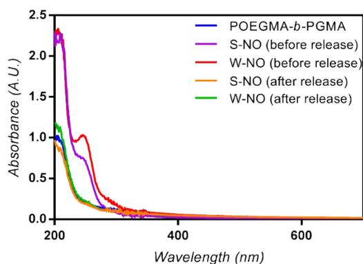
Fig. S5. UV-Vis absorption spectrum of POEGMA-*b*-PGMA (blue line), NONOate loaded NPs (S-NO/purple line and W-NO/red line) before release and corresponding NPs after two months incubation in PBS (S-NO/orange line and W-NO/green line) demonstrating successful NONOate conjugation. All spectra were acquired at a polymer concentration  $0.1 \text{ mg mL}^{-1}$  in water.
