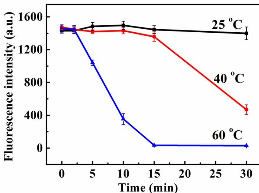
**Figure S5** Effect of temperature on the fluorescent stability of histone/DNA-templated CuNCs. The error bars represent the standard deviation of three independent measurements.
