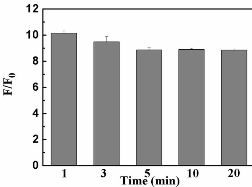
**Figure S3** Effect of histone-DNA interaction time on the fluorescence intensity of CuNCs. The error bars represent the standard deviation of three independent measurements.
