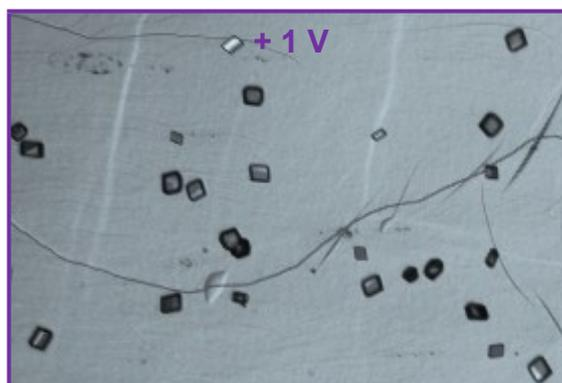
**Fig. S4:** Optical image of resulting crystal growth for an applied potential of + 1.00 V vs. SCE at the HOPG/Pt working electrode at a time of 5 hours
