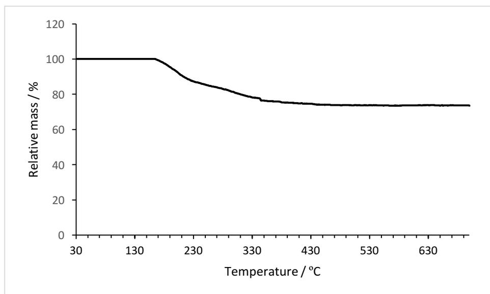
**Figure S32.** Thermogravimetric analysis (TGA) of **3-NP(L)**; organic ligand (assumed to correspond to mass loss) 26.4 wt% of **3-NP(L)**
