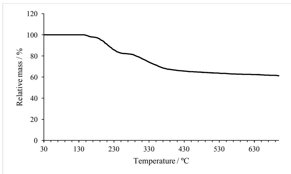
**Figure S33.** Thermogravimetric analysis (TGA) of **3-NP(D)**; organic ligand (assumed to correspond to mass loss) = 38.7 wt% of 3-NP(D)
