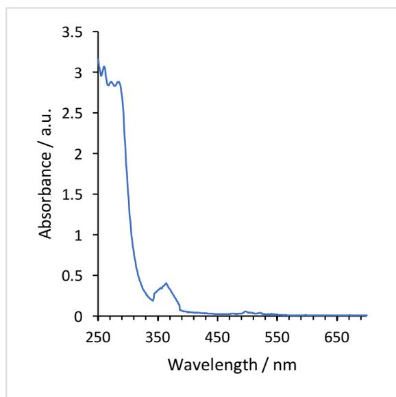
**Figure S19.** UV-Vis absorption spectrum of **1(D)** in DCM
