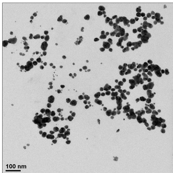
**Figure S29.** TEM image of 3-NP(L) following de-protection with hydrochloric acid
