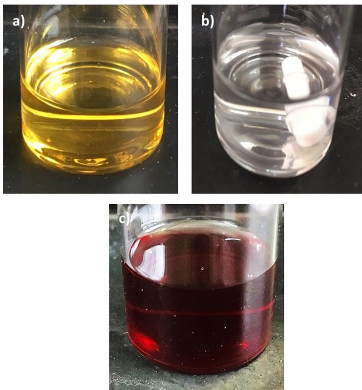
**Figure S16.** Photographs of **3-NP(D)** synthesis: a) **2(D)** in THF before addition of  ${}^t\text{BuNH}_2\cdot\text{BH}_3$ , b) following reaction with  ${}^t\text{BuNH}_2\cdot\text{BH}_3$  and being stirred for 24 hrs at room temperature (25 °C), c) removal of solvent and **3-NP(D)** re-dispersed in DCM.
