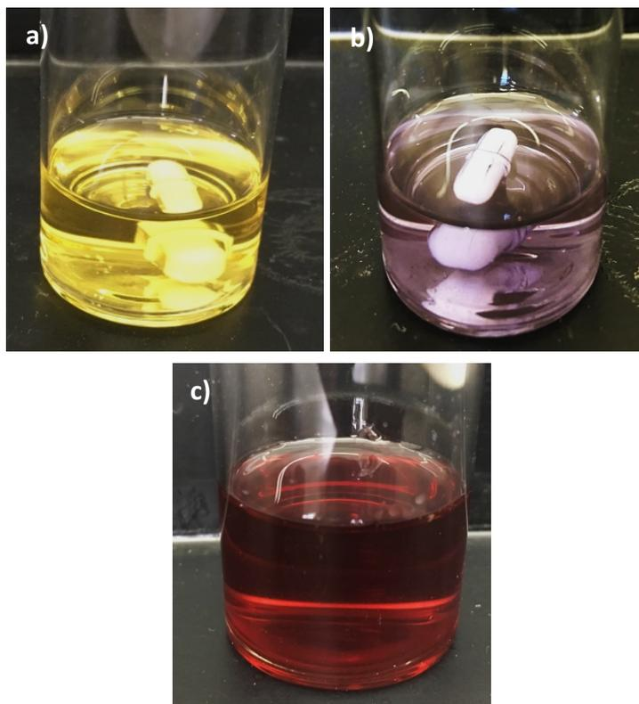
**Figure S15.** Photographs of **3-NP(L)** synthesis: a) **2(L)** in THF before addition of  $t\text{BuNH}_2\cdot\text{BH}_3$ , b) following reaction with  $t\text{BuNH}_2\cdot\text{BH}_3$  and being stirred for 24 hrs at room temperature (25 °C), c) removal of solvent and **3-NP(L)** re-dispersed in DCM.
