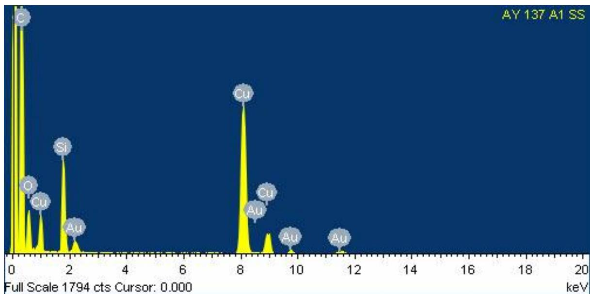
**Figure S28.** EDX analysis of **3-NP(L)**; copper and silicon peaks have been determined to originate from the TEM grid not the sample.
