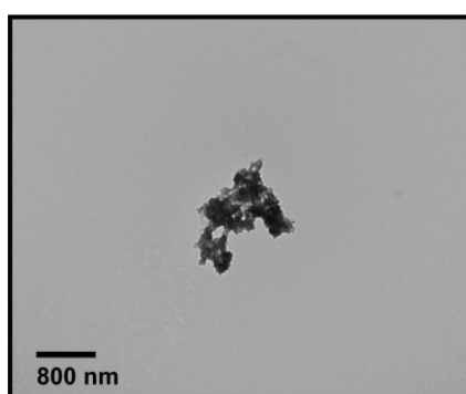
Figure S15. TEM images of 500 μM PO 18 C in 10 mM CaCl 2 after 15 h. Few aggregates were observed.
