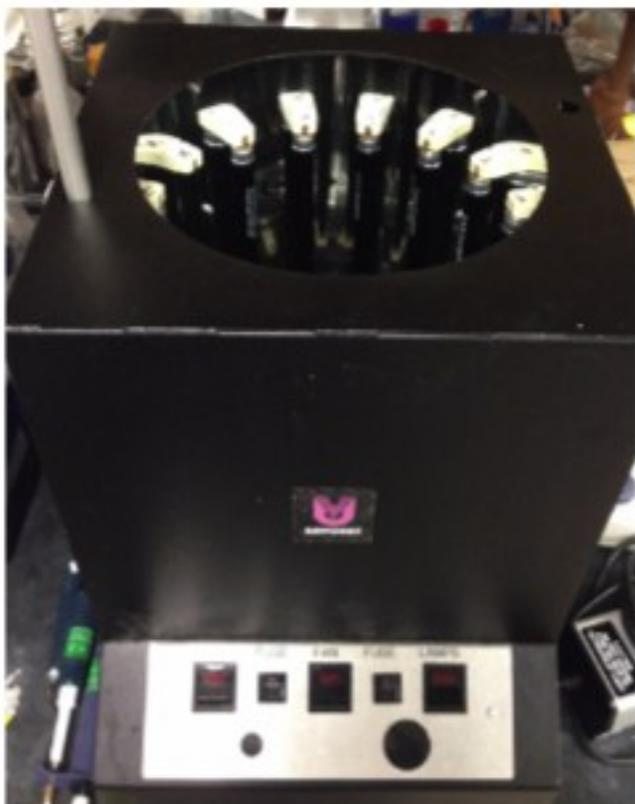
Figure S2. The Rayonet RPR-200 Photochemical Reactor has a maximum of 16 lamps surrounding a central reaction chamber. The lamps used in this study were mercury emission lamps, with primary emission at 254 nm. This reactor is the same system as used by Ritson and Sutherland<sup>1</sup>.
