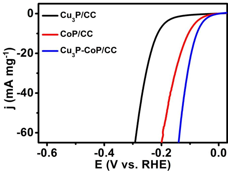
**Fig. S4.** Mass-normalized polarization curves for Cu<sub>3</sub>P/CC, CoP/CC and Cu<sub>3</sub>P-CoP/CC in 0.5 M H<sub>2</sub>SO<sub>4</sub>.
