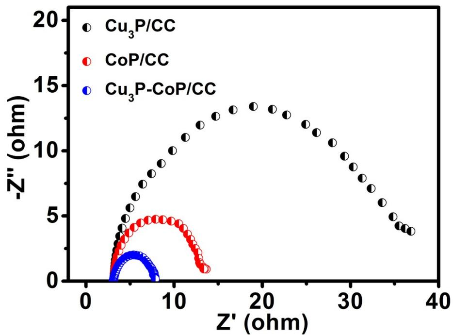
Fig. S5. Nyquist plots of Cu<sub>3</sub>P/CC, CoP/CC and Cu<sub>3</sub>P-CoP/CC recorded in 0.5 M H<sub>2</sub>SO<sub>4</sub>.
