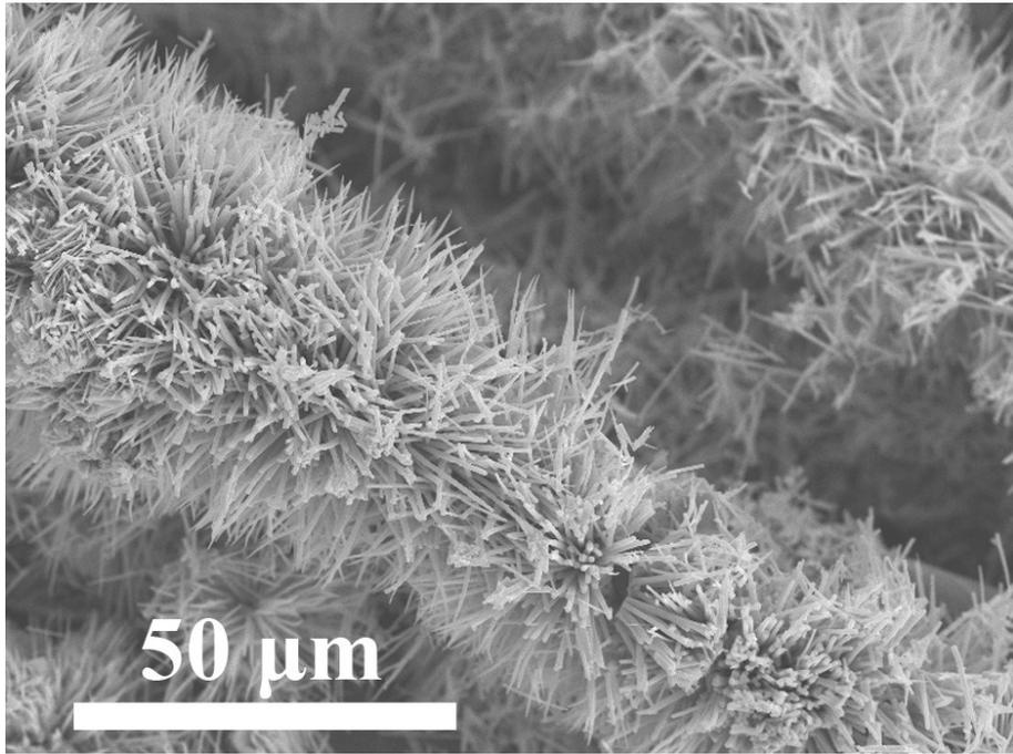
**Fig. S2.** SEM image of  $\text{Cu}_3\text{P-CoP/CC}$  after 500 cyclic voltammetry cycles.
