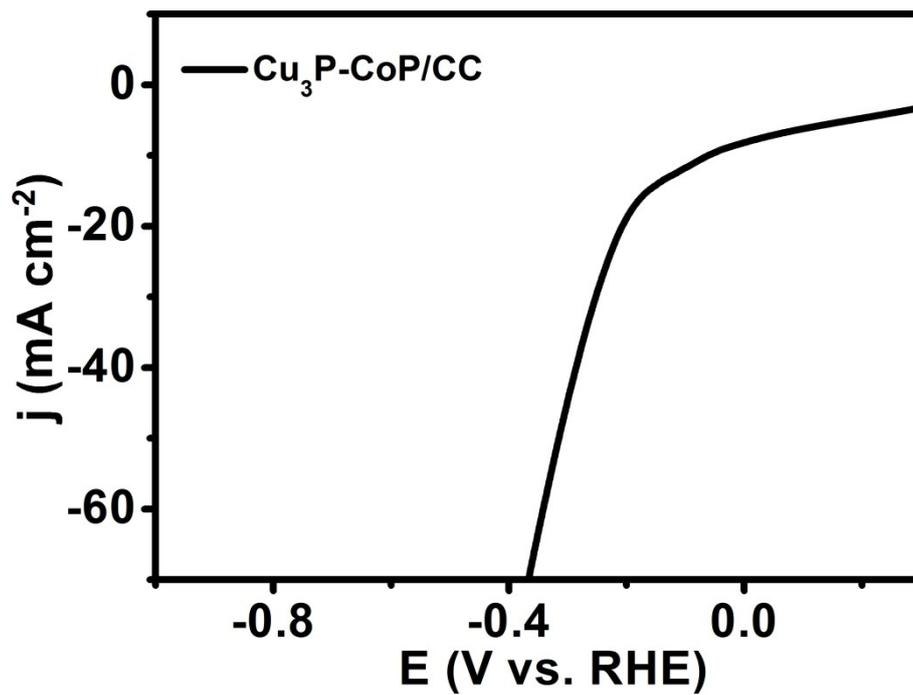
**Fig. S1.** LSV curves for Cu<sub>3</sub>P-CoP/CC with a scan rate of 5 mV s<sup>-1</sup> in 1.0 M KOH.
