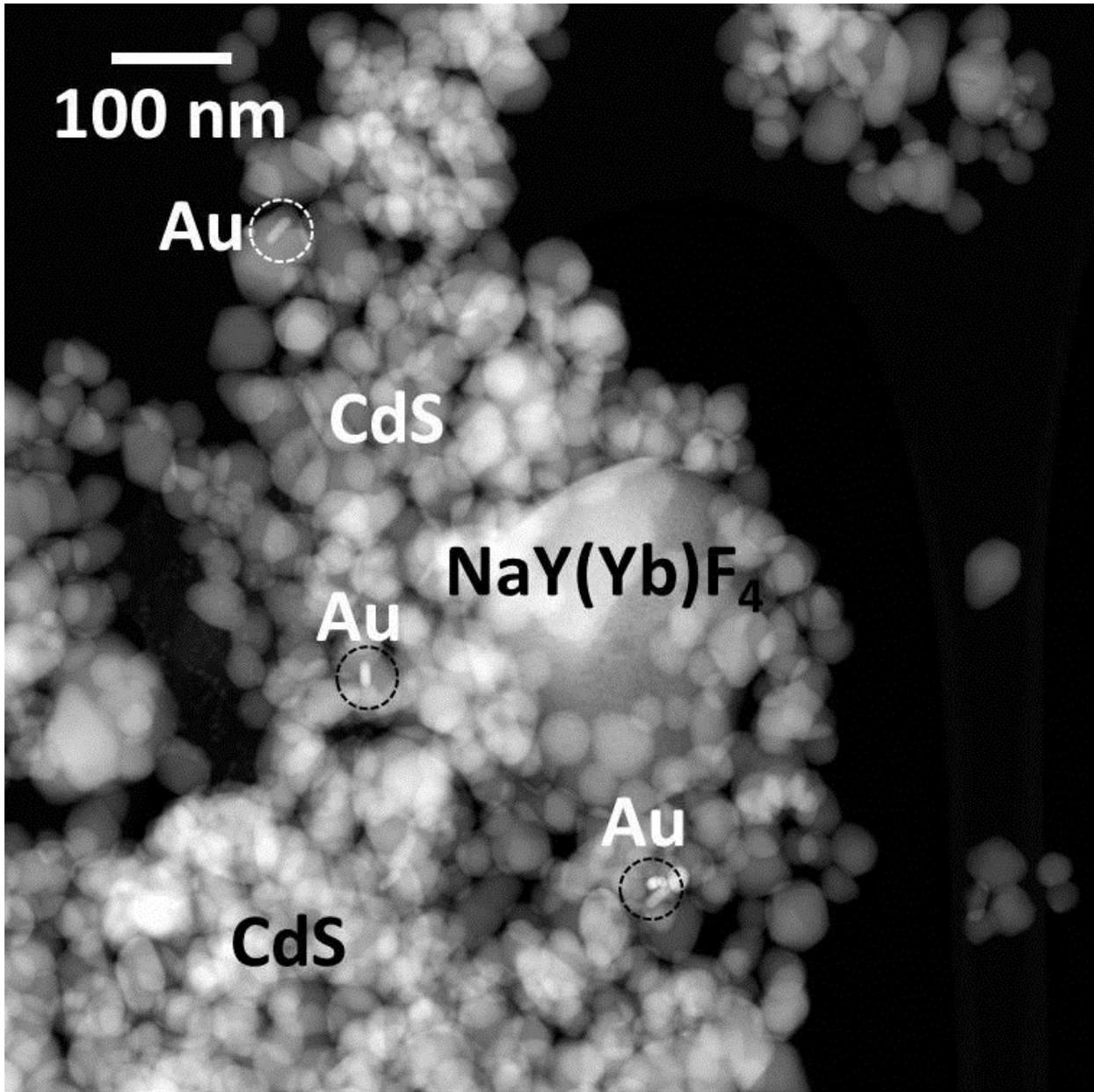
Figure SF3 B. STEM-HAADF of  $\text{NaYF}_4(\text{Yb})\text{:Tm}$
