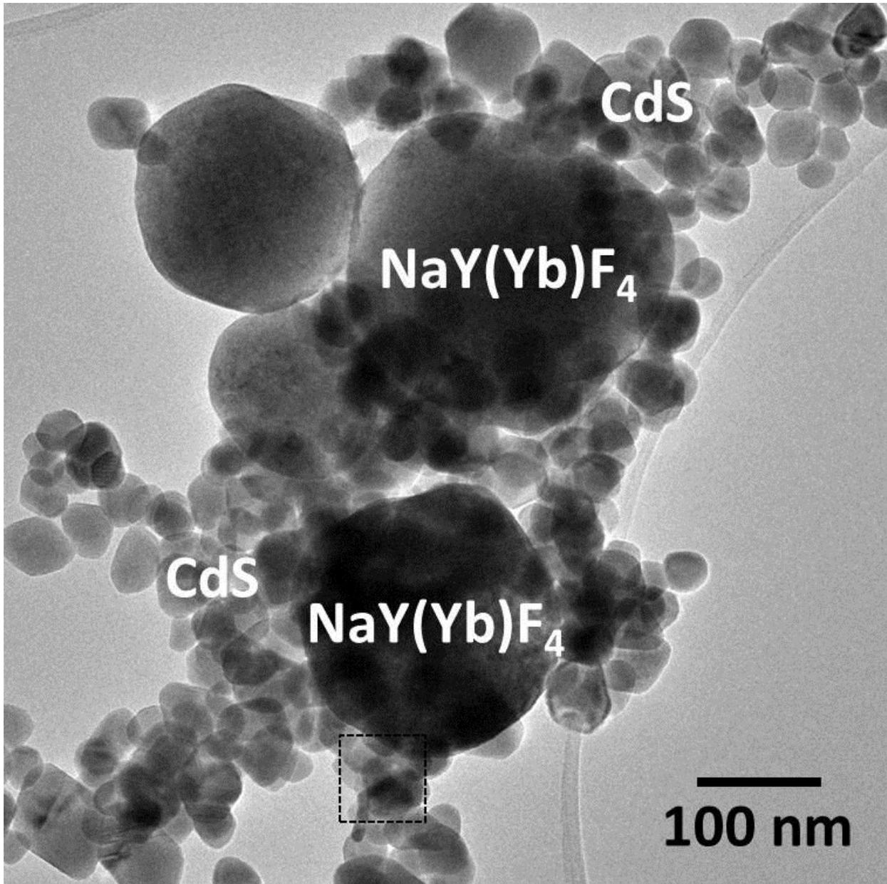
Figure SF3 C. HRTEM of  $\text{NaYF}_4(\text{Yb})\text{:Tm}$
