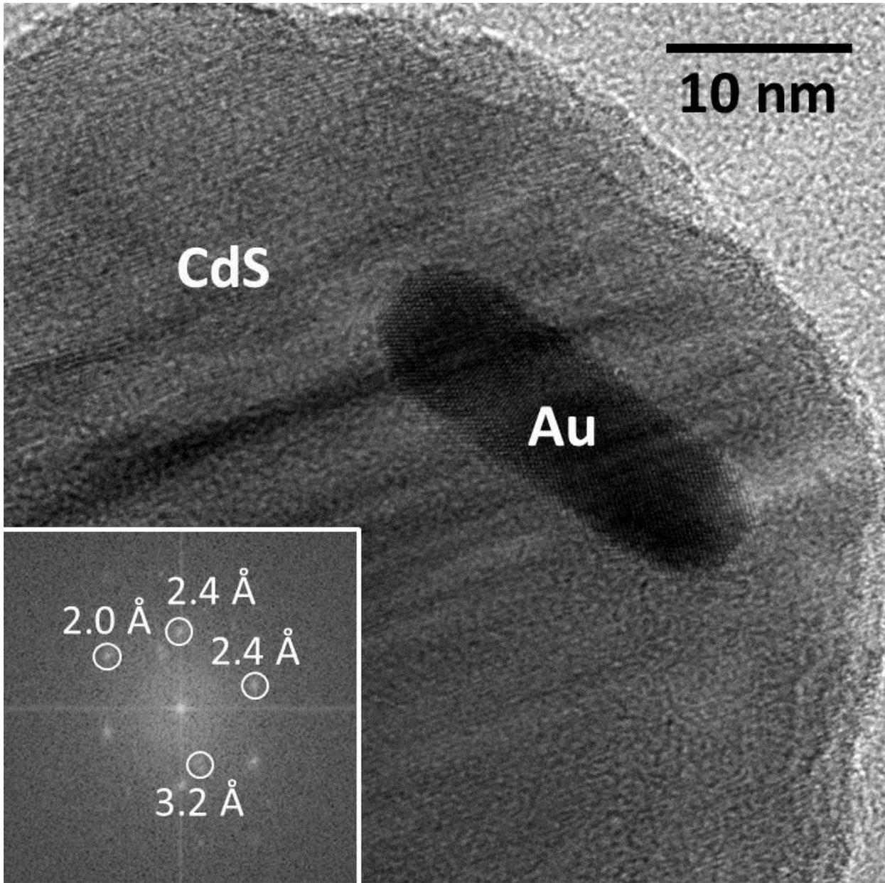
Figure SF3 D. HRTEM and FFT of Au/CdS nanoparticles
