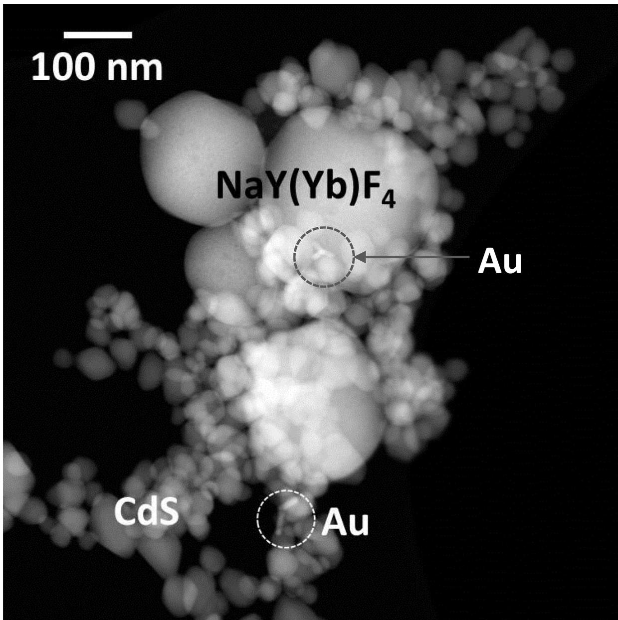
Figure SF3 A. STEM-HAADF of  $\text{NaY}_4(\text{Yb})\text{:Tm}$
