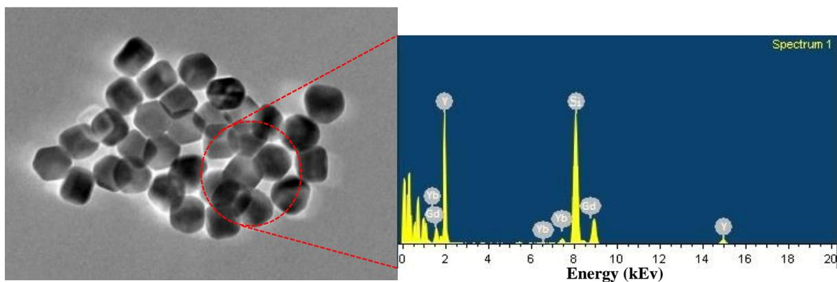
Fig. S2. Energy-dispersive X-ray analysis (EDX) patterns of  $\beta$ - NaYF<sub>4</sub>:Yb,Gd NPs showing elemental composition.
