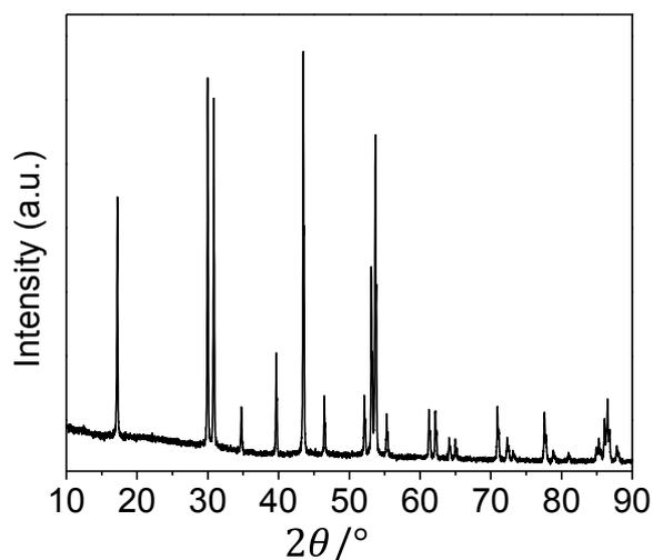
Fig. S1. Powder XRD patterns of as-prepared  $\beta$ -NaYF<sub>4</sub>:Yb,Gd NPs. The overall peak profile demonstrates an excellent crystallinity of the UCNPs.
