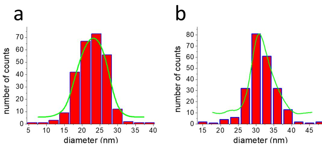
Fig. S3. The size distribution of the UC-NPs obtained from TEM images for NaYF<sub>4</sub>:Yb,Gd NPs (a) and LTP- conjugated  $\beta$ -NaYF<sub>4</sub>:Yb,Gd NPs (b). Image J software was employed for quantitative analysis. Data were obtained by measuring more than 200 UC-NPs for both the case.
